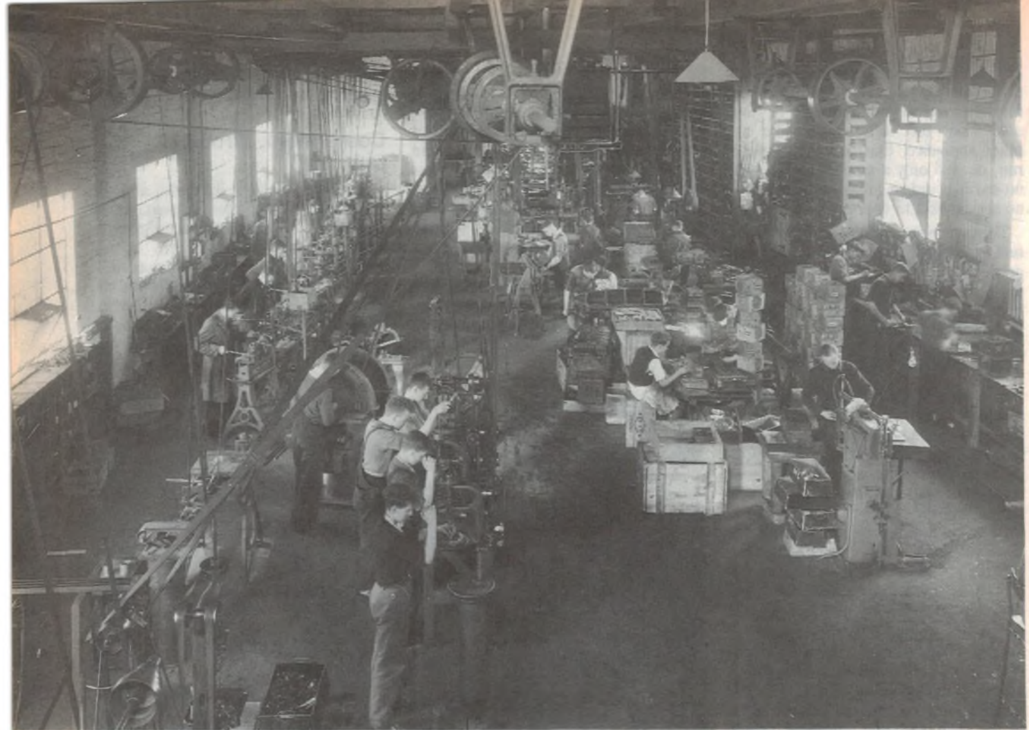
An overall view inside the Melbourne factory of Astor, again in the 1930's. Note the overhead drive shafts and belting, with drilling machines in the centre foreground and lathes at upper left.
