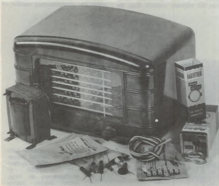
In the 50 years from about 1925 to 1975, countless radio receivers were built by hobbyists. This kitset from 1945 made use of a bakelite moulded cabinet and other parts left over from factory production runs.
