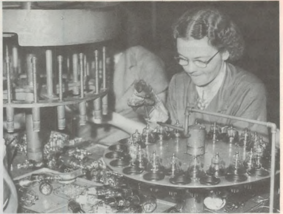
Fitting grid caps to the tops of valves in the Amalgamated Wireless Valve Company at Ashfield, Sydney in the mid 1930's.
