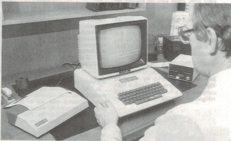
The Apple II, another extremely successful 'first generation' personal computer. By late 1981, combined Apple and TRS-80 sales were over 1 million units.
