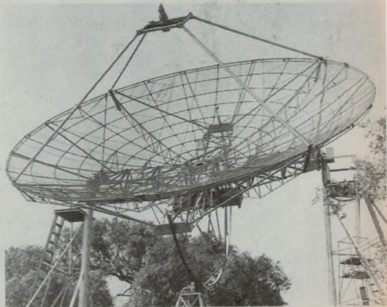
Fig.8 (below): 36-ft diameter transit instrument at Potts Hill, used mainly for H-line work.
