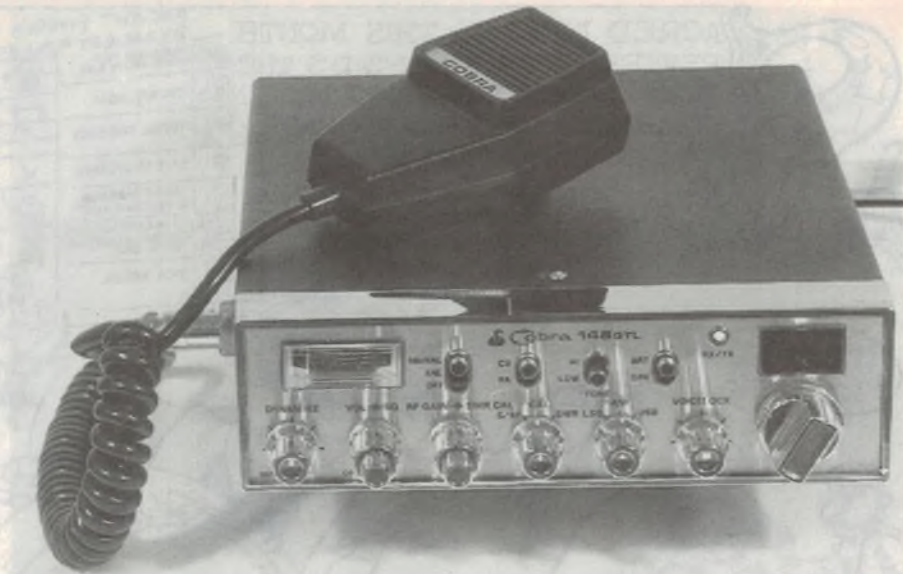
The Cobra 148GTL, a fancy late-model CB transceiver. It features 40-channel operation, AM/LSB/USB, noise blanking and ir:built SWR metering.
