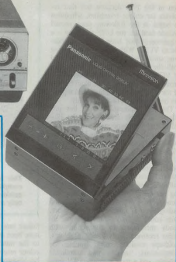
This current-model 'Minivision' personal portable colour TV receiver from Panasonic shows how far television has come since the mid 1950's. It uses a colour LCD screen and features digital tuning over both VHF and UHF channels.
