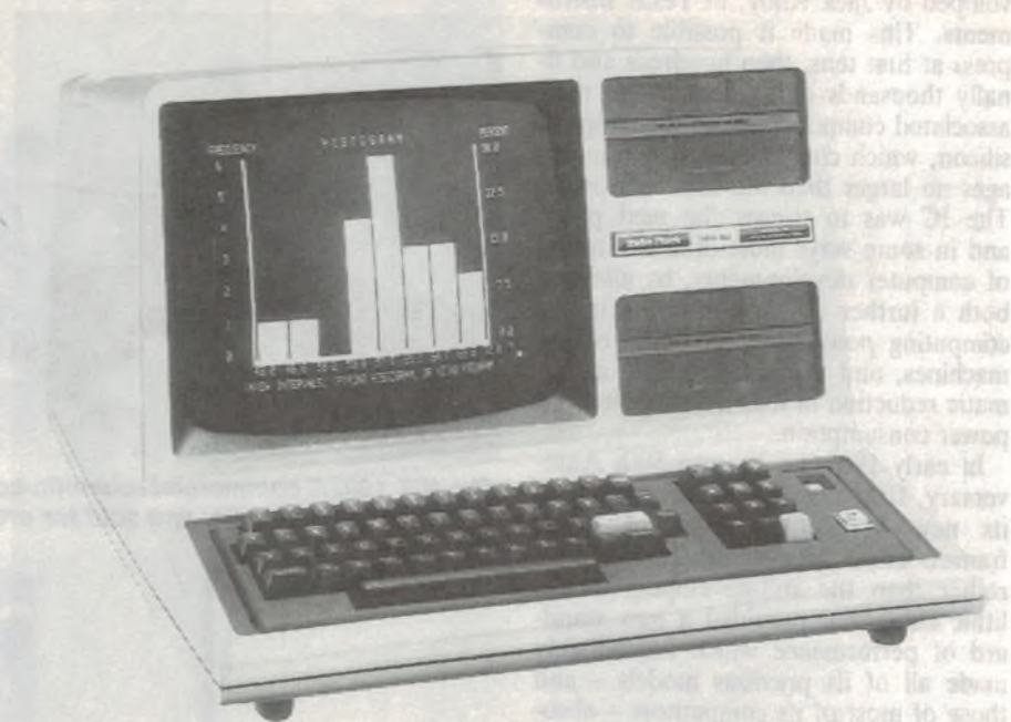
Above: Not the original Tandy TRS-80 model 1 personal computer, but its successor the model 3. The earlier unit had the computer, monitor and floppy disk drives as separate units.
