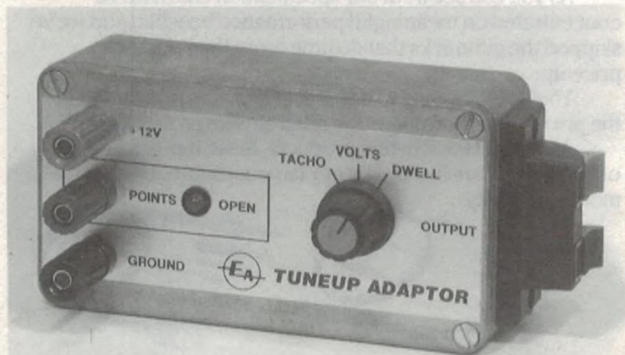
The unit may be permanently installed into the engine bay and hard-wired to the ignition system, or used as a portable test instrument with flying connector leads.
