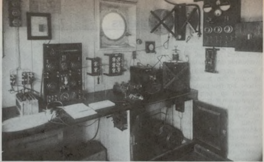
Spark transmitters were widely used in Australian merchant ships. Pictured above is the radio cabin of S.S. 'Burwah', fitted with an AWA ½kW quenched spark set.
