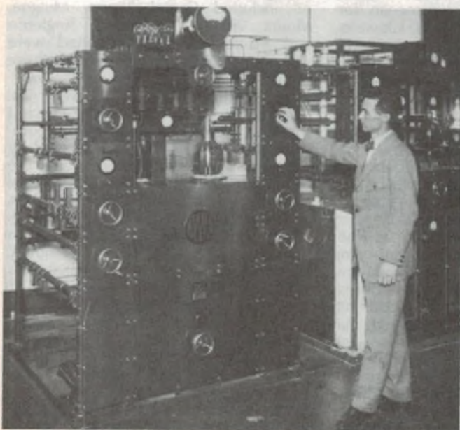
AWA engineer Sydney Newman with the company's experimental 20kW shortwave transmitter, Pennant Hills, 1928.
