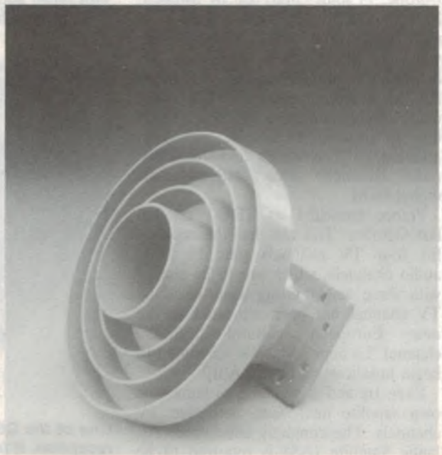
A feed horn for C-band reception, normally bolted to the input flange of the LNA or LNC, at the focus of the dish antenna. It includes a circular to rectangular waveguide transition. The annular rings are RF chokes, forming a low-loss reflector. (Courtesy Dick Smith Electronics)
