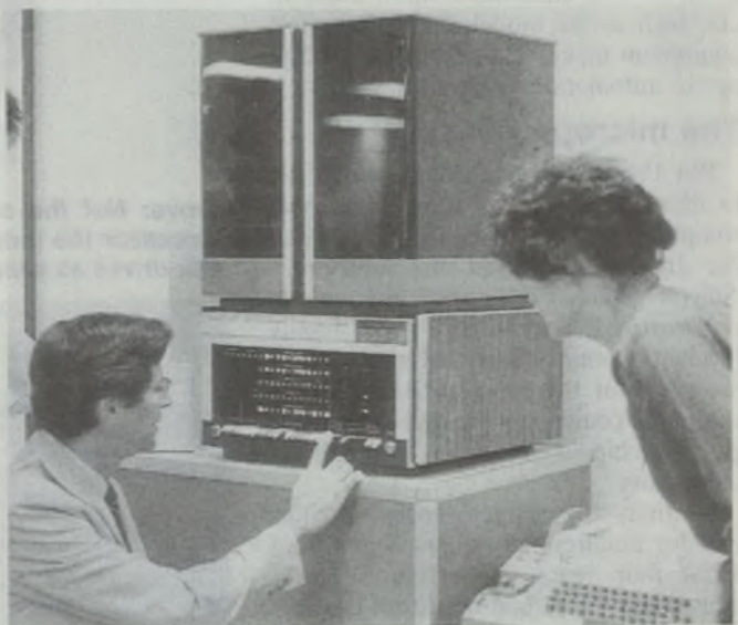
The ICT 1902A commercial/scientific computer, released in early 1968. It used TTL integrated circuits, and sold for around $200,000.
