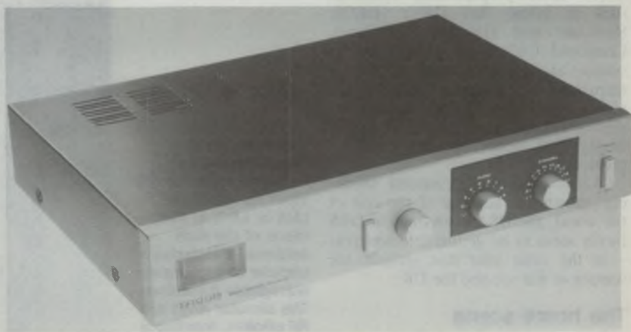
One of the DBS receivers available from Dick Smith Electronics, for Intelsat V reception. It tunes from 950 to 1450MHz, producing video and audio.
