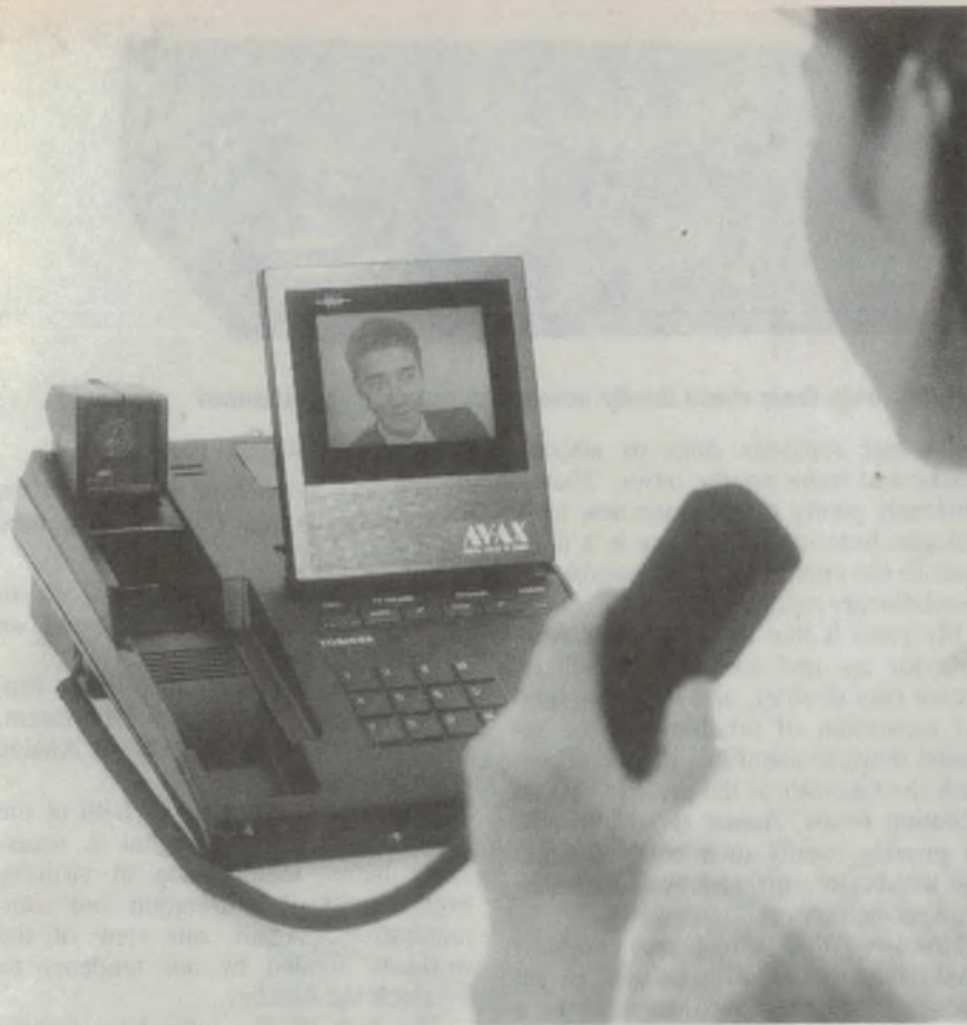
Toshiba's new prototype colour videophone, which uses two 64kbit ISDN channels to provide moving images. But do users really want video phones?
