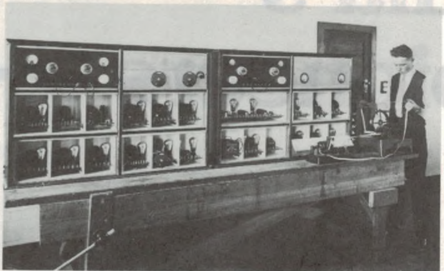
This 'special 16 valve supersonic heterodyne receiver' was used at AWA's La Perouse station for reception of high speed morse from Melbourne in the '20s.
