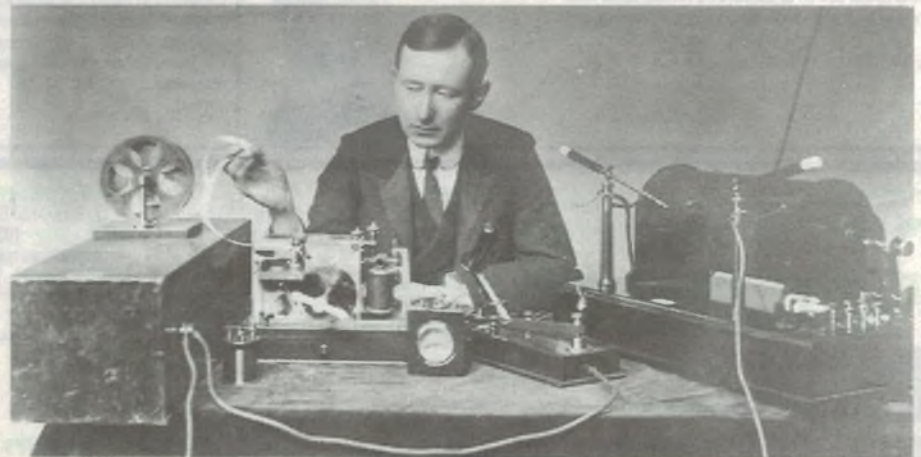
Wireless pioneer Guglielmo Marconi pictured in 1911 with some of his equipment. Note the induction coil at right.
