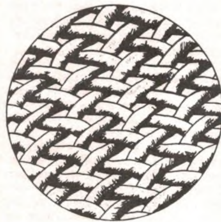
Fig.1: The 'glass' reinforcing in an epoxy-fibreglass PCB laminate is generally a plain weave of 'E' glass fibre.
