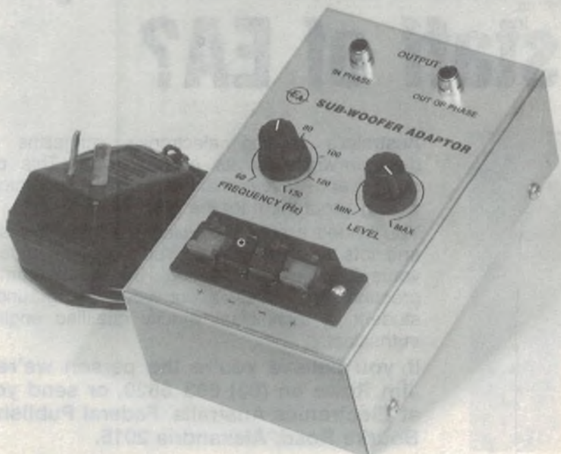
The completed prototype of the adaptor. Independently powered by a low-cost plug-pack, it can easily be connected to almost any hi-fi system.
