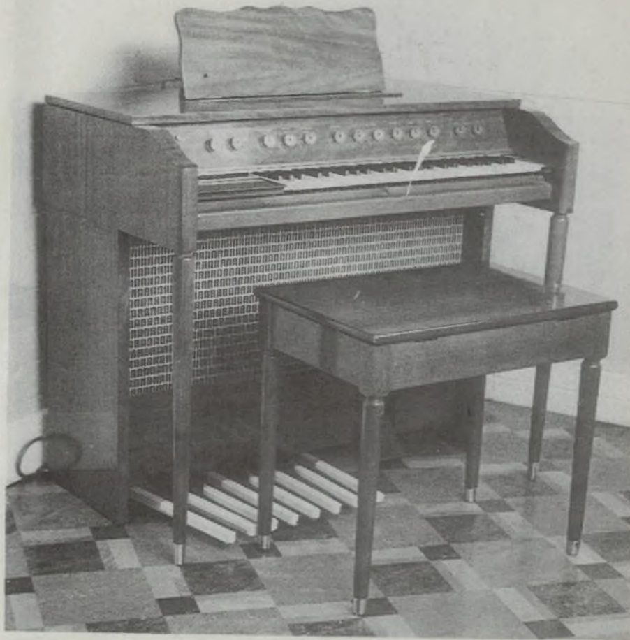
The Stromberg-Playmaster kit organ, described in this magazine during 1961-2. Small electronic organs like this took over from reed instruments, showing the way for bigger and better spinet models which are now routine in homes and small churches.
