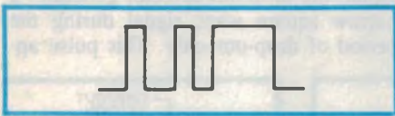
Fig.5: When it reaches the FM demodulator at point P, the signal is a rectangular wave.
