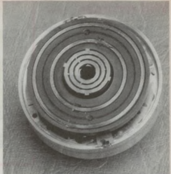
Underneath the upper section of a head drum assembly from a Philips VCR, showing the rotating halves of the rotary transformers for each head. The windings are the lighter rings in the central (annular) grooves.
