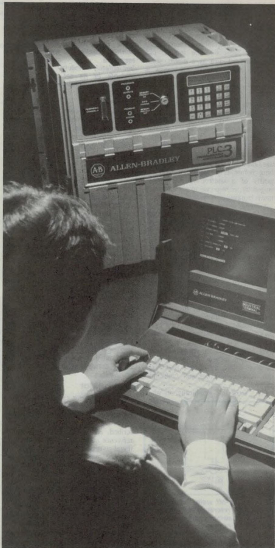
Programming a PLC unit. Photo courtesy of Allen-Bradley.
