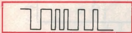
Fig.3: The luminance signal at point N is in the form of an FM carrier centred on 4.3MHz, and deviating by +/-500kHz.
