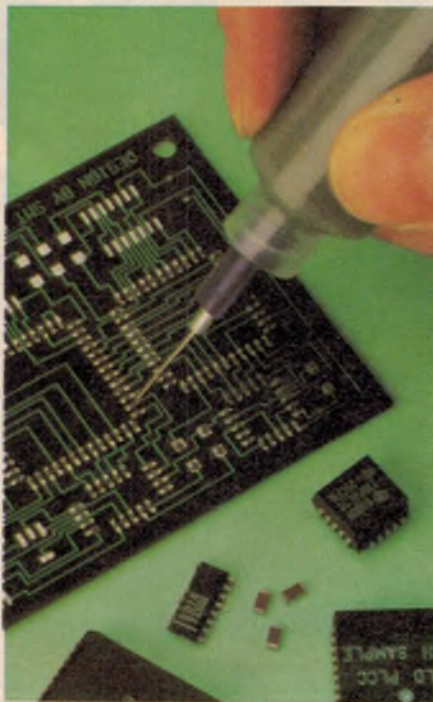
Reliable solder connections with no bridging between tracks depends upon precise application of solder paste.
