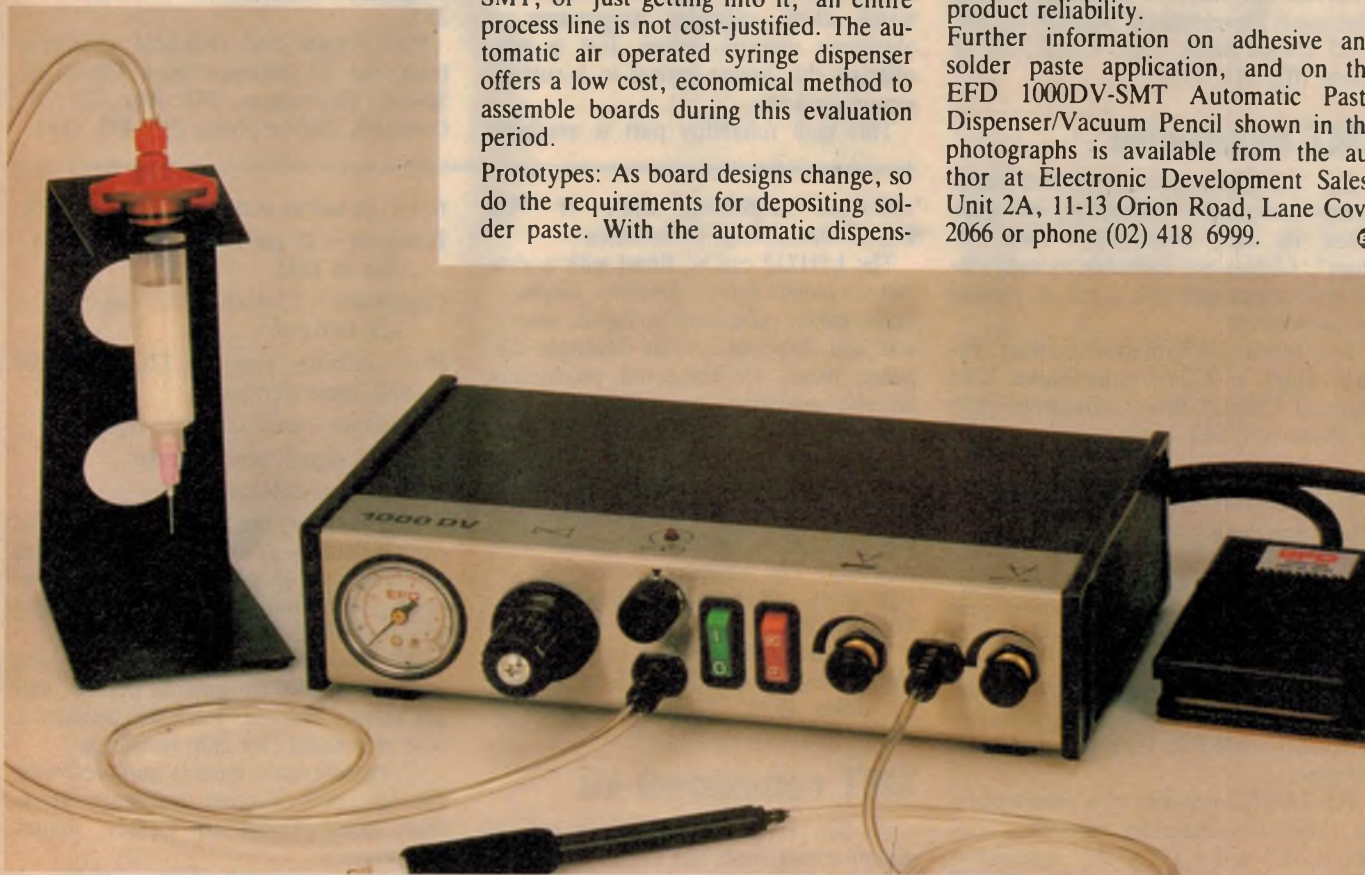
The EFD model 1000DV-SMT surface mount workstation allows precise and consistent air-pulse application of either adhesive or solder paste, together with precise handling and placement of components via a vacuum pickup pencil with multiple tips.
