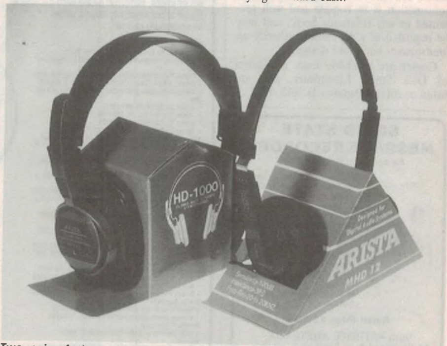
Two pair of stereo headphones from Arista. The HD-1000 pair at left have 'circum-aural' muffs, while the MHD-12 pair at right have foam pads.
