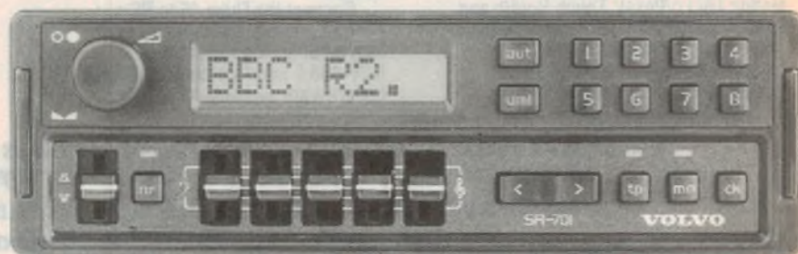
The Volvo SR-701, first RDS radio to become available in the UK. It is built in Japan by Mitsubishi.
