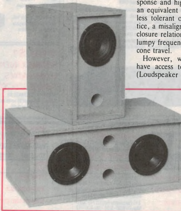
The prototype enclosures in unfinished particle board. Both versions offer a smooth response down to about 35Hz.
