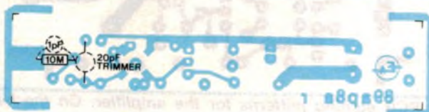
Fig.7(b): Suggested probe head mods to add the input divider permanently.
