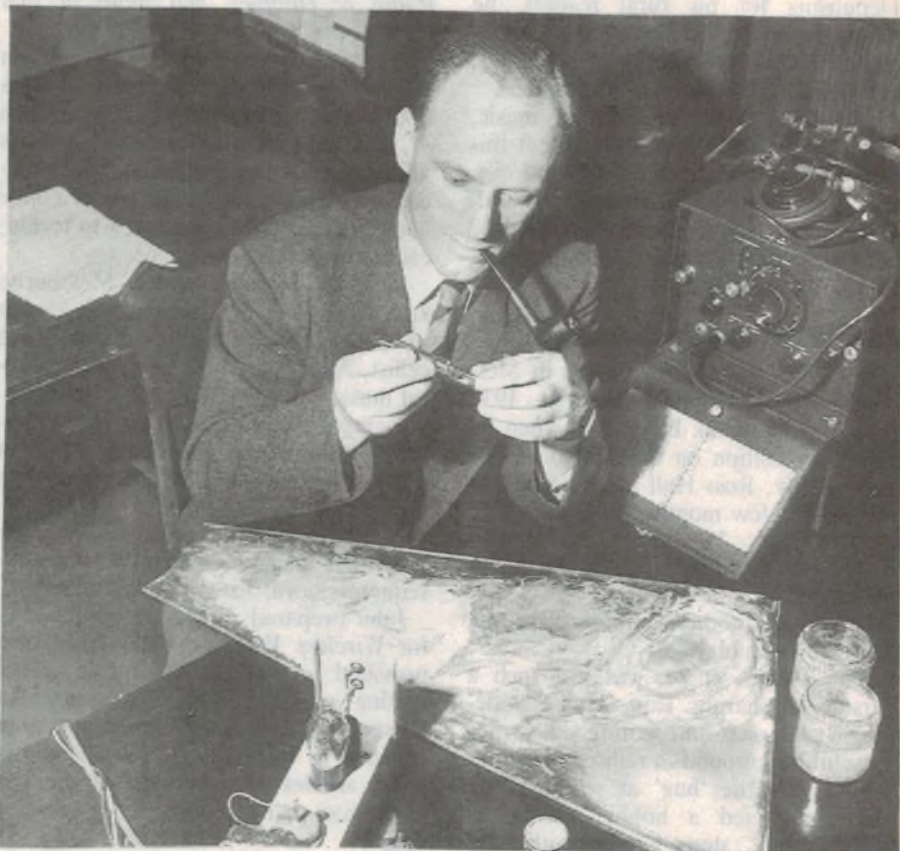
Complete with pipe and micrometer, John is pictured here with his crystal-grinding paraphernalia spread out on the table: frequency meter (top right), a slab of rigid very flat glass and (foreground) his test oscillator. In those days, crystals were large enough to handle – gingerly! (Courtesy Dr Alice Moyle)
