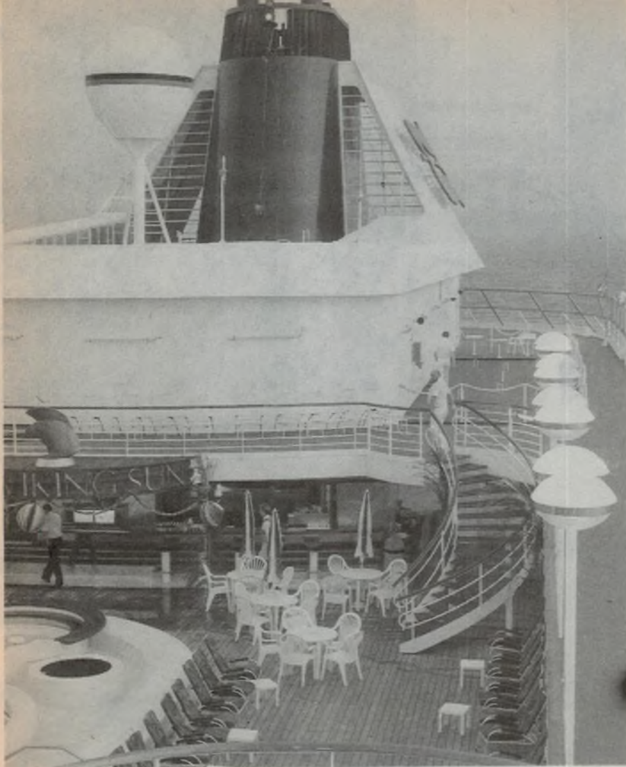
Well above the Sun's entertainment and pool deck and near the stern funnel is a radome-enclosed Intelsat dish, one of three satellite dishes on the elegant vessel.
