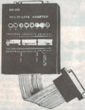
A complete in-line tester/adaptor which makes complex and time consuming Serial connections a breeze. Comes with 25 pin male connector at one end and 25 pin female connector at the other. With jumper pads and wires, as well as 24 in-line switches, for quick selection for any RS-232 configuration. The tester itself has 8 bi-colour LED's which monitor the lines and tell you at a glance when you've got it right.
