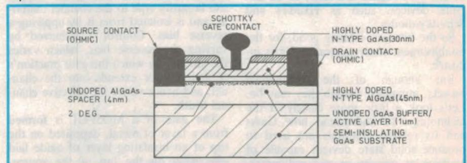
**Fig.2: Construction of a standard high electron mobility transistor, or HEMT, which conducts via a two-dimensional electron gas or '2 DEG'.**
