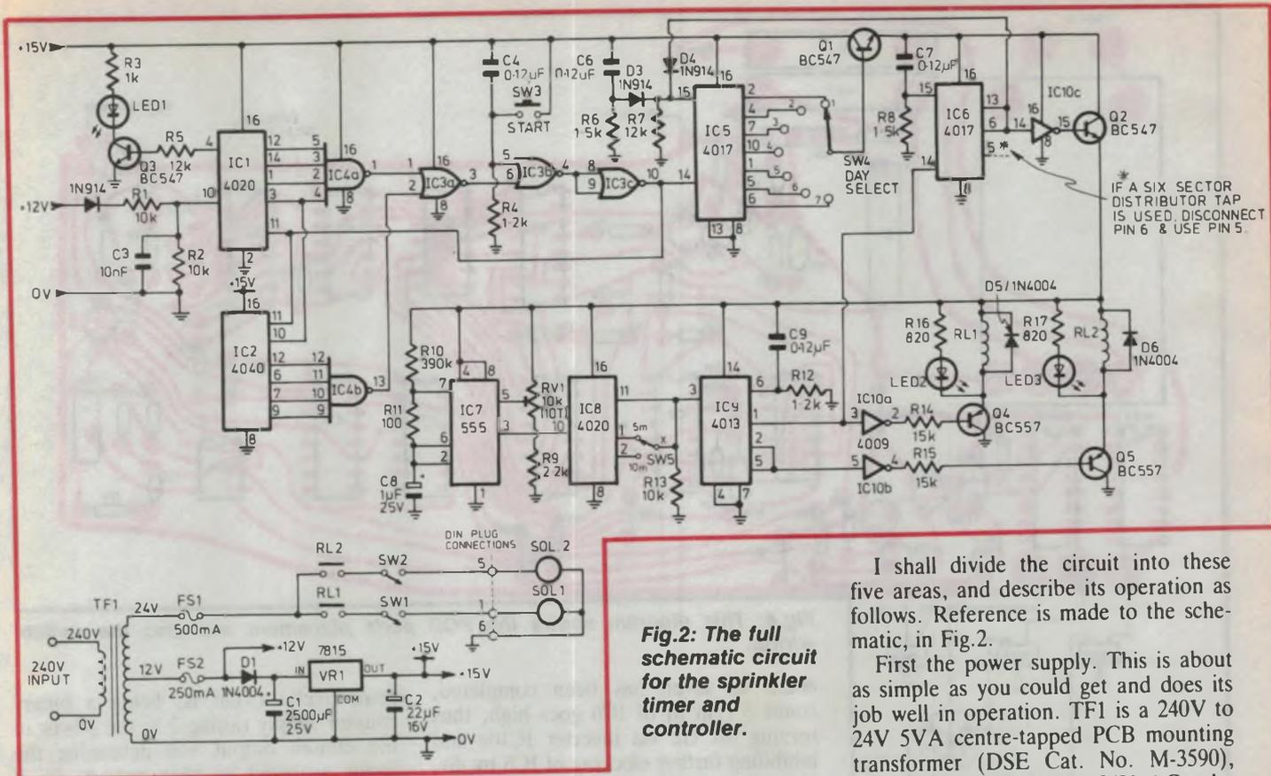
**Fig. 2: The full schematic circuit for the sprinkler timer and controller.**
