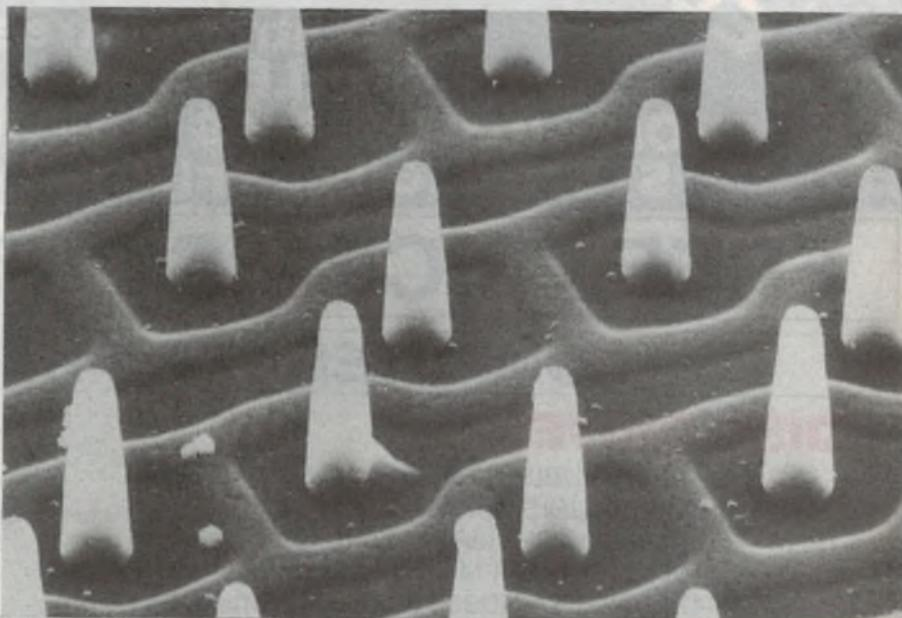
*No, it's not a bunch of candle flames, but an inverted scanning electron microscope shot of the trench capacitors in Siemens' new 4MB DRAM chip.*
