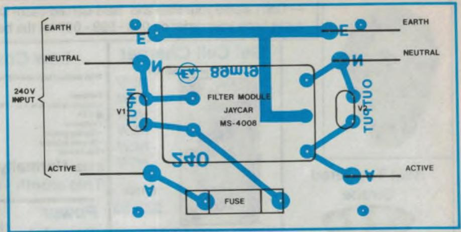
The PCB layout for the Jaycar mains filter unit. The fuse holder should ideally be protected from accidental contact with some form of insulated covering.
