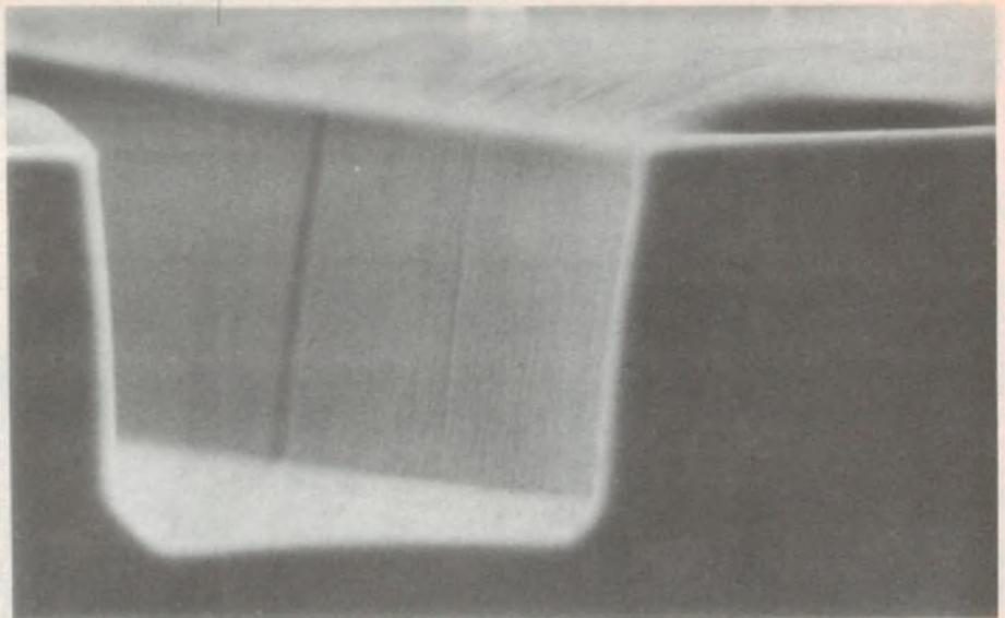
**Cross-section of one of the sub-micron trenches etched into a GaAs wafer by the Group, using reactive ion etching. Note the steep sides.**
