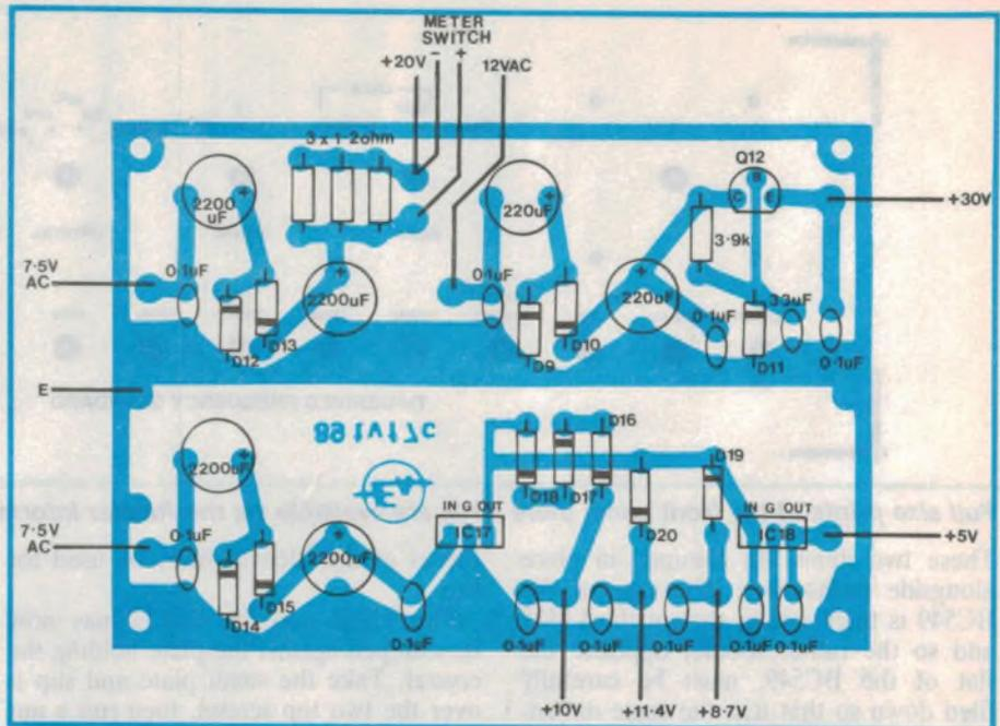
Above shows the component location and wiring for the power supply board, with the board etching pattern itself shown below actual size.
