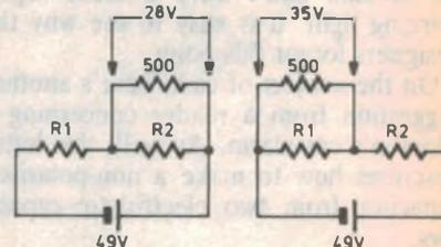
The question is, given the data shown on the two circuits in Fig.3, deduce the values of R1 and R2. Have fun – it's easy enough when you know how, but can lead you into some dead ends on the way.
