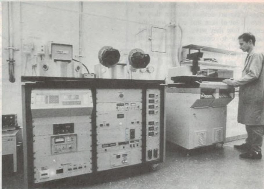
The Group's RIE/PECVD plasma etching and deposition system, left and centre, with its wafer dicing saw in use at right.
