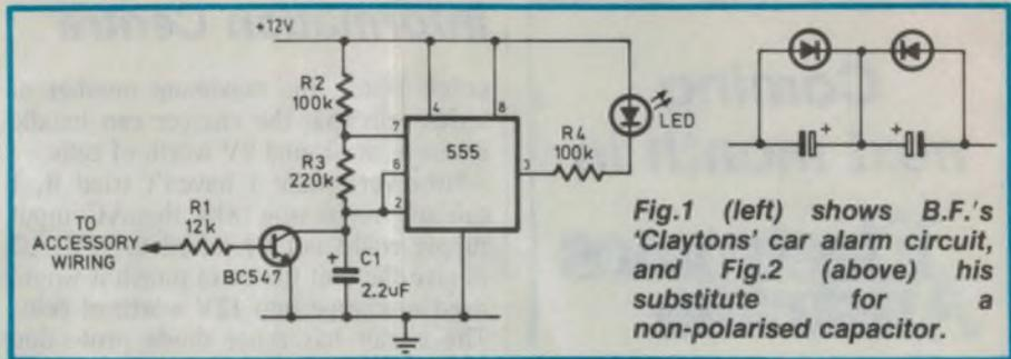
Fig.1 (left) shows B.F.'s 'Clayton's' car alarm circuit, and Fig.2 (above) his substitute for a non-polarised capacitor.
