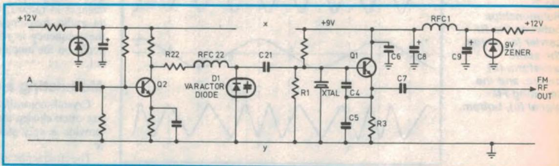
lator frequency. We have frequency-modulated the crystal oscillator by an audio voltage.
