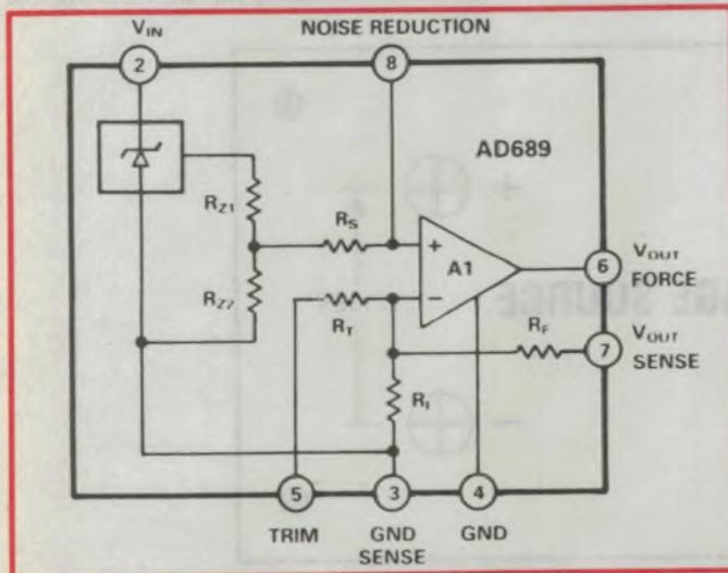
**Fig.1: A simplified internal circuit for the AD689.**
