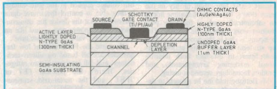
**Fig.1: The basic construction of a GaAs MESFET device. Its operation is explained in the text.**
