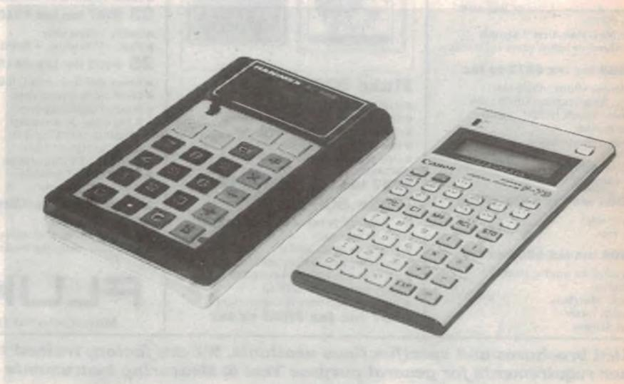
**Twelve years of pocket calculator development! The 1975 model Hanimex BC999B on the left has only 8 maths functions. It measures 135 x 83 x 24mm. By comparison, the 1987 Canon F-73 has more than 48 maths and scientific functions, and measures only 135 x 70 x 9mm.**
