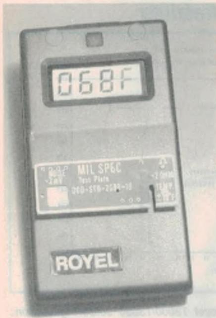
Royal's test unit, which can be used to monitor whether an iron continues to meet temperature control and leakage specs.
