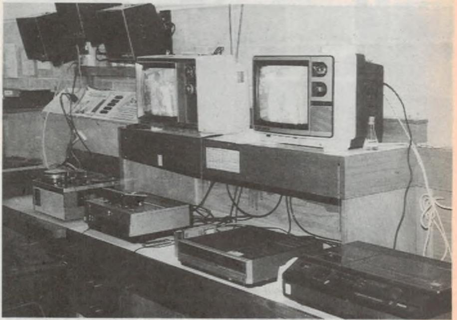
**A typical college AV workroom. The equipment in this system includes two VHS recorders, a Philips NV1500 and an old Sony AV 3670-CE monochrome machine. All units are still in use, although the Philips and the Sony are only used for playback these days.**
