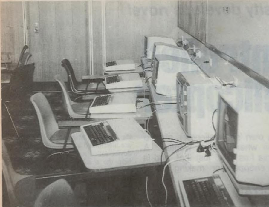
*The BBC model B microcomputer was designed specially for educational use and this picture shows a typical college computer studies room. Networking was part of the Model B's initial design specification, and since then thousands of LAN specialists have cut their teeth on BBC's and 'Econet'.*
