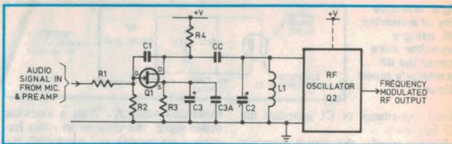
Fig.4: Reactance modulation using a JFET transistor (Q1).
