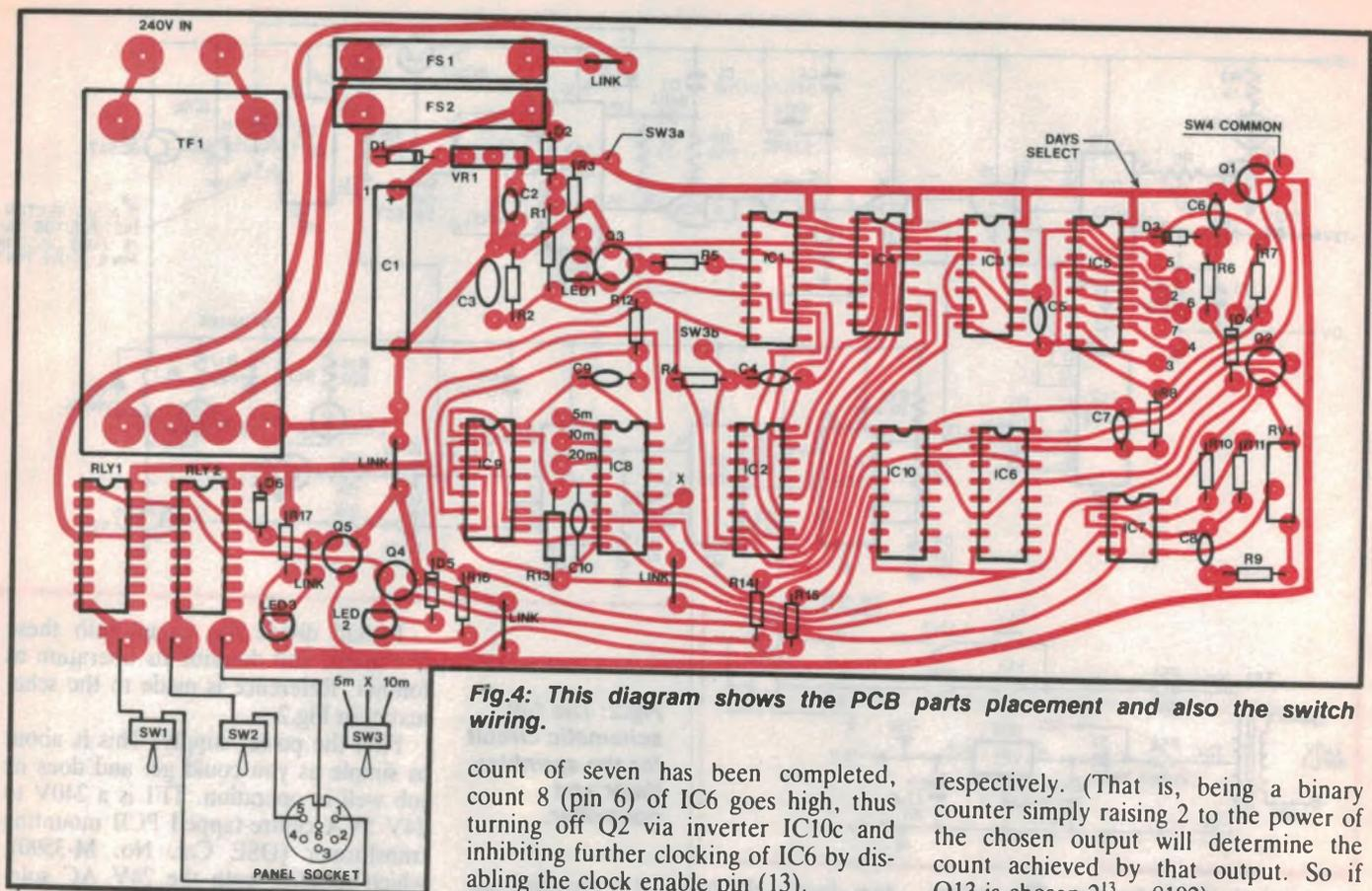
**Fig.4:** This diagram shows the PCB parts placement and also the switch wiring.
