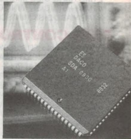
static CMOS RAMs from 1K byte to several megabytes. The SDA 8800 HSDA controller is already intended for operation with future SRAMS. Up to 32 caches of 4Mbytes each can be connected to one SDA 8020 HSDA shift register.
