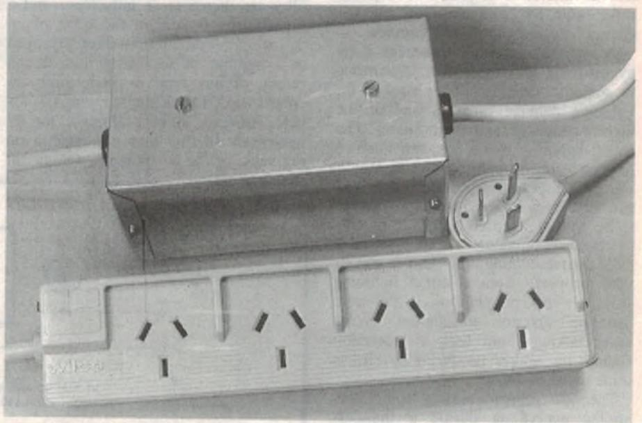
**Fig.5:** By inserting a mains filter in the lead of a multi-outlet board, protection can be provided for a number of appliances. The total load from the board will be limited to around 3A, which should be adequate for a TV, video and hi-fi combination.
