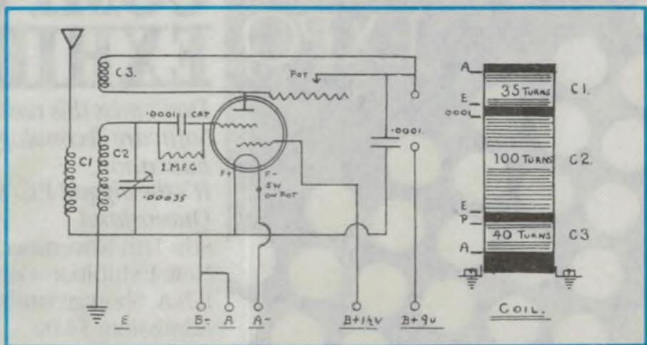
**The circuit of the Improved Hikers. The 'pot' was an inexpensive regeneration control and on/off switch. The use of regeneration gave sensitivity and selectivity out of all proportion to the small number of parts used.**
