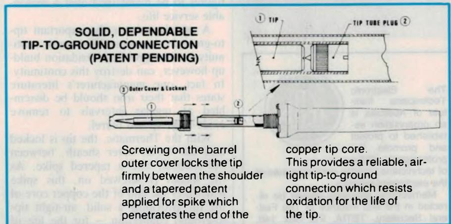
To ensure reliable long-term grounding of the tip, Royal's Thermatic iron uses a tapered spike, which penetrates the back of the tip.
