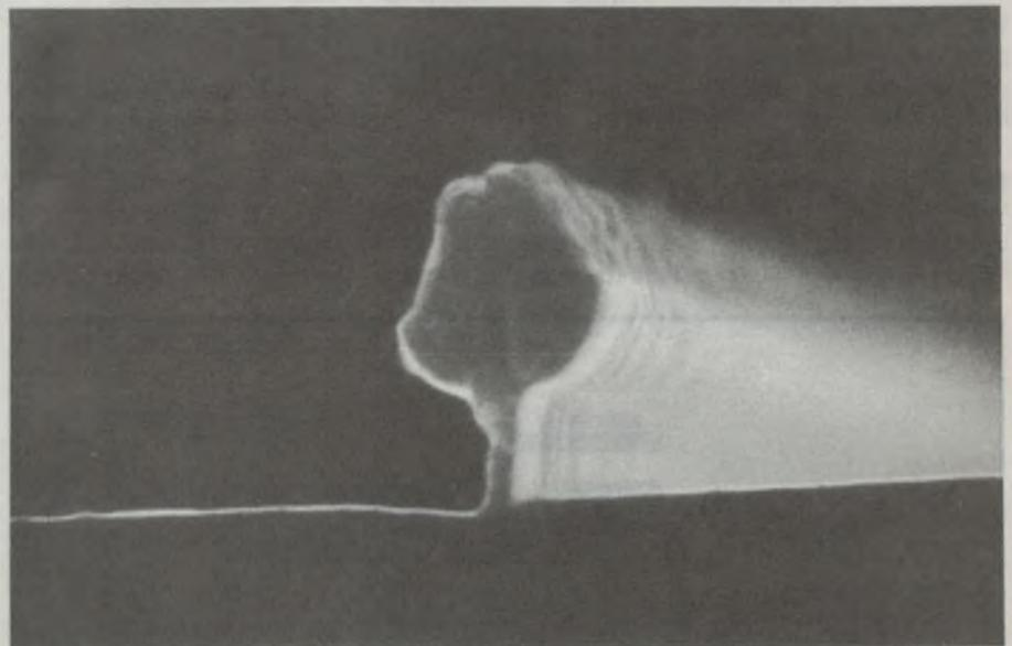
**Scanning electron microscope shot showing the cross-section of one of the Group's gate electrodes. The wide 'mushroom' at the top is about 0.7µm wide (long), and the base only 0.1µm. The latter is the effective gate length!**
