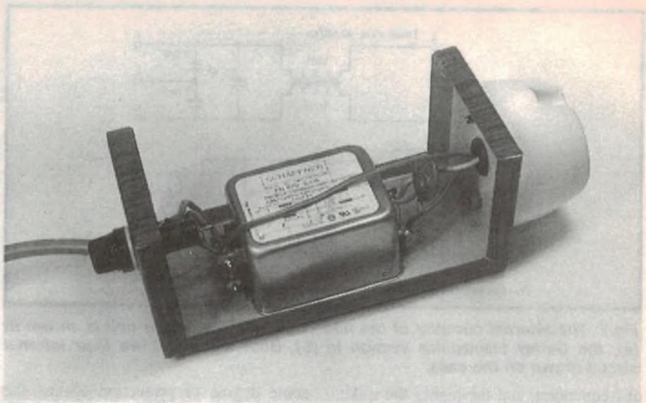
**Fig.4:** This photo shows the assembled unit, with the case cover removed. Anchor the incoming mains cord, and connect the active (brown wire) to the end connection of the fuse holder. Also make sure everything is well earthed.
