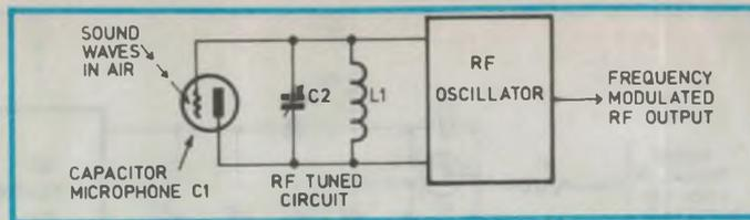
duced capacitance of C1 increases the RF frequency.
