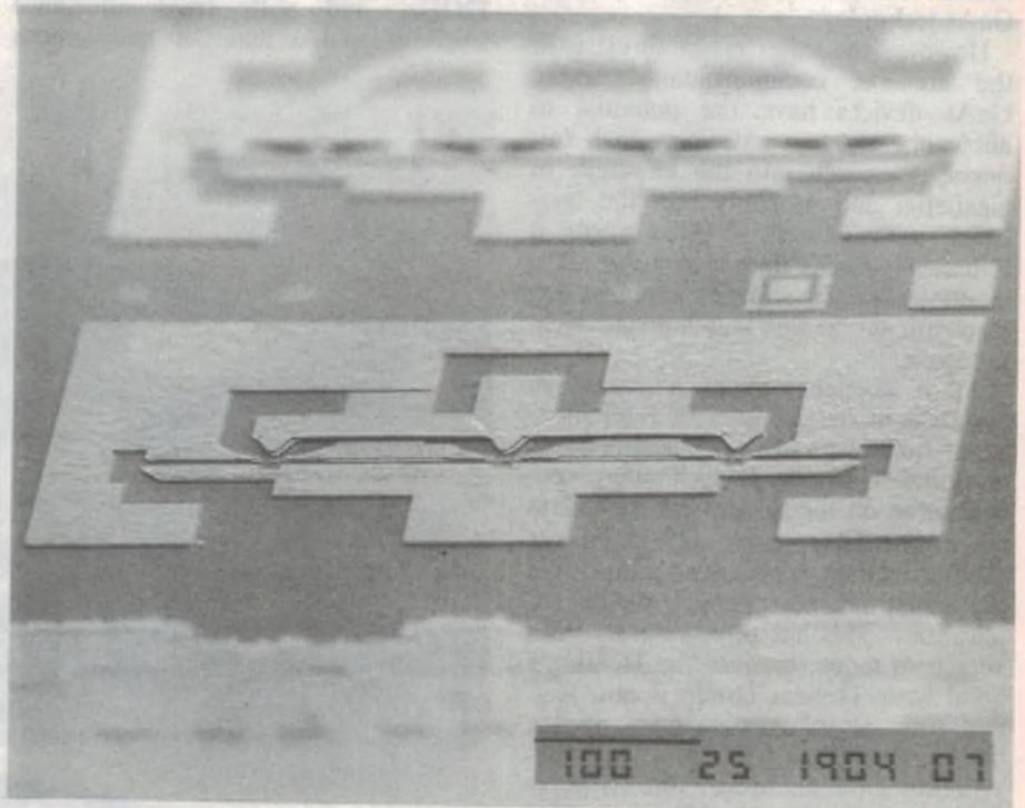
**A scanning electron microscope shot of a mm-wave MESFET. The gate electrode is only just visible as a very thin horizontal line across the centre.**
