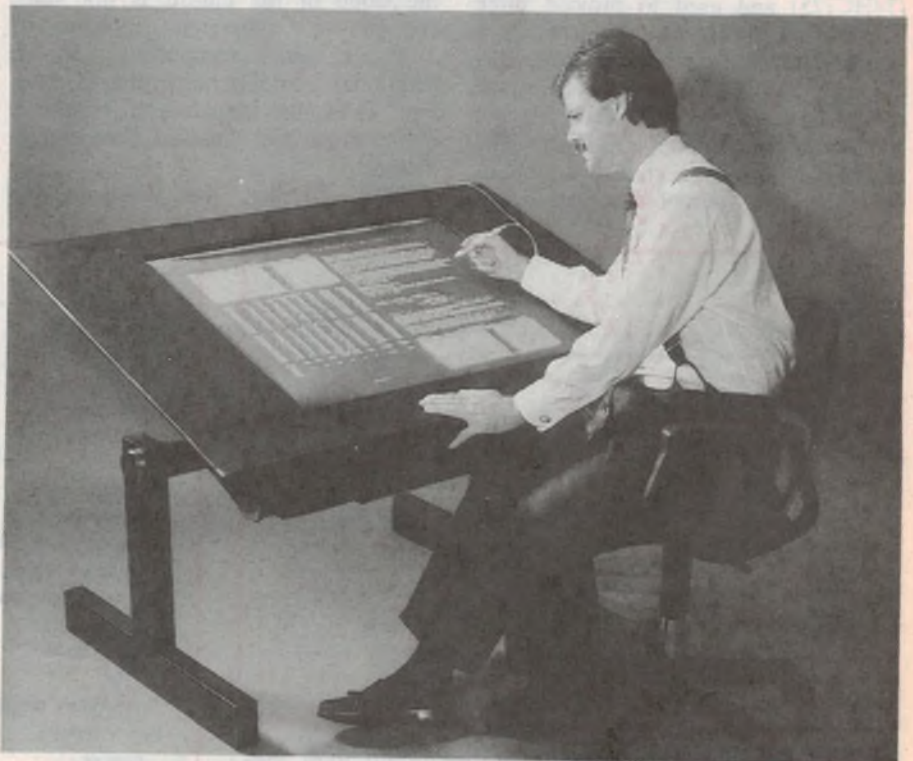
The PCP plasma workstation has a resolution of more than 3.5 million pixels, effectively forming an 'electric drafting board'.
