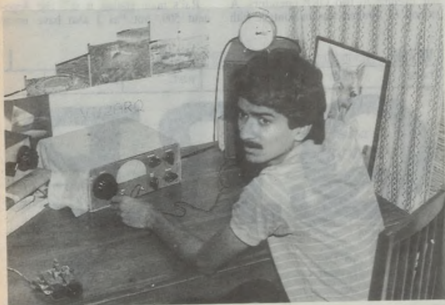
A keen QRP operator in Madras, Shrikanth VU2ARQ, built this QRP CW transceiver which has since enabled him to work many European stations.
