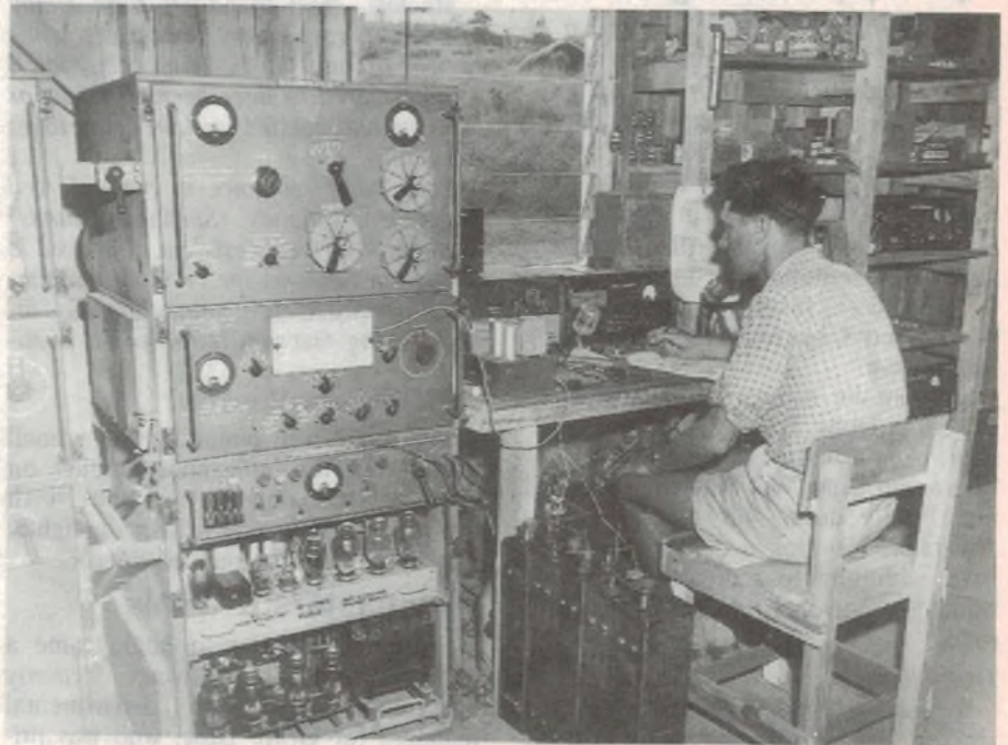
A shot taken inside a mission station at Rugli in New Guinea, around 1950. A CRMF transceiver is visible behind the operator's right hand; the large transmitter on the left is an ex-RAAF AT-13C. (Courtesy CRMF)
