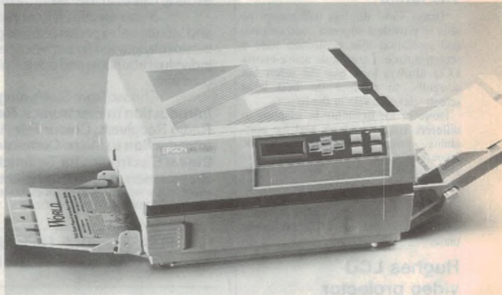
The new Epson GQ-5000 laser printer, just released in Australia and designed for desktop publishing. Based on a Motorola 68000, it prints 6 pages per minute and provides 13 internal outline fonts plus 11 bit-mapped fonts, in sizes from 2.16 to 240 points. It also provides Centronics, serial and video interfaces.
