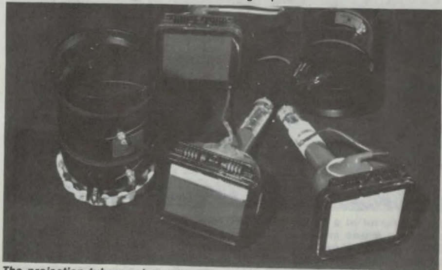
The projection tubes and matching lenses from a Barco video projector. The tube on the left has been partly drained of its cooling fluid.
