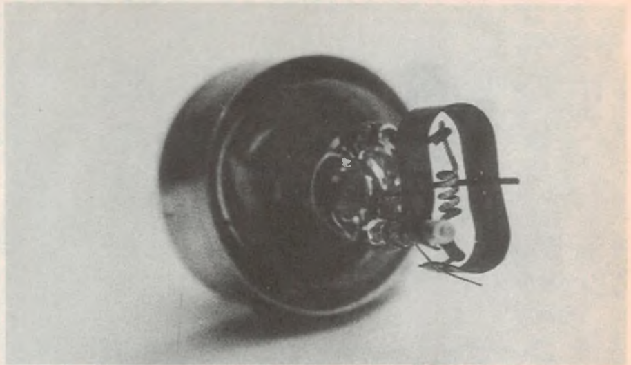
Another view of the lamp end assembly, showing the cathode filament inside its shield.
