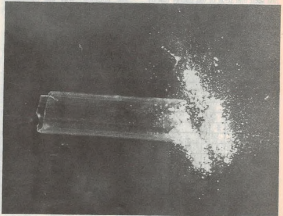
The phosphor is a white powder coating the inside of the glass tube. It can be tapped out of a broken lamp, as shown.
