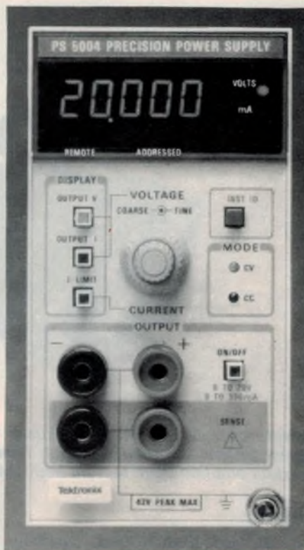
The compact PS 5004 programmable precision supply module from Tektronix is part of that firm's TM 5000 modular instrument system. It provides 0-20V at up to 300mA, with full IEEE488 compatibility. (Courtesy Tektronix)
