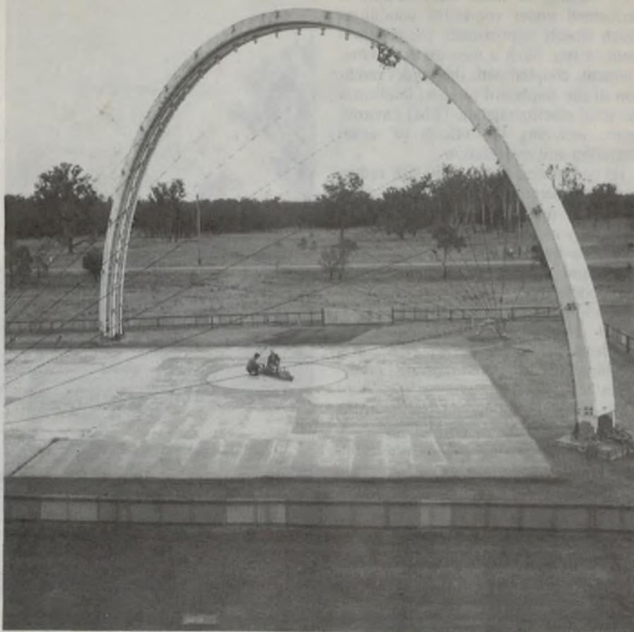
An overview of the test range, showing the large non-metallic arch used to support the moving transmitter antenna. Its plastic support cables are also visible. (Photo by George Hicks)
