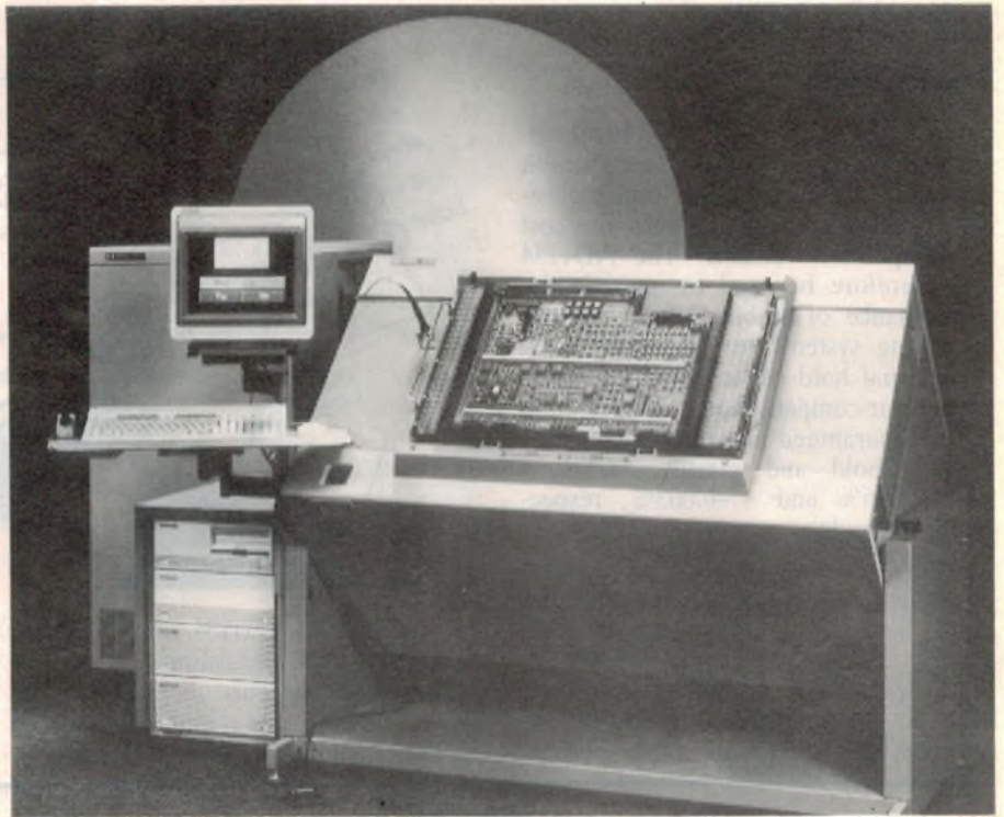
Hewlett-Packard's new HP 3070 combinational-board-test system, which can carry out fully integrated digital and analog functional tests on wired PC boards with up to 2592 circuit nodes.
