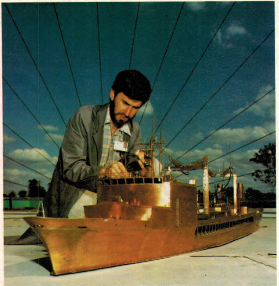
Adjusting a scale-model antenna on a ship model, in preparation for testing on the range. (Photo by George Hicks)
