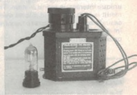
Fig.2: The companion Philips 1017 trickle charger for 'A' batteries, with its tiny mercury-vapour rectifier.
