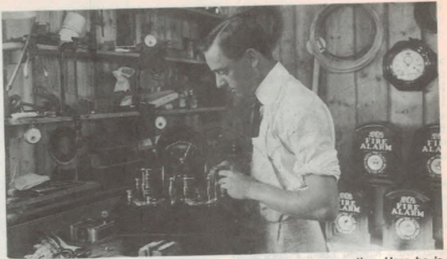
In 1913, Raymond Allsop joined Shaw's factory as an apprentice. Here he is shown assembling a spark transmitter.
