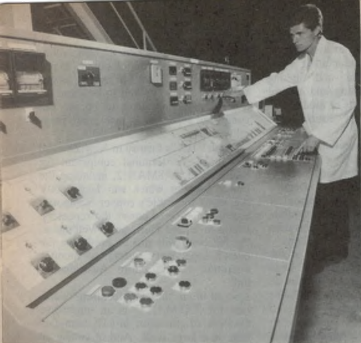
The control console for the 'composite' line, which includes winding on the steel wires and adding the copper conductor.
