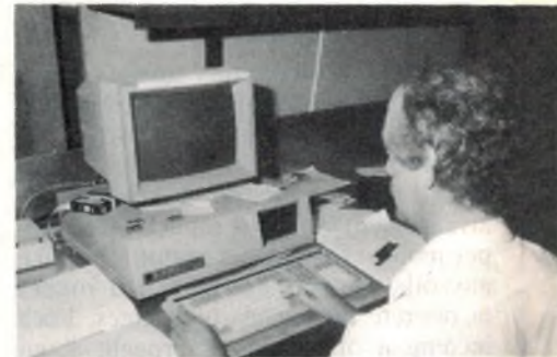
Dr Giles working on the plotter's software with an IBM-PC. The 6802 machine code is assembled on the PC and then transferred into the plotter's memory for testing.
