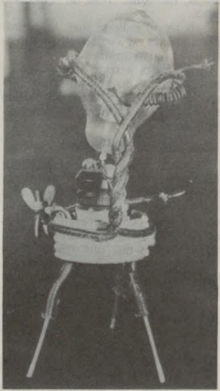
Fleming's first experimental diode detector valve, developed in 1904. It became the subject of considerable legal argument.
