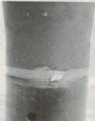
Fig.1B: Wrap a layer of 5A fusewire around the damaged shielding and solder to the earthing wire.
