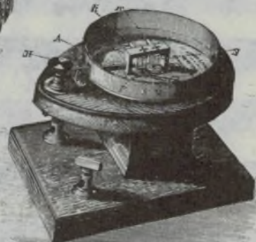
Fig.15: This Ayrton-Perry voltmeter uses gearing and has return springs. Perhaps you can figure out how it works!
