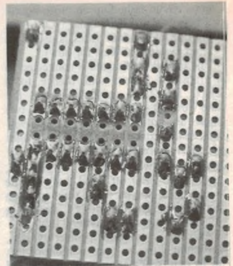
Photo 5: The copper side of a piece of Vero-board with our EA-Thing project wired up.
