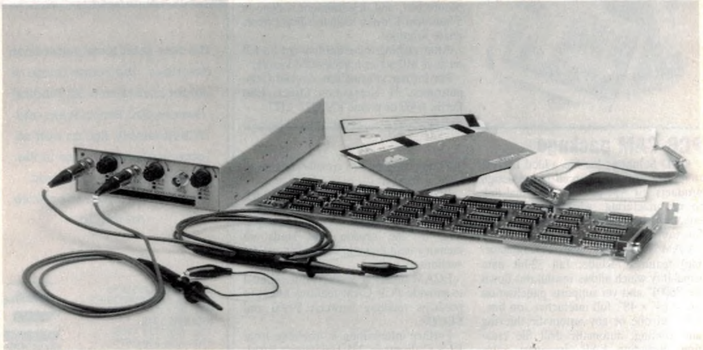
The complete storage scope package from Hilink. The card is installed in the PC's expansion slot, while the analog interface box sits outside the host computer or in a spare disk drive cavity.
