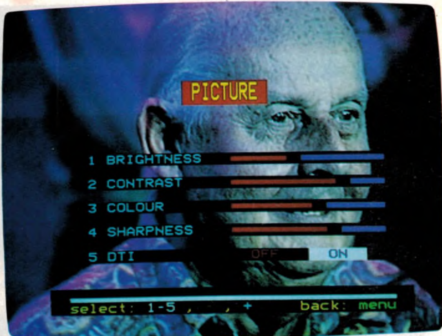
The picture menu with its 'slider' adjustments and the DTI (Digital Transient Improvement) selector. The sharpness control was quite effective.
