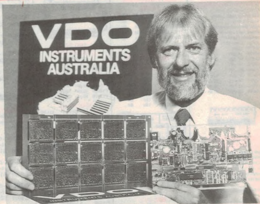
VDO's production engineering manager, Mr Tony Fruehwirth with samples of the first circuit boards manufactured by the company using a chlorofluorocarbon (CFC) free process.
