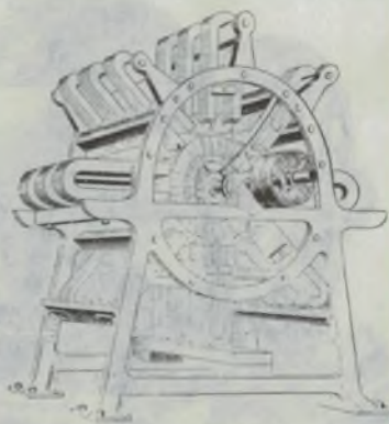
Fig.4: The construction details of the Alliance alternator shows the copious use of permanent magnets. This machine was intended to power the arc light in a lighthouse.
