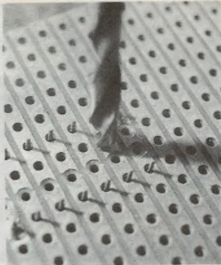
Photo 4: How Vero-board tracks can be cut easily using a twist drill as 'countersink'.
