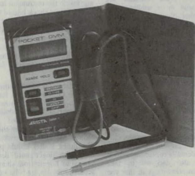
Arista's DMM-1 is a very compact autoranging 3.5-digit 'shirt pocket' model, smaller than many pocket calculators.
