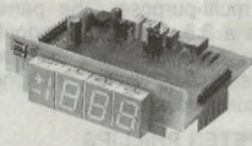
ATM28 3 1/2 Digit LED DVM ±199.9mV or 1.999VDC Jumper Sel. Bright Orange 1/2" Disp. .... $56.00
