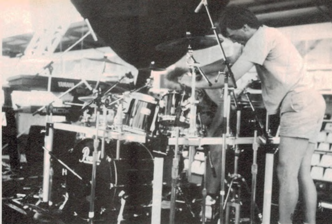
Part way through rigging the microphones. Although the cables are not connected, eight microphones are in position, each directed to just one drum.
