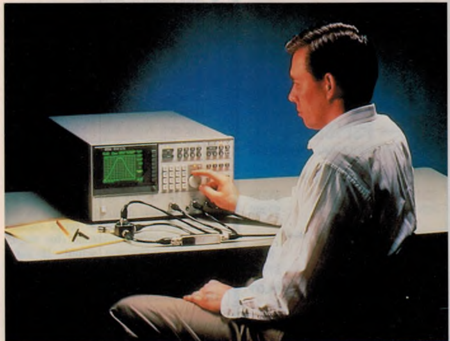
HP's 3077B Network Analyser, which can be easily programmed in 'Instrument BASIC' to perform comprehensive and accurate tests on both devices and subsystems, over the range from 5Hz to 200MHz.
