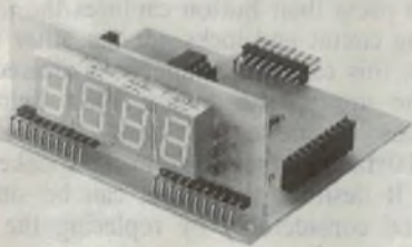
ATM13 Universal 4 Digit 4MHz Counter, bright Orange 1/2" Displays, Reset & Latch 5V 50mA ..... $54.50
