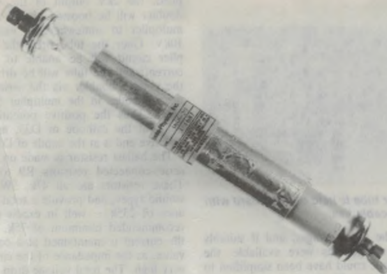
This photo shows a 4mW He-Ne laser tube that can be used instead of the 0.8mW tube described in the article. It's larger and much brighter.
