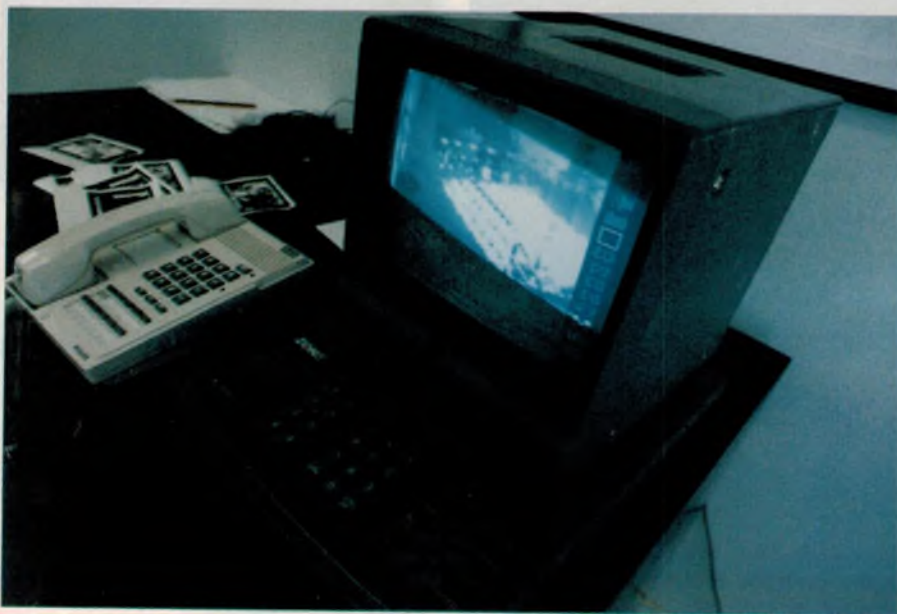
The receiver console, which can remotely control camera operation.
