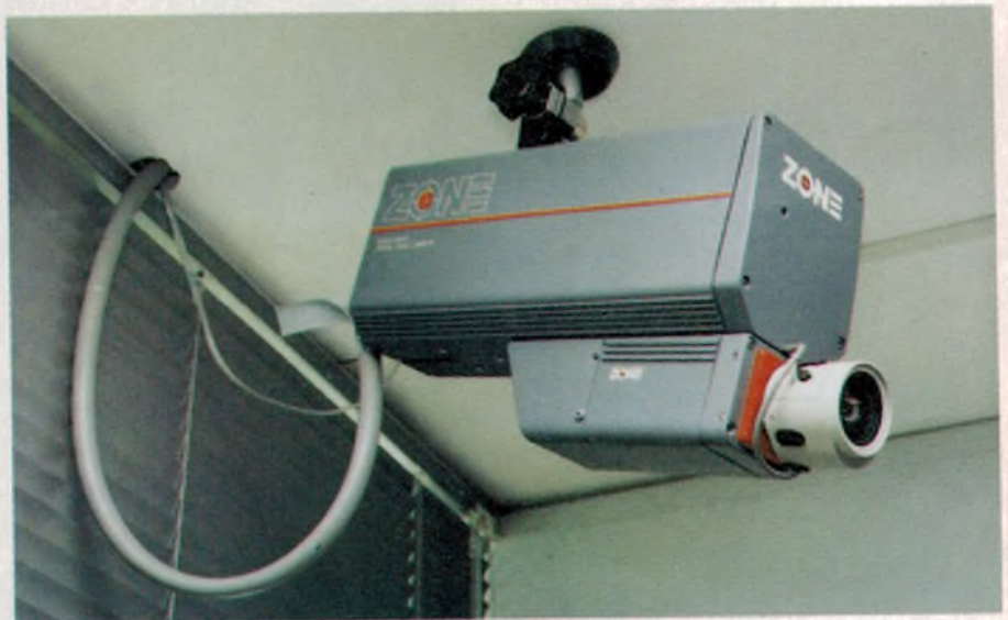
The master camera, equipped with an 85° coverage Fujinon lens. Note the two cables at rear: the thick co-ax is for satellite camera inputs, while the thin line is for phone output.
