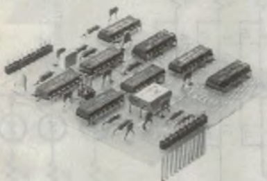
ATM15 Stopwatch/timer connects to ATM13 1, 1/10 or 1/100Sec at 9999 counts. Crystal controlled operated by switch, opto beam break (ATM20) ..... $44.50
