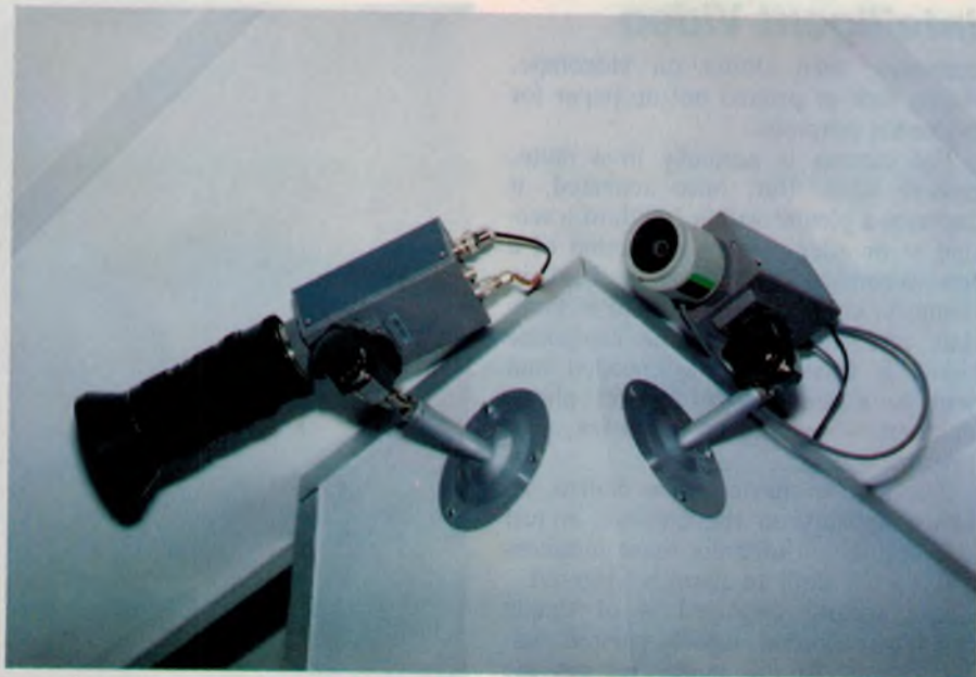
Two 'slave' or satellite cameras maintaining surveillance. Their pictures are passed on to the master camera.
