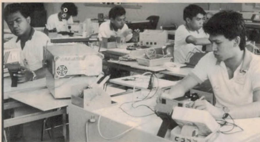
Testing automatic AC voltage regulators at Labrador Electronics Corporation, in Cubao, Quezon City. LEC also makes a range of uninterruptible supplies.
