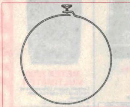
Fig.1: Hertz's receiver. This diagram from a 1906 book shows how the loop included a microscopic spark gap which discharged on receiving a signal. It has been estimated that at least 300 volts would have been necessary to create a visible spark. But with this elementary and insensitive equipment, Hertz was able to prove Maxwell's predictions of the behaviour of radio waves.
