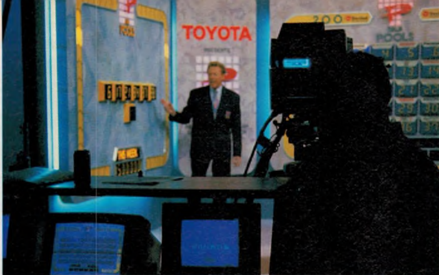
This studio action shot shows the screens of the two computers that control the game. If either fails, the other takes over automatically.
