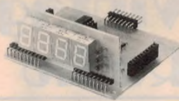
4 DIGIT COUNTER Universal Counter, 1 1/2" Bright Orange Disp. Rst & Latch 5V @ 50mA. ATM13.....$54.50
