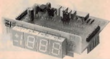
3 1/2 Dig. LED VOLTMETER ±199.9mV or 1.999V Single +5V supply ATM28 $56.00
