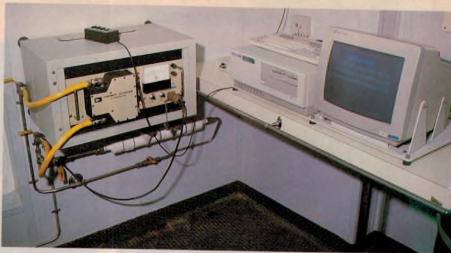
The fluorometer, used for continuous measurement of chlorophyll. The yellow pipes carry seawater from a sampling hole in the ship's hull through the instrument and back out again. Data is processed initially by the PC at right.
