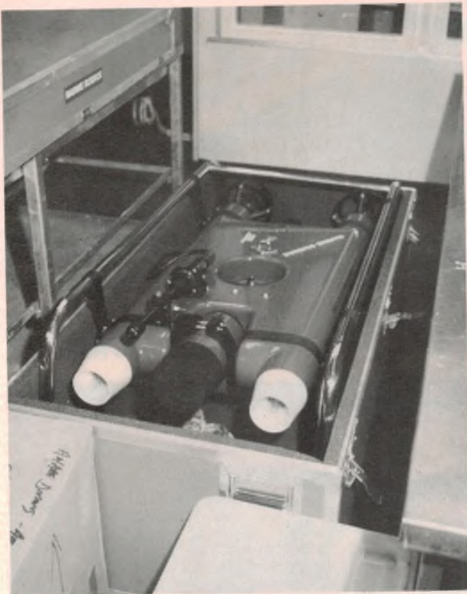
The submersible camera. The white tubes enclose strobe lights, above and below the camera lens – here wearing a dark lens cap.
