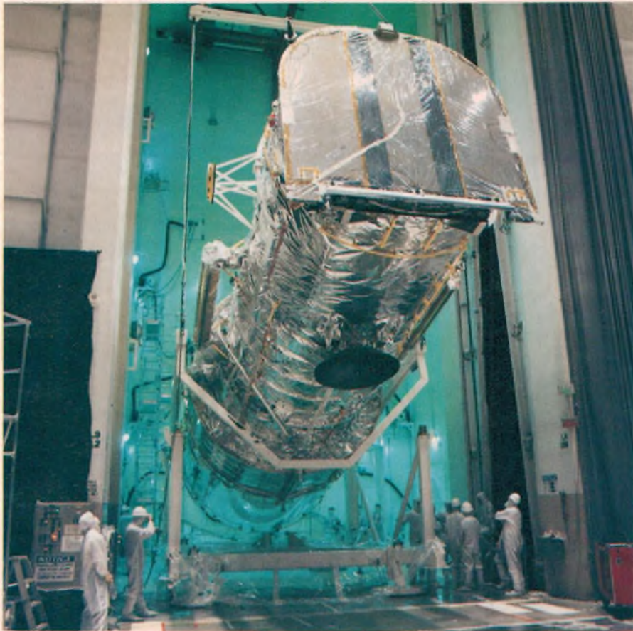
Manoeuvring the telescope assembly out of the lab, for transport to the Shuttle for launching. Note the protective wrapping.
