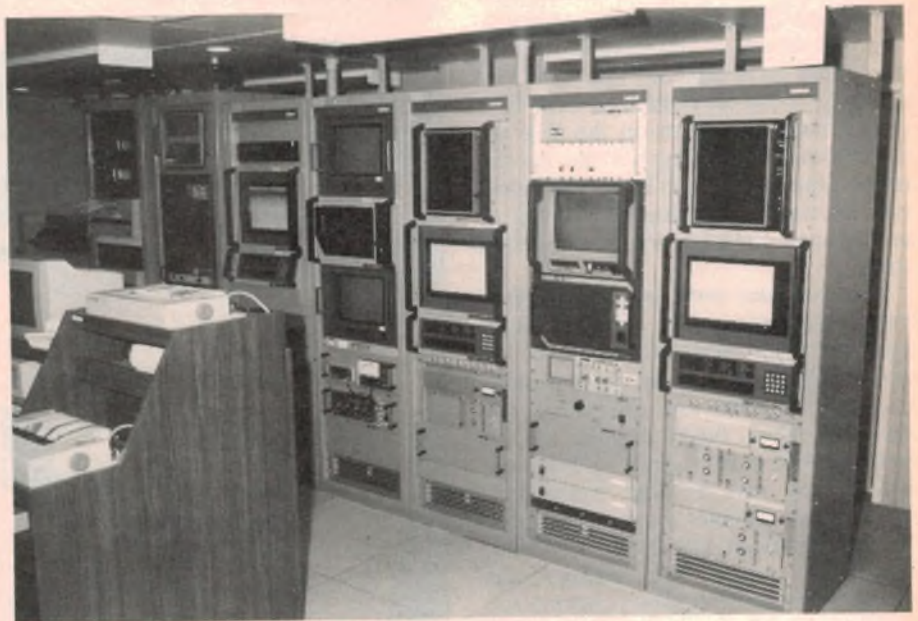
The 'acoustic' instrument rack, with the various depth sounders on the right, and the Hewlett-Packard computer on left.
