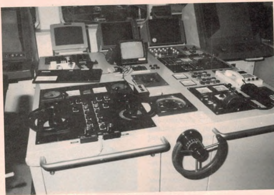
A closeup of the master console on the bridge. The small TV monitor shows a view from the top of the mast, where a remotely controlled camera replaces the traditional 'crows nest'.
