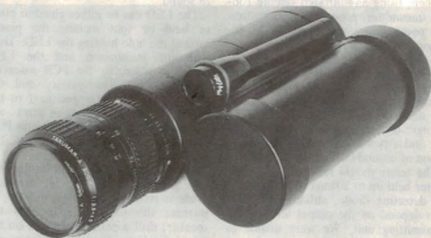
It's hard to believe, but this all new case for the infrared night viewer is homemade. Add a 35mm telephoto lens to the case and the result is a truly professional piece of equipment.
