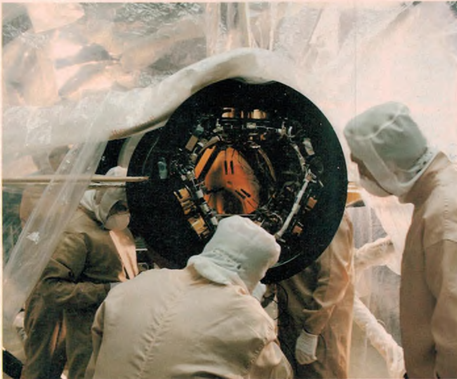
Making adjustments to the telescope's 330mm (13") secondary mirror, made by Hughes Danbury Optical Systems from a single piece of Zerodur.
