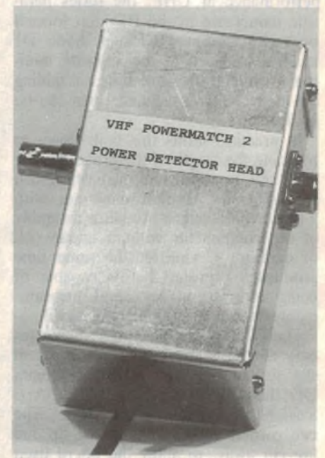
A shot of the assembled in-line RF power head, which fits in a small utility box. Maximum power is 12W.
