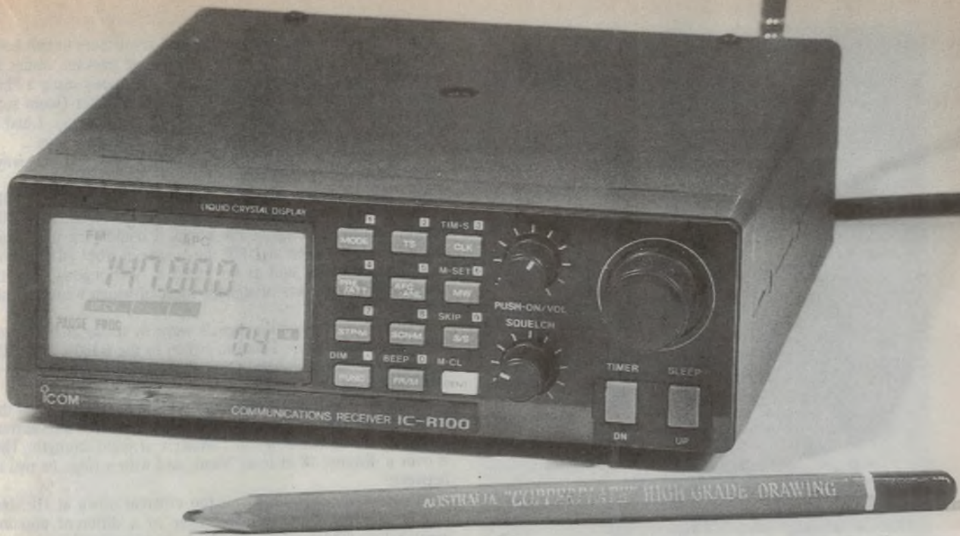
And here's the IC-R100, at very close to life size as you can see from the pencil. Note that the LCD contrast is much better than is apparent in this shot. This set tunes from 100kHz right up to 1856MHz.
