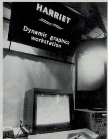
Quantel's new Harriet video graphics workstation – a dynamic setup with totally random access solid state storage.
