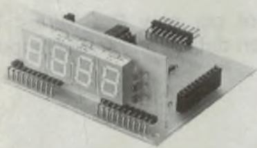
ATM13 Universal 4 Digit 4MHz Counter, bright Orange 1/2" Displays, Reset & Latch 5V 50mA ..... $54.50
