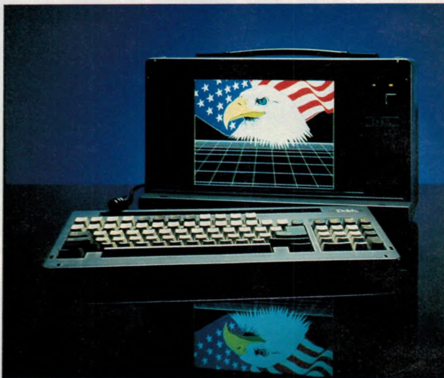
The active matrix colour display in Dolch's new 80486-based laptop portable provides a brightness and clarity very comparable with conventional CRTs.
