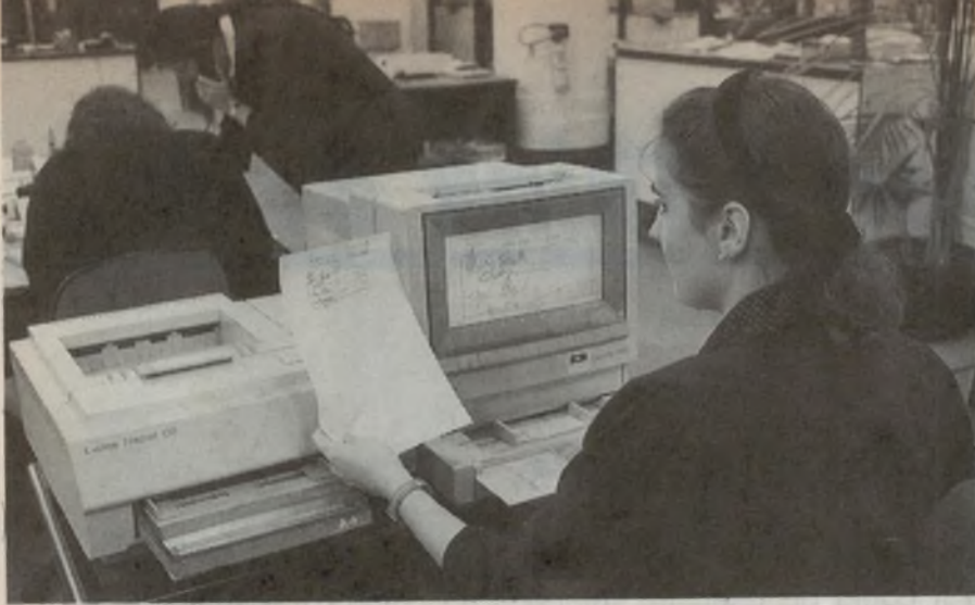
The Commonwealth Bank has installed three Canon 'Friday' systems in its Martin Place (Sydney) branch to speed up signature verification on cheques. The new systems use removable magneto-optical disks — each of which holds the equivalent of 12,000 A4 pages of information.
