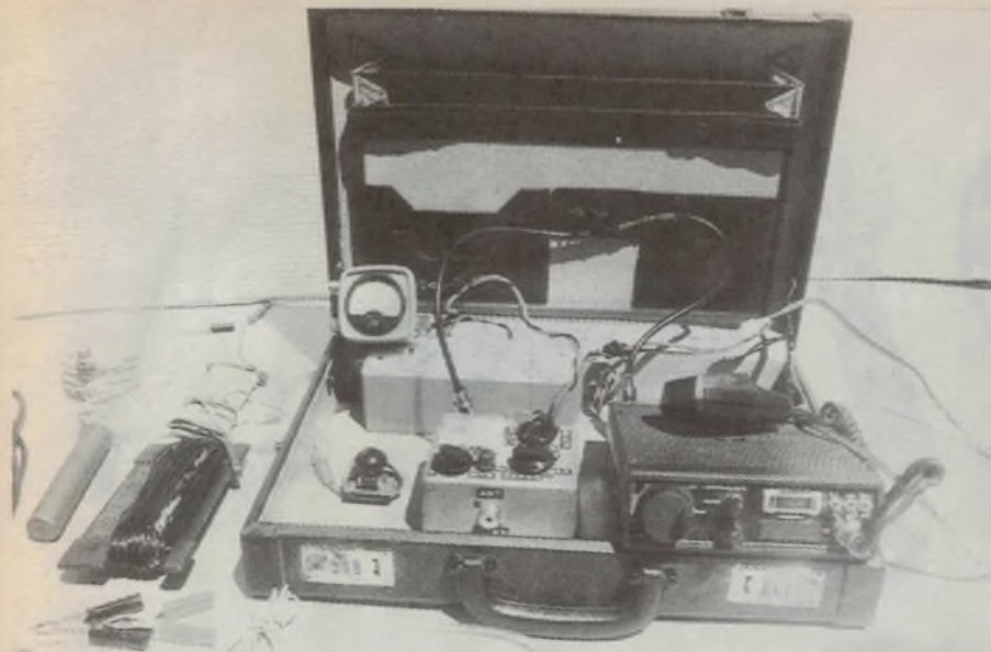
All unpacked and ready to operate – the author's briefcase station. The shot at lower left shows it when all packed up.
