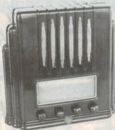
Fig.1: AWA's 1938 R52G Radiolette has a nicely proportioned bakelite cabinet. At some stage this one has lost its badge, but chances are that it can be replaced.
