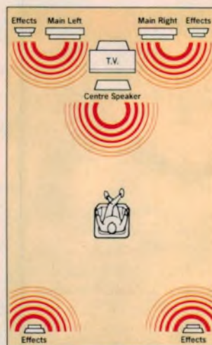
Multi-dimensional sound imaging created with a 7-speaker DSP-Dolby Pro Logic surround system.
