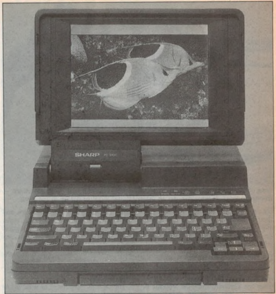
Sharp's PC-5500 laptop, which features built-in floppy disk and hard disk drives, together with a screen offering VGA-level resolution.
