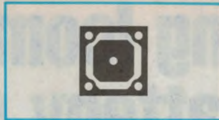
Here are the actual-size etching patterns for the two versions of the dummy loads – for the N-series socket (left) and the BNC socket (right). They're too small for coding!
