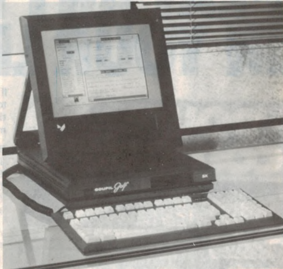
The Goupil Golf is a very compact new personal computer from Newbury Park-based Computer Peripherals Inc. Using the new 386SX processor running at 16MHz, it features a fold-up 10" backlit LCD screen plus 1.44MB 3.5" floppy drive and a 20MB, 40MB or 100MB hard disk.
