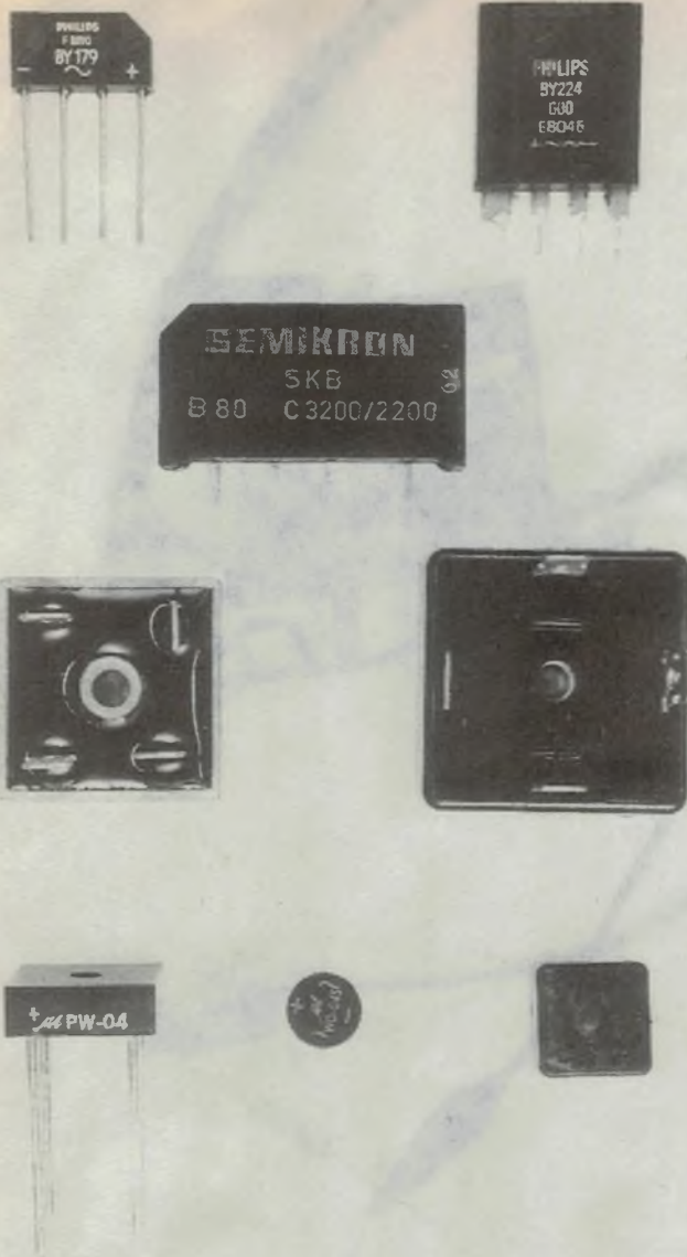
Fig.4: This photo shows the various package styles for bridge rectifiers. Those shown in the second row from the bottom can handle forward currents of 25A or more. The bottom row have a more modest current capability of an amp or so, and are commonly used in low power electronic circuits.
