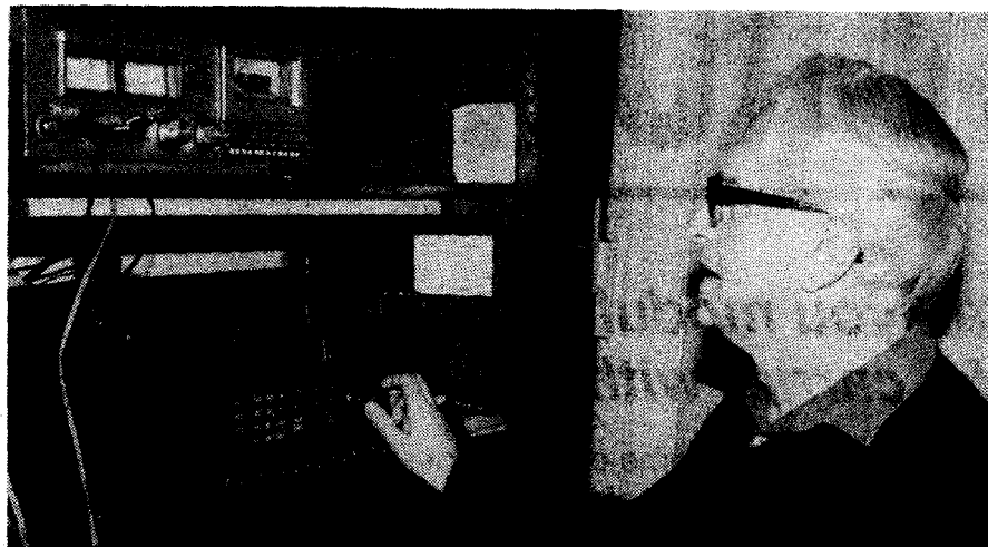
A Grundig 650 communication receiver is typical of a modern radio with keypad tuning, memories and a digital readout showing the time and frequency.
