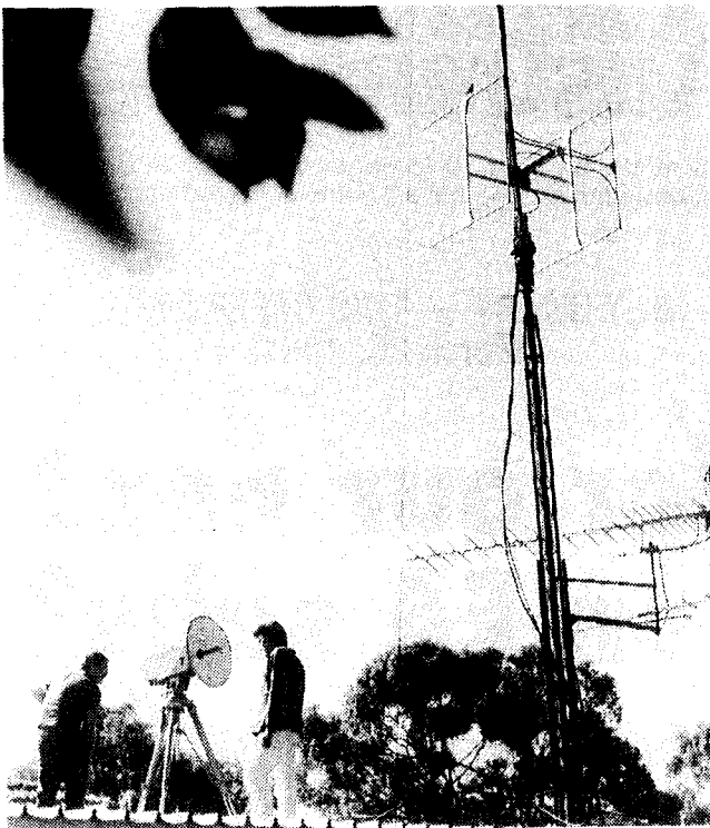
Left: technicians from the ABC set up a microwave link in the shadow of the high-gain UHF antenna system normally used by the Gladesville Amateur Radio Club for ATV transmissions. The microwave link took the signals to the ABC TV tower at Gore Hill. Above: The professional looking test card which was transmitted before the live broadcast.
