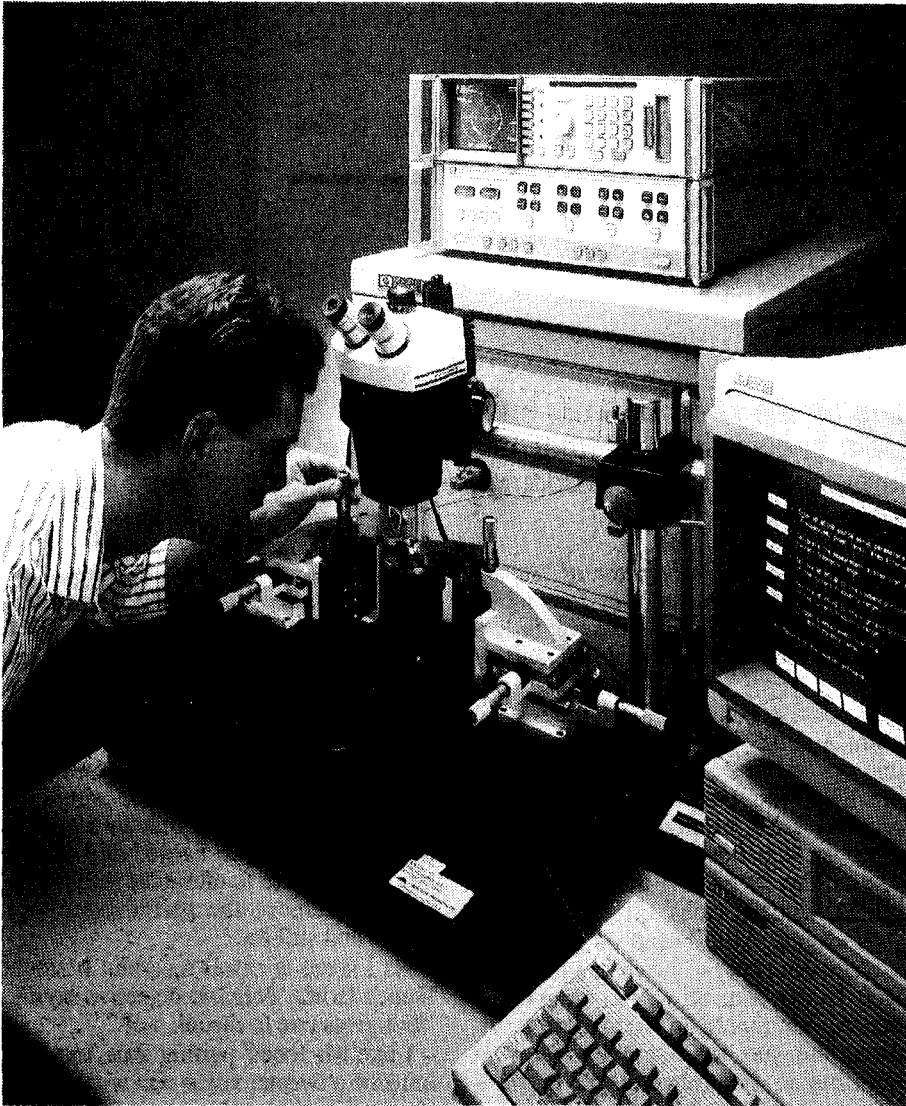
Hewlett-Packard's new HP85109B network analyser system extends semiconductor on-wafer broadband measurements of millimetre wave devices from 45MHz to 62.5GHz. The system provides greater than 63dB of dynamic range right to 62.5GHz and high power (minus 12dBm) at the probe tip to measure active devices requiring high test port power.
