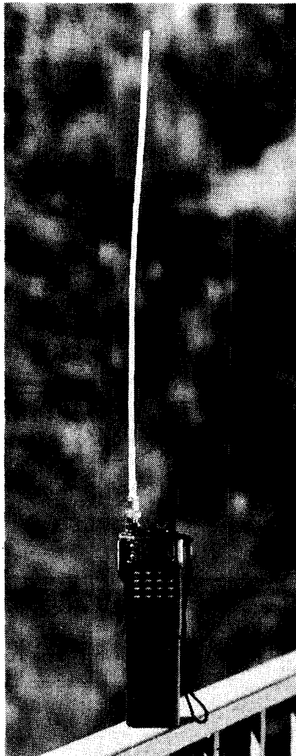
What we are making — the antenna mounted on an Icom IC-24AT VHF/UHF hand-held radio.
