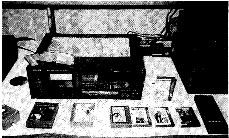
Louis took this close up shot of a Philips demonstration prototype DCC recorder, together with an array of software cassettes. This demo machine had a transparent panel in the top of the case.
