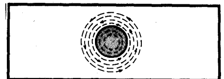
Fig.2: Current flowing in a conductor produces a magnetic field, which is strongest at the surface.
