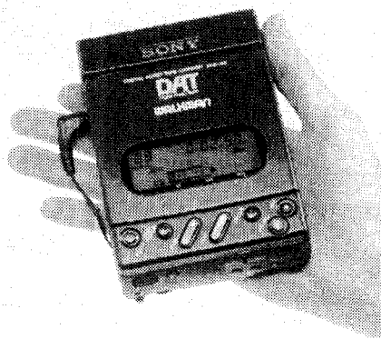
Sony's TCD-D3 digital Walkman, a complete record-play DAT machine in surprisingly compact form.
