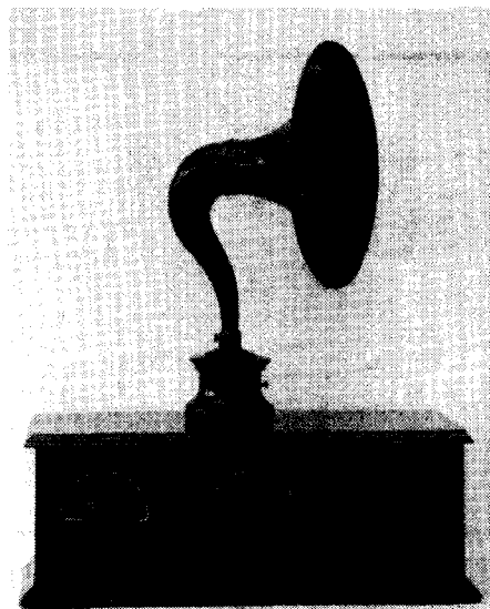
Fig.1: In 1925, domestic receivers had not become pieces of furniture. With its metal panel and lack of ornamentation, the Stewart Warner 300 was strictly functional in appearance.
