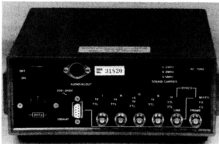
Rear view of the colour bar/pattern generator, showing the six component video BNC connectors with their level selection switches at bottom right. Also visible is the DB9 output connector and the sound carrier frequency switch.
