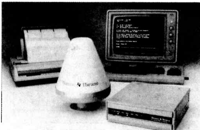
A typical Inmarsat-C terminal, from Thrane and Thrane.
