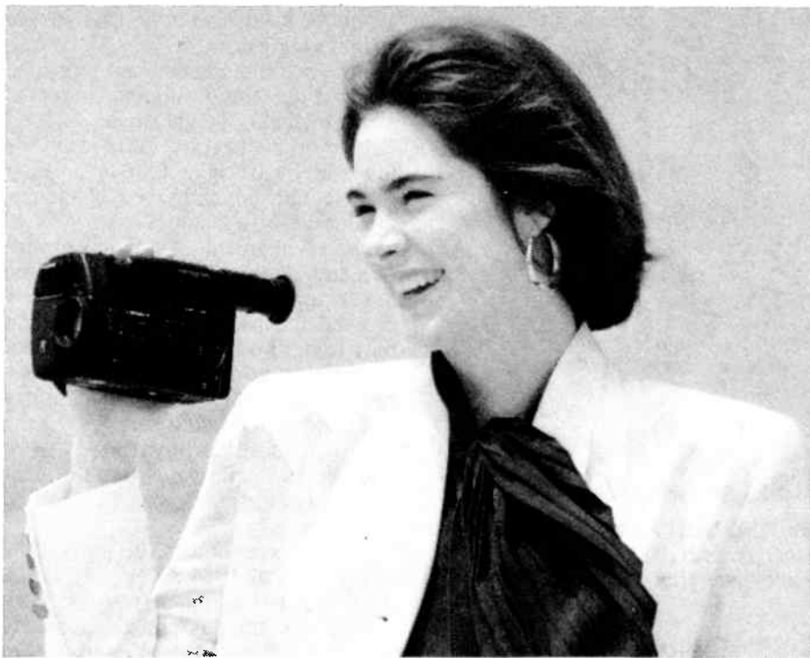
This photo shows just how small the TR-55 Handycam really is. The miniaturisation was the result of a management demand to shrink the internals to 75% of the previous model.
