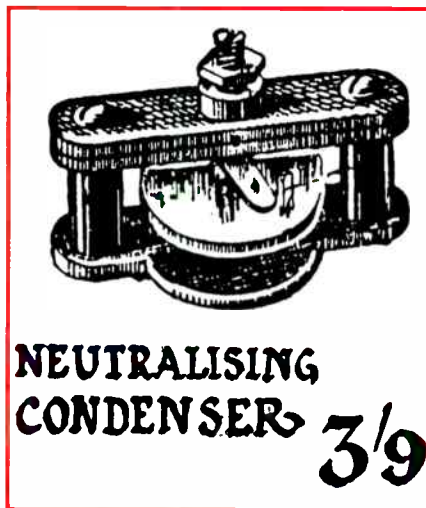
Fig.4: Pictured here about actual size, neutralising condensers (capacitors) offered an open invitation for experimenters to 'fiddle', often to no good purpose.
