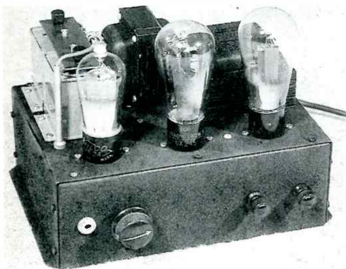
A surviving Loftin-White amplifier, very similar to the Electrad version of Fig.3. The wiring techniques are typical of 1930.
