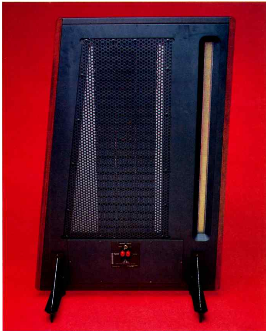
The rear of one of the 'Stage' loudspeakers, showing the support brackets, the input terminals and tweeter level switch, and the rear openings for each driver element. The wide darker band down the centre of the mid-range driver is the array of magnets, cemented to the perforated steel back panel.
