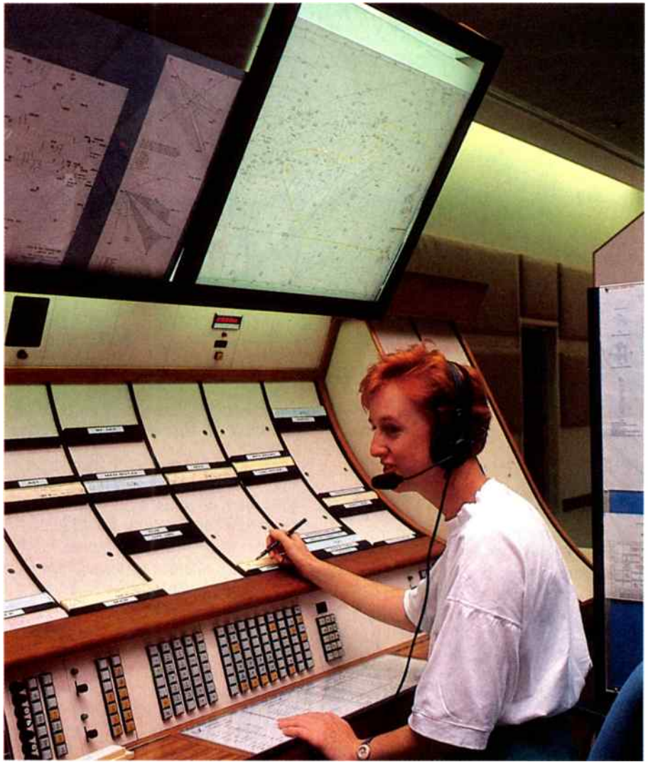
This is the procedural control console. The pilot submits a flight plan in advance and then files this path, notifying 'reporting points' along the way.
