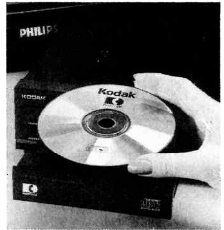
Apart from having a gold coloured metallisation, Photo CD discs are virtually identical with audio CD's.
