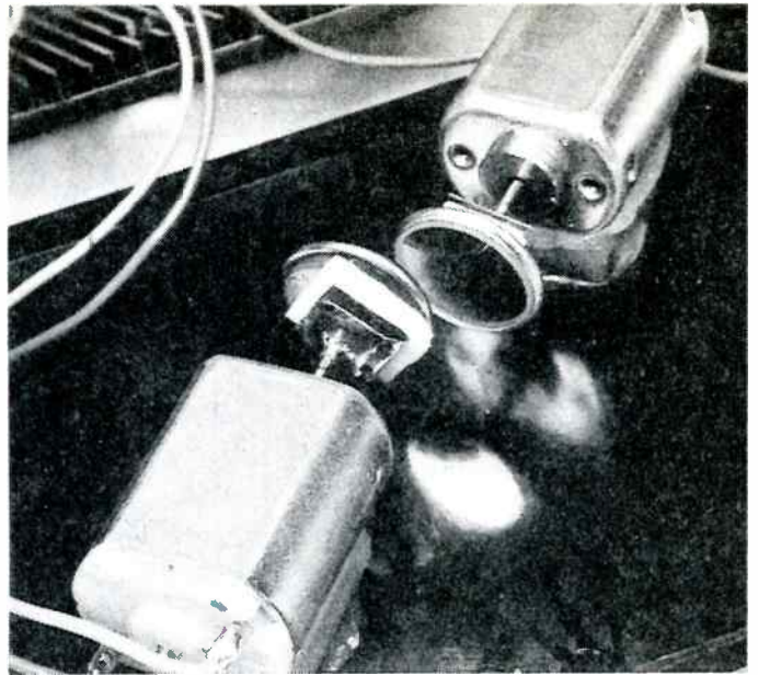
Fig.8: A close up shot of the motors. Dental mirrors were used on the prototype, available from most dental suppliers. Mirrors will be supplied in the kit for this project.
