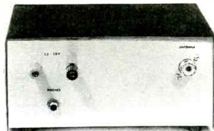
The rear panel is not exactly cluttered. The battery connections and phone socket are on the left with the antenna input on the right.
