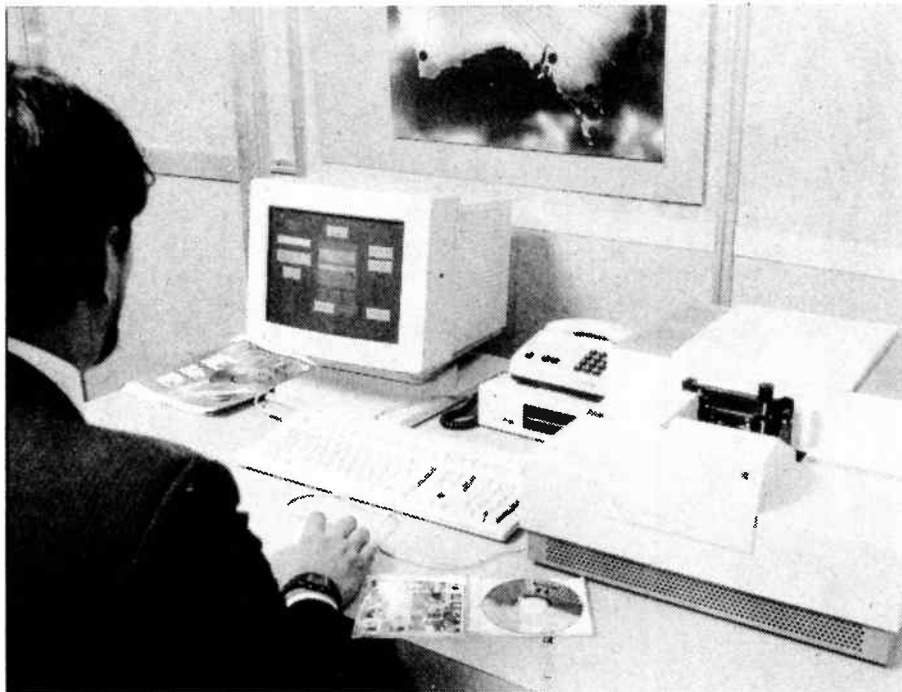
Using Kodak's Photo CD workstation, the photo-finisher can transfer each image from a film transparency or negative onto a CD, cropping and enlarging as desired. Up to 100 images can be stored on a single disc.
