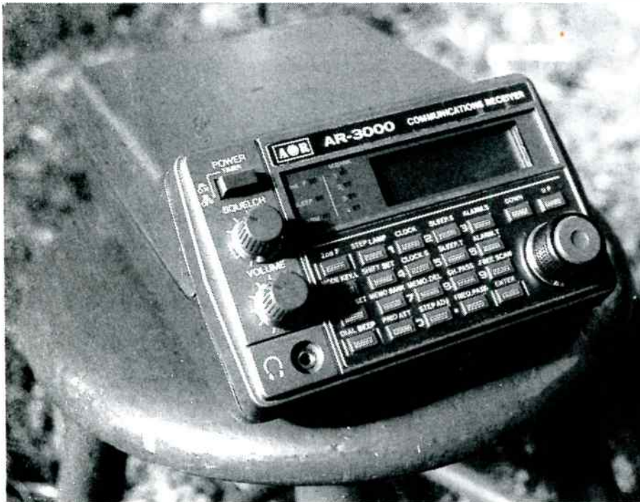
The author's AR-3000 scanning receiver. In this first of two articles he describes how to monitor its operation and control its reception simply and easily from a PC, using some short BASIC programs and an interface cable.
