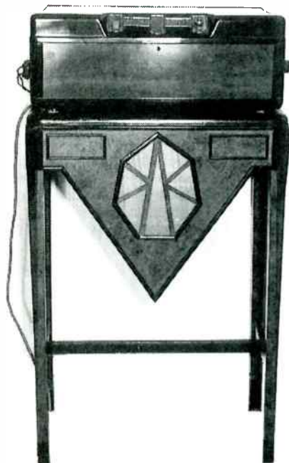
Fig.1 (right): The 2510 was very popular when combined as shown here with the 'Sevenette' magnetic (moving iron) speaker.
