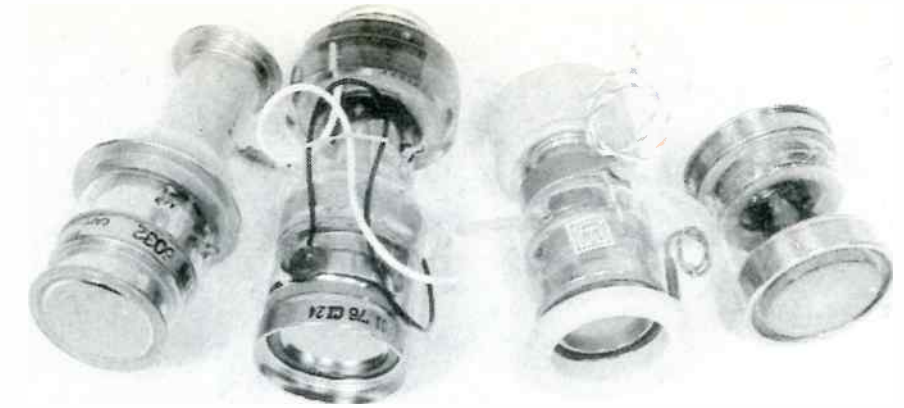
Fig.3: There are various IR tubes available, as shown in this photograph. The BWB448 tube, described in this article is shown in the centre. The 6032 and 6032A tubes on the left can also be used. The Phillips fibre-optic coupled tube on the right has a greater sensitivity and doesn't need a focus voltage.
