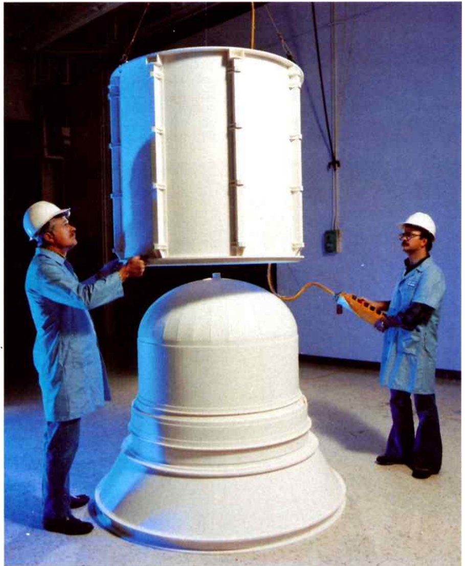
Technicians integrate components of an F-Sat mockup. The F-Sat bus design will feature simple aluminium construction, a high degree of access to components plus the ability to handle very high (2kW+) power demand.
