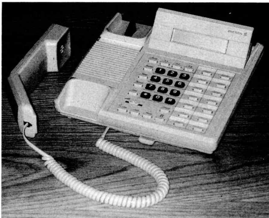
Calling Line Identification (CLI) is one of the new facilities offered by modern display phones such as this model from L.M. Ericsson.
