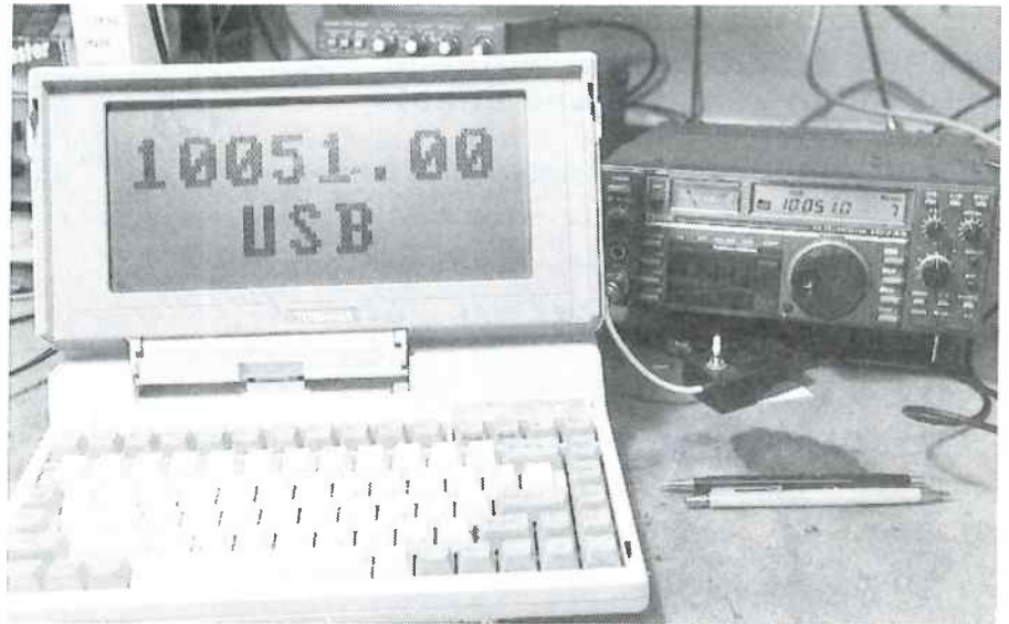
The 'Bigchars' program as it looks on the LCD screen of a Toshiba laptop computer.
