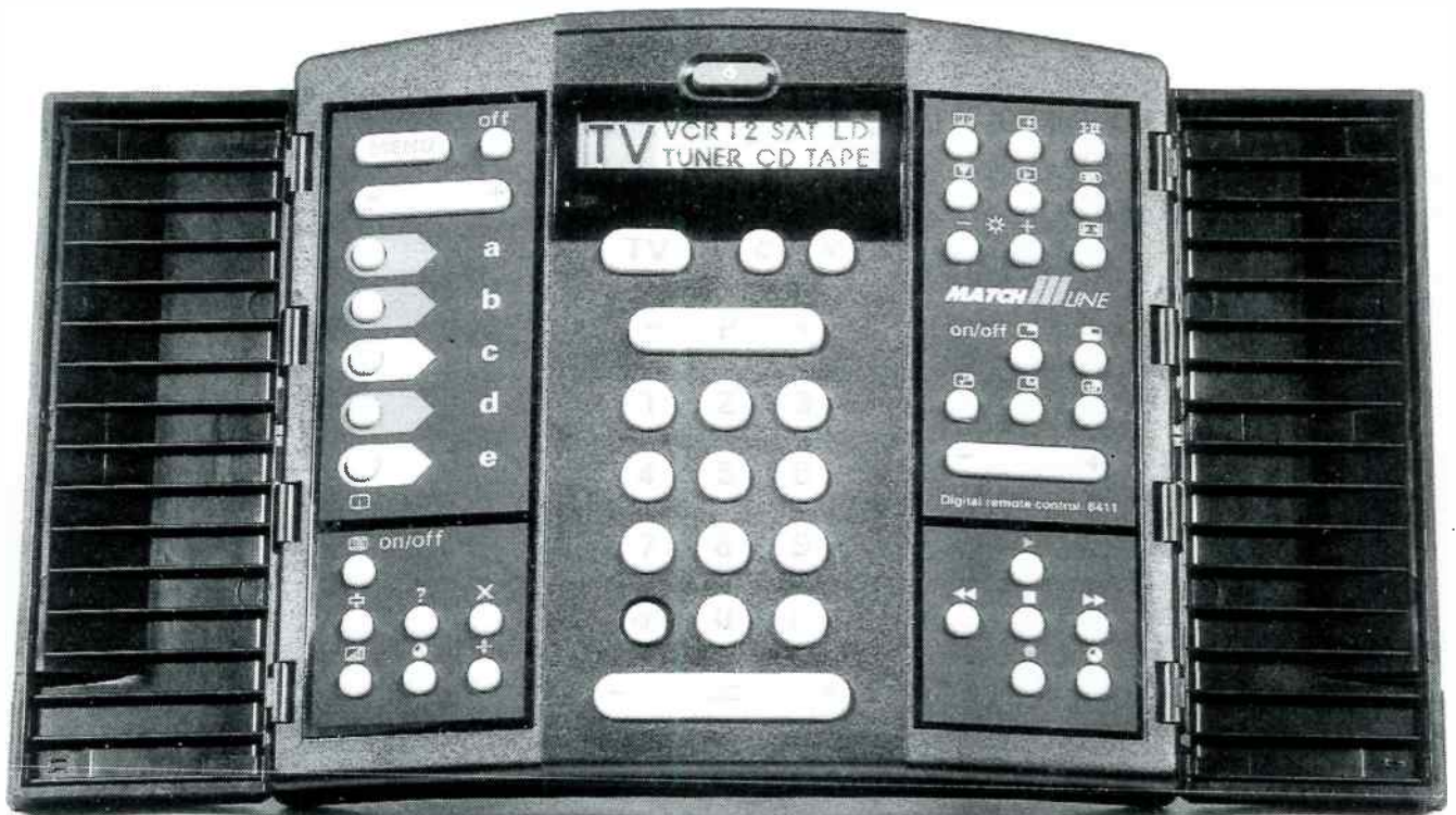
The Matchline's remote control shown with its side 'flaps' open. The most commonly used buttons are gathered in the centre of the unit, while the more specialised function buttons are normally hidden under the flaps. Note the LCD screen at the top of the unit, which shows the remote's current mode.
