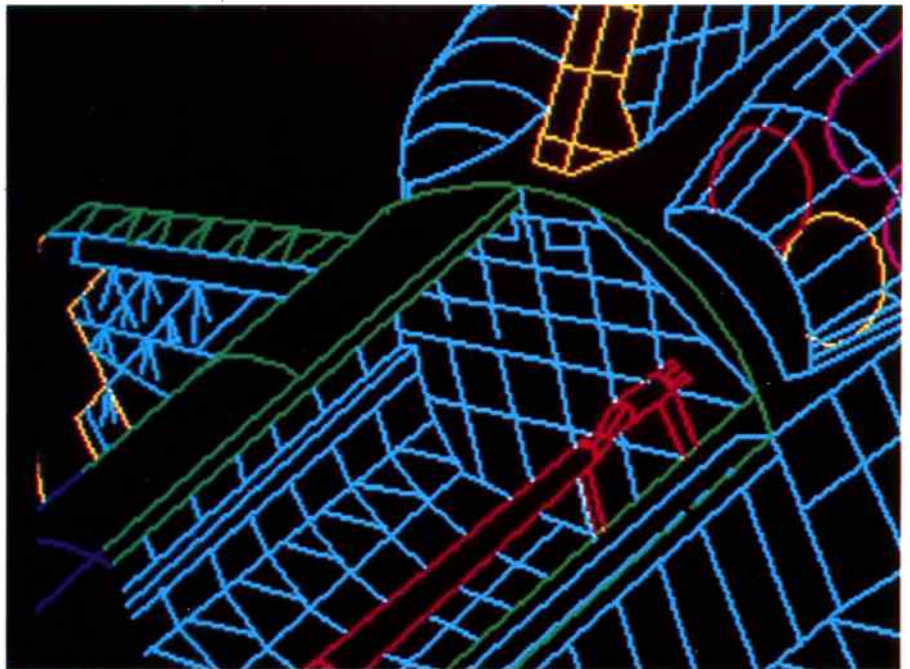
Fig.1: Detail from a CAD image displayed on a standard S-VGA video adaptor, showing the 'jaggies' produced by scan aliasing.
