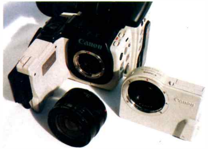
The EX1's body, with a 24mm SLR lens and the necessary adaptor.
