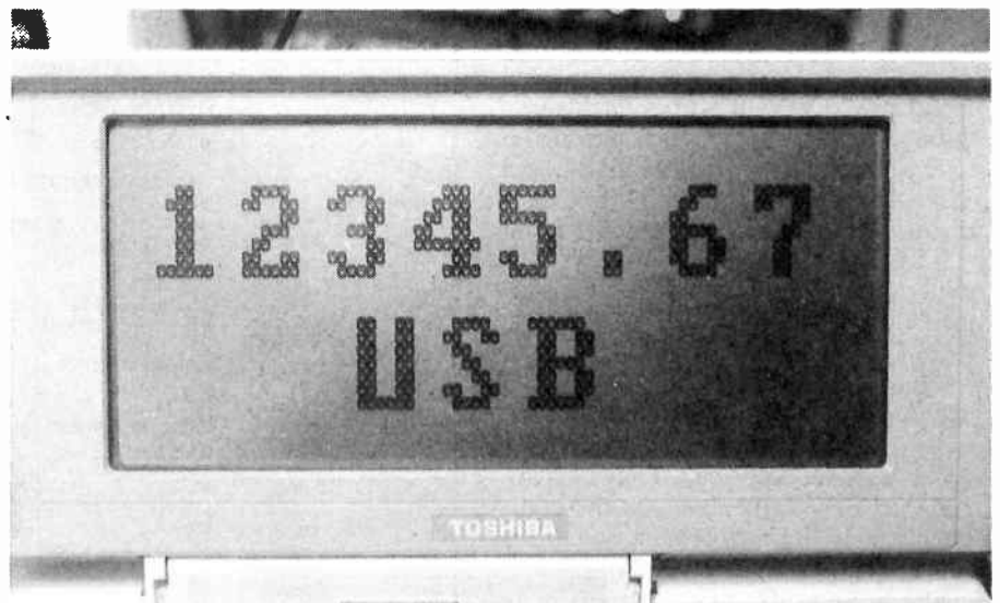
A close up shot of the characters generated by the 'Bigchars' program, as it looks on the LCD screen of a Toshiba laptop computer. As you can see, the characters have been made up of 'smiley' faces.
