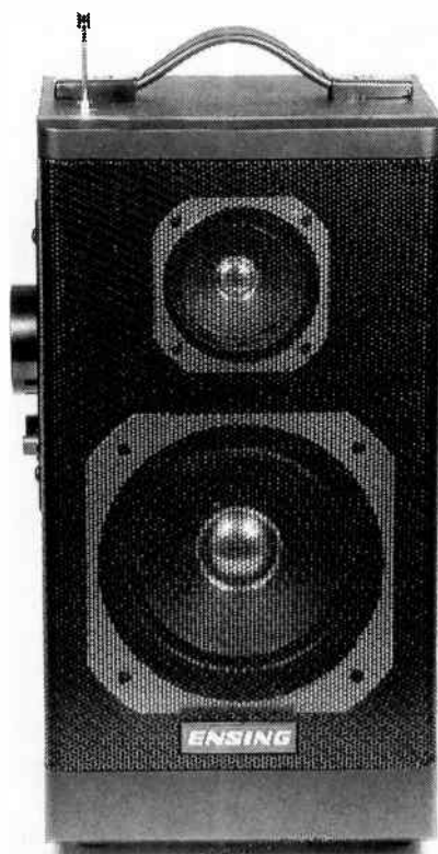
The unit's 'rear' panel showing the internal tweeter and woofer speakers. Note the telescopic antenna on the top panel.
