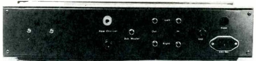
Fig.4: For the prototype, the Input and output sockets were mounted on the rear panel of the case, with RCA sockets for signals and terminal posts for the speaker. The sockets needn't be insulated from the panel, but all terminals are.
