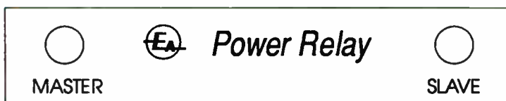
The label for the front panel. The circles are the mounting holes for the two neon bezels.
