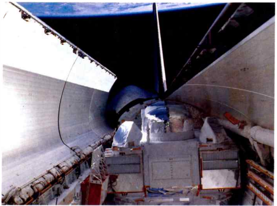
The GRO still sitting in the Space Shuttle's payload bay, with the doors opening for deployment. The shot below shows it being lifted out of the bay. Both shots were taken through the windows of the Shuttle's aft flight deck.
