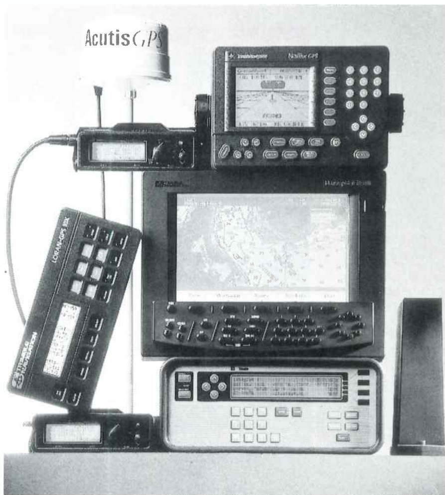
Some of the navigation receivers produced by Trimble Navigation. Most are equipped for GPS, in some cases in combination with other services such as LORAN and Omega.
