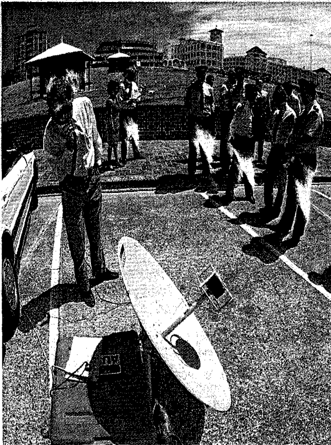
Another shot taken during the Bondi Beach tests, showing the Intelsat-A system being used. As you can see, even this system is reasonably compact and portable.
