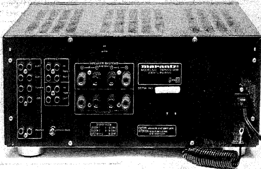
The rear end of the PM-72 looks rather like that of many other amplifiers. However there are two sets of loudspeaker outputs, selected by front panel pushbuttons, and also a coiled lead to earth other components such as a CD player.
