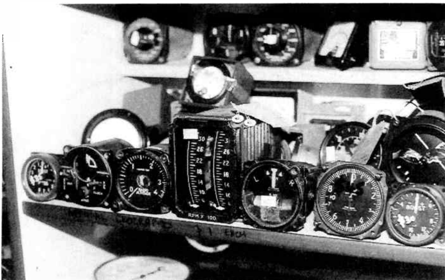
A collection of old aircraft instruments displayed at a second-hand store on Sydney's northern peninsula. Some of these instruments also turned out to be quite 'hot', again by virtue of their radium-zinc luminous paint.
