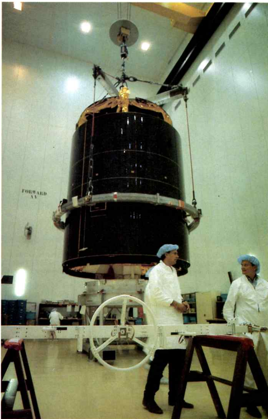
In this shot taken during the preparation of an INTELSAT satellite similar to the VI F-3, the 'capture bar' which will be used by astronaut Pierre Thuot is visible on trestles in the foreground.
