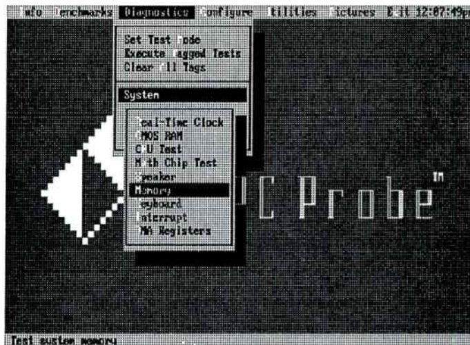
PC Probe's main screen with its elegant mouse-driven, pull-down menu system.
