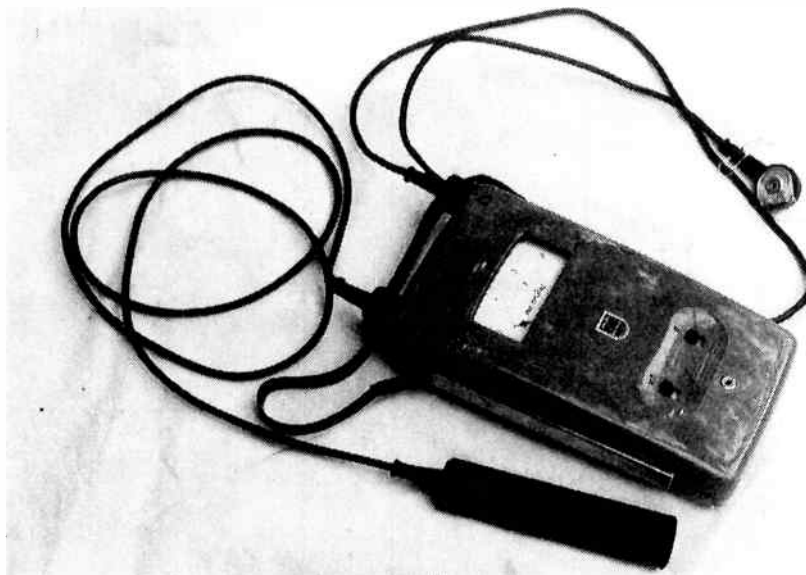
Here is the elderly Philips Geiger Counter, purchased by the author many years ago from a disposals dealer in South Australia. After replacing all of the original capacitors, it was restored to useful life — but told a disquieting story...
