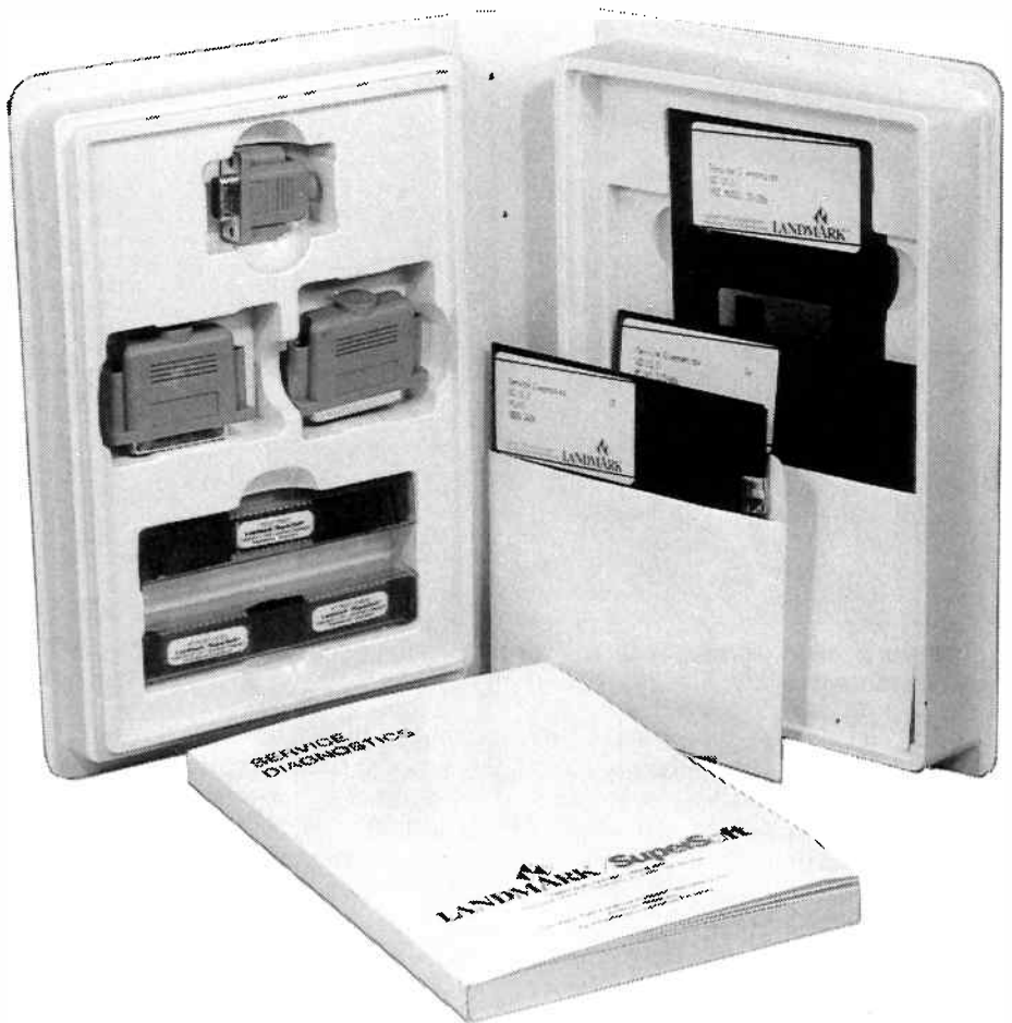
The SuperSoft diagnostic kit comes complete with serial port 'loopback' plugs (as does PC Probe), and a set of dedicated POST ROMs to replace the system BIOS chips.
