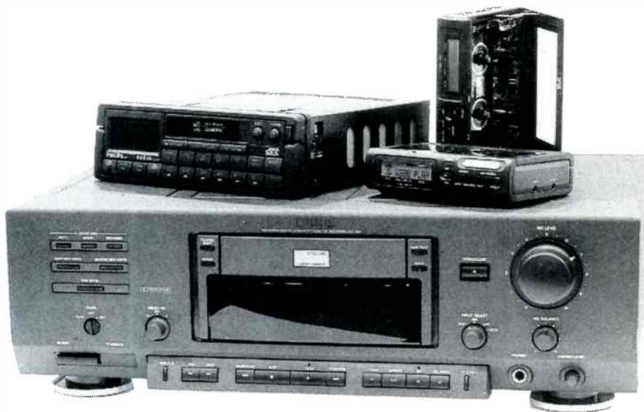
Among the DCC products displayed on the Philips stand were a high level recorder, fitted with Dolby B and C noise reduction, a car stereo system fitted with the radio data system (RDS), and a 'personal portable' recorder.
