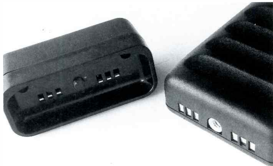
The base of the camera mates with the host adaptor, for charging the internal NiCad cells and also downloading the stored images to the computer via a serial port.
