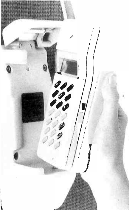
A close up of an SIA Celestel sky phone. Using the system in conjunction with Inmarsat's global satellite network, flight crews can contact control towers worldwide.
