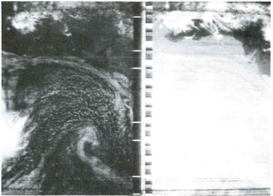
Photo 2: A picture from an American NOAA satellite, showing the same scene as in Photo 1 but taken several hours later. There are two separate images, with the one on the left showing that taken by the visible light camera and the one on the right by the infrared scanner.
