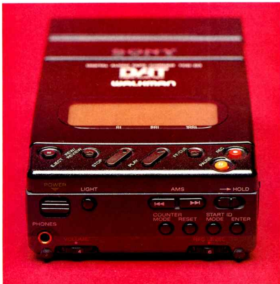
A close up of the main control area of the TCD-D3 recorder. The deck control buttons are along the top, while the functional controls such as track search, start ID and recording level are on the front itself.
