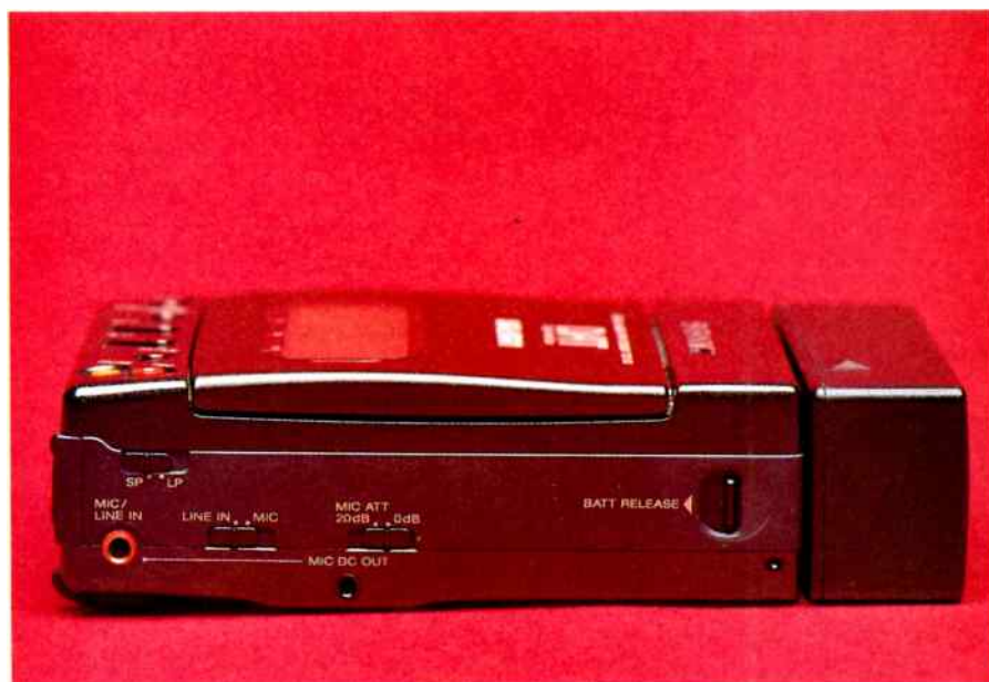
Along the right hand side of the case are the mike/line input socket, and control switches for input level and recording speed. Also available, as you can see, is a socket for supply of DC to a high quality capacitor microphone.
