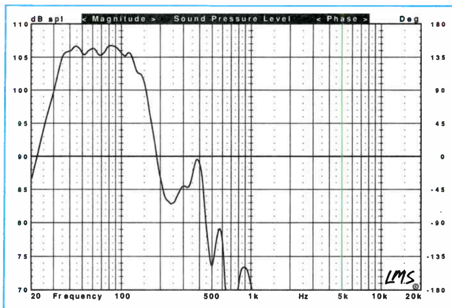
The sub-woofer's frequency response measured in a typical listening room — you really couldn't ask for better....
