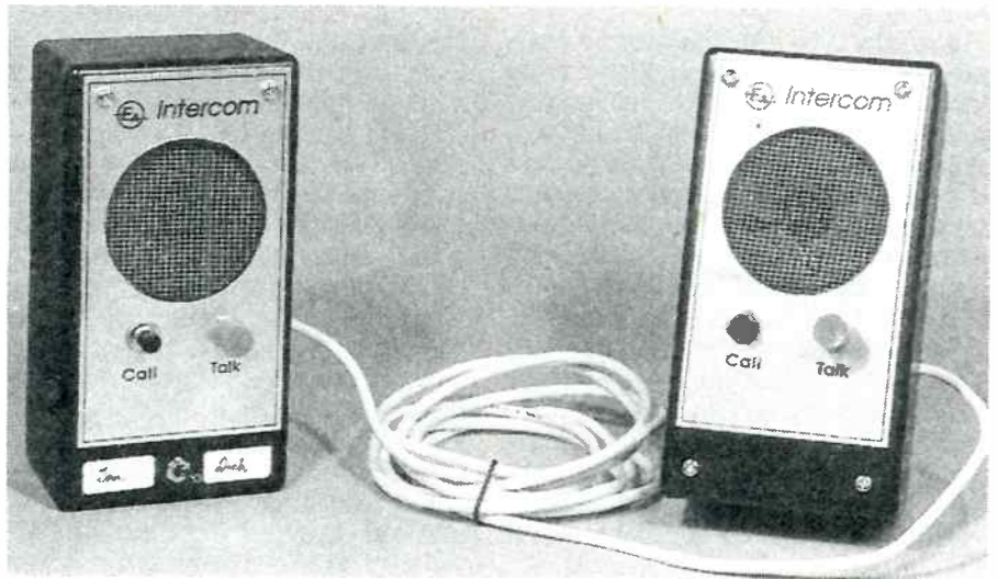
Shown are two variations of our intercom unit. The model on the left shows the optional privacy switch, and also the hole (lower left panel) to allow external adjustment of the amplifier gain.
