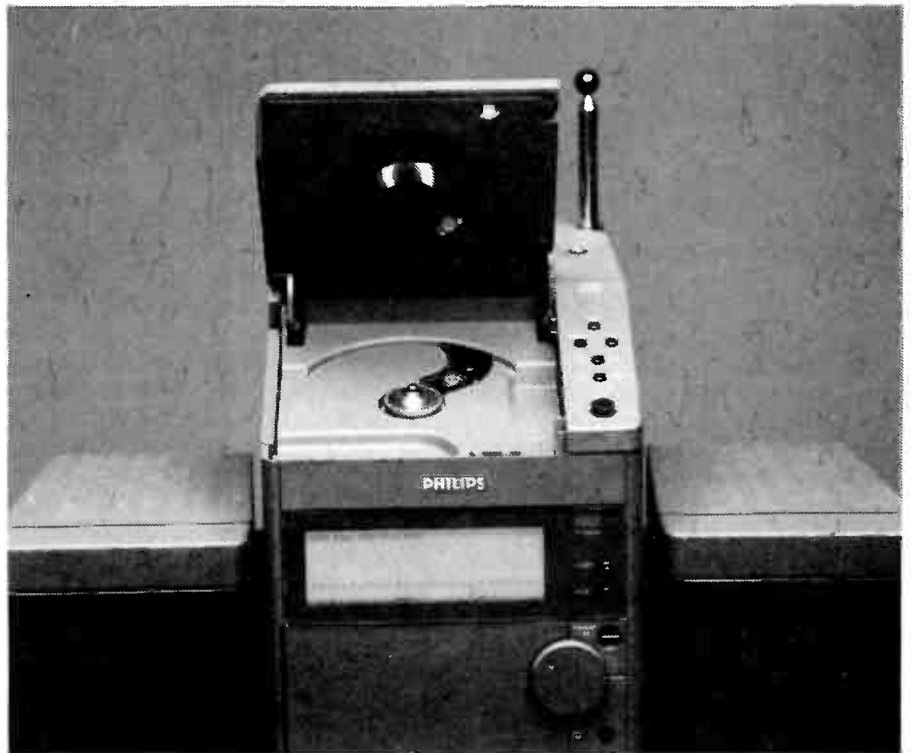
Unlike many other domestic CD players, this one has a swing up lid — revealing the laser optics. This makes it easier to clean the lens, but also makes it easier for dust to reach it — so that cleaning is likely to be needed more often!
