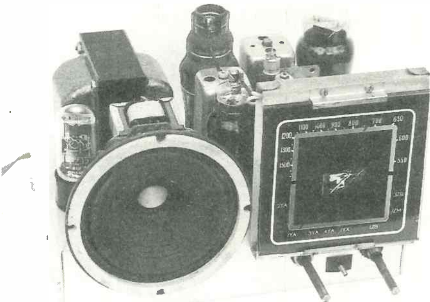
The completed chassis. A similar layout was used for all versions, with exact dimensions and orientation dependent on the size of the main components. 6G8-G and 6B8-G IF valves require shielding — this chassis uses a 'goat' type shield (centre rear), which John Moyle also used in the original.
