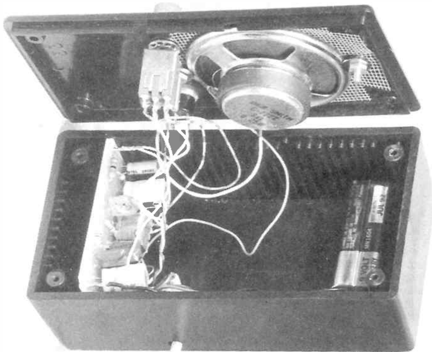
Looking inside the box shows the space at the right for the battery, and at the left for the privacy switch. The PCB slides into the slots on the sides of the zippy box.
