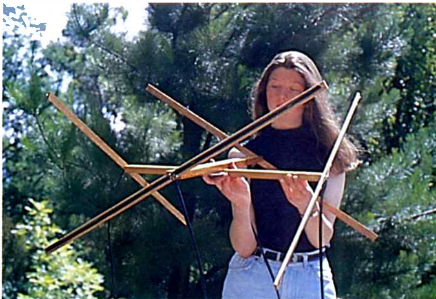
Photo 1: Tom's daughter Fiona is seen here holding the prototype of his Lindenblad antenna for the 137.4MHz weather satellite band. Note that each of the four elements slopes upwards to the right at 30 degrees, as viewed from the outside.
