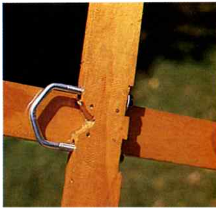
Photo 3: The lower wooden cross piece of the Lindenblad is fitted with a 'U' bolt as shown, for mast mounting.
