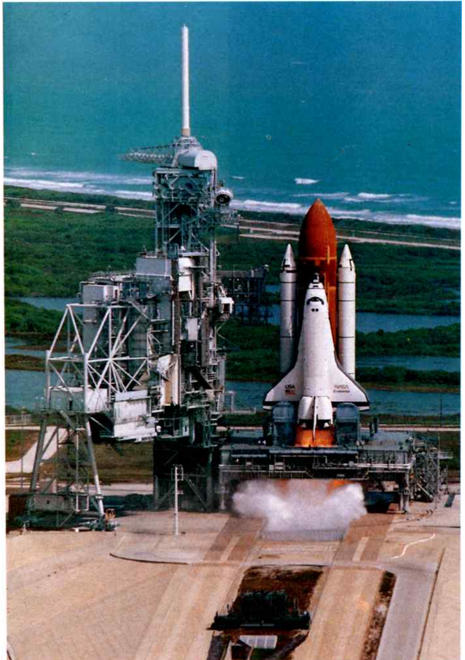
At Launch Pad 39B, the newest Space Shuttle 'Endeavour', undergoes a 22-second firing of its three main engines. A successful firing is required before launch on NASA's mission STS-49.
