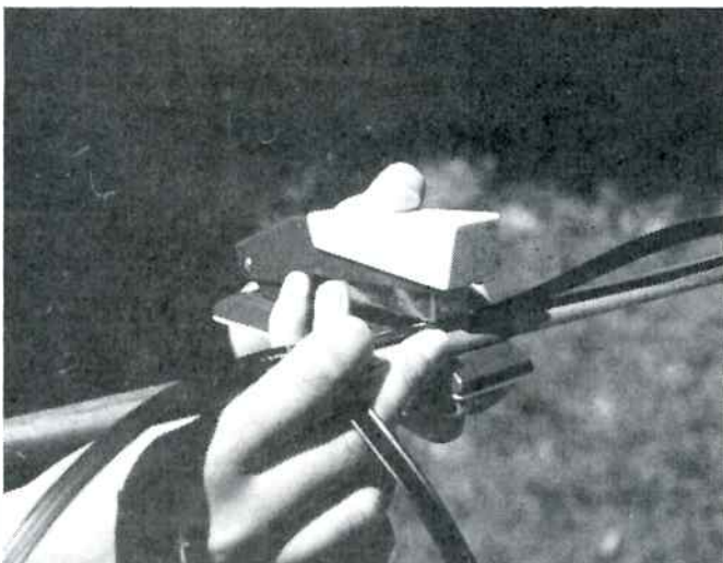
Photo 5: The 300 ohm ribbon used to make up the Lindenblad elements is attached to the wooden supports using the 'office' stapler, as shown here.
