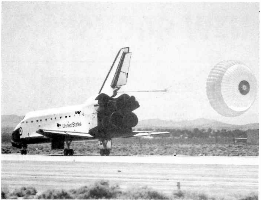
The main chute is fully deployed on Space Shuttle Endeavour's first landing, following a successful nine-day mission in Earth orbit. The landing was the first use of the Shuttle's drag chute system.
