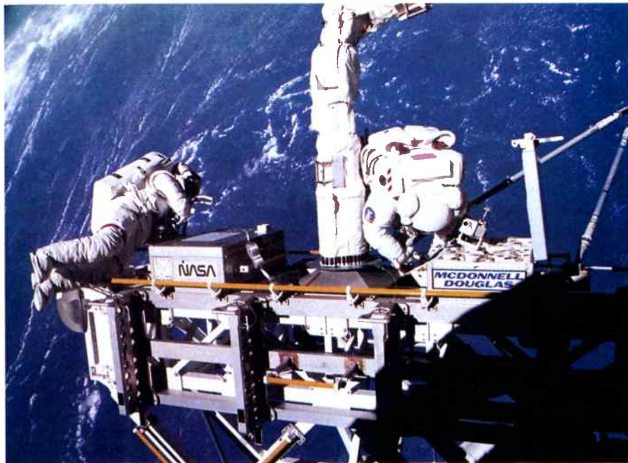
Here we see astronauts Kathryn Thornton (lef) and Thomas Akers at work with the components of the Assembly of Station by EVA Methods evaluation, the Ulti-purpose Support Structure (MPSS) is held aloft by Endeavour's remote manipulator system.
