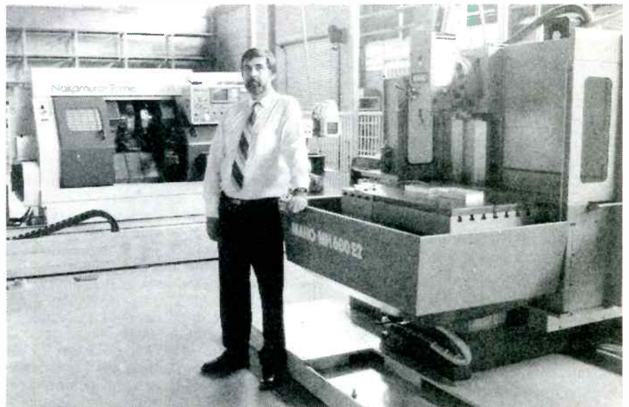
The NSW TAFE's new $7 million Automated Manufacturing Technology Centre at Lidcombe (western Sydney) boasts a number of large computer controlled machines, like those shown here with Centre Manager Gary Holborow. As it happens, the machines are mounted on special 'hovercraft' bases which allow them to be moved around effortlessly when required, on a cushion of air.
