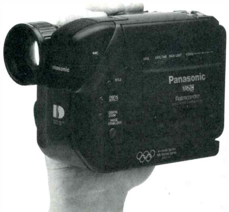
Panasonic's second image stabiliser camcorder, with an improved stabiliser system — the NV-S5A.
