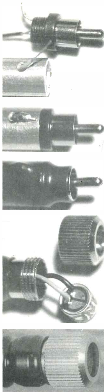
Photos 1 to 5: Stages in the assembly of the author's low cost 'calibrated' microphone, developed to go with his sweeper. Photo 1 shows the modified RCA plug; Photo 2 shows the fitted plug and earth wire solder joint; Photo 3 the same after fitting the heatshrink sleeve; Photo 4 the mic insert ready to be fitted into the Belling-Lee plug body; Photo 5 the assembled mic end.
