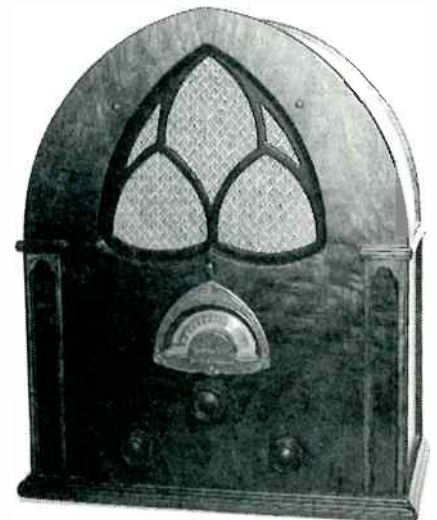
Left: The lacquer on this valuable 60-year-old Atwater Kent model 84 'Golden Voice' cabinet had deteriorated to the point where repolishing was the only remedy. Done professionally (above), this has really enhanced the set's value.
