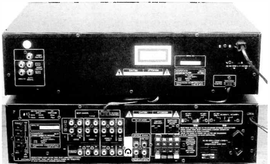
A rear view of the LVD-V7 laserdisc player (top) and the RX-V7 receiver, showing the connectors. Note that a special 'system control' cable is used to interconnect the two, so that the receiver can control some of the player functions.
