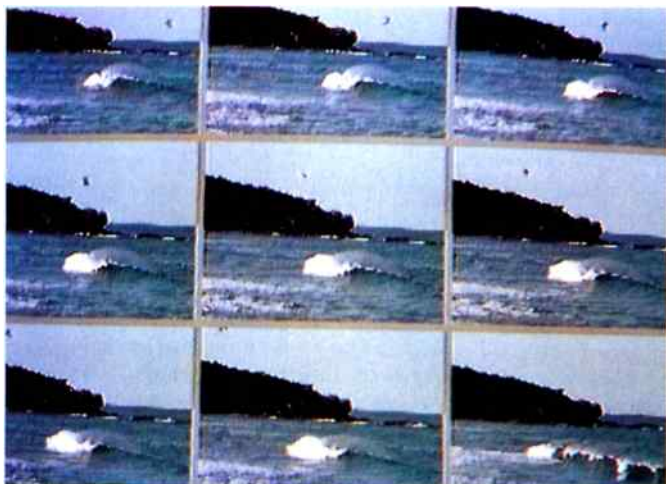
Multi mode — a nine-way split screen. Note the position of the seagull, indicating progressive capture of frame.
