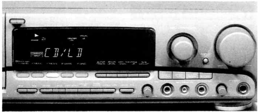
A close up of the centre and right-hand section of the front panel on the RX-V7 receiver. There are a relatively large number of control buttons, but many of these are only used occasionally.
