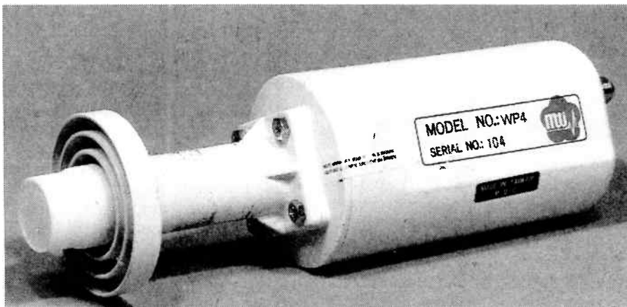
And here is the dual-polarity LNB, complete with its feed horn assembly.
