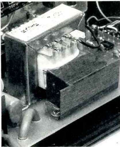
Three close-up shots inside the strobe, showing (a) the mains wiring insulating cover, and also the mains cable threaded in 'Loch Ness Monster' fashion through the PCB holes; (b) the completed converter transformer T2, mounted on the board; and (c) one of the flash tube support/connection loops, with the triggering electrode wire also visible.
