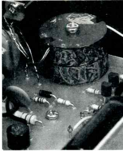
Three close-up shots inside the strobe, showing (a) the mains wiring insulating cover, and also the mains cable threaded in 'Loch Ness Monster' fashion through the PCB holes; (b) the completed converter transformer T2, mounted on the board; and (c) one of the flash tube support/connection loops, with the triggering electrode wire also visible.
