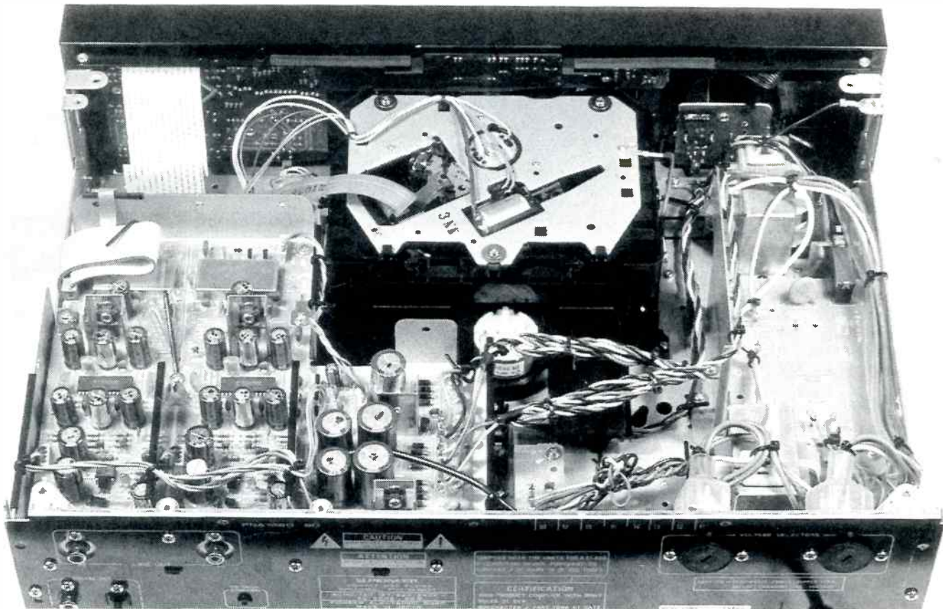
A general view inside the player. The mechanism in the centre looks rather unusual, because of its inverted nature compared with most other players. The PC board at lower left contains the separated D/A converters and analog output circuitry, with a great deal of shielding and careful layout evident.
