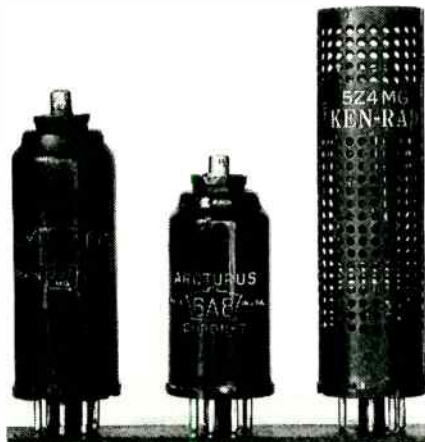
Fig.4: The 'metal glass' construction was the easy way out, for some makers faced with massive re-tooling costs. Hytron's 6Q7MG (left) used a tubular glass envelope with a metal shield; the Arcturus 'Coronet' series (6A8, centre) looked less traditional, but still had an internal glass envelope; while Ken-Rad (right) only progressed to metal valves in 1935, making the MG type until then.
