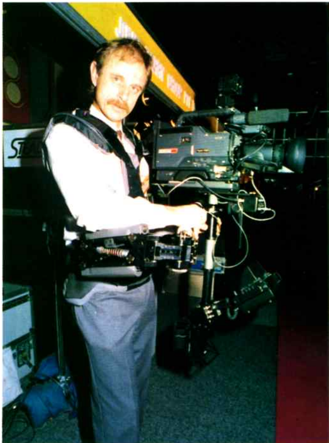
The John Barry Group was demonstrating this 'budget' Steadicam unit to support lightweight film and video cameras. It's priced at only $30,000!
