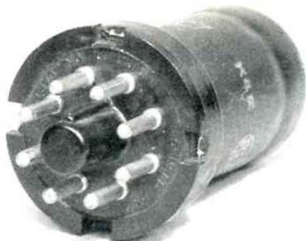
Fig.6: With the metal valves appeared the reliable octal base, which proved to be very successful and long-lived.
