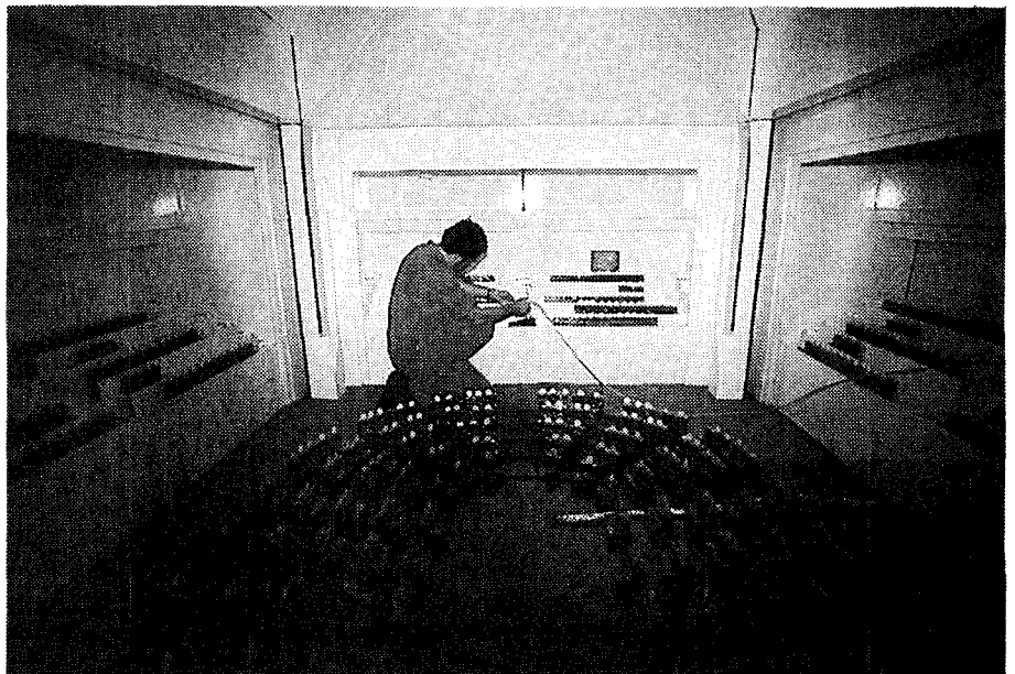
Danny Neuman, one of Louis Challis' associates, shown adjusting a microphone inside the 1/10th scale model for the Representatives Chamber of new Parliament House, during the acoustic modelling.
