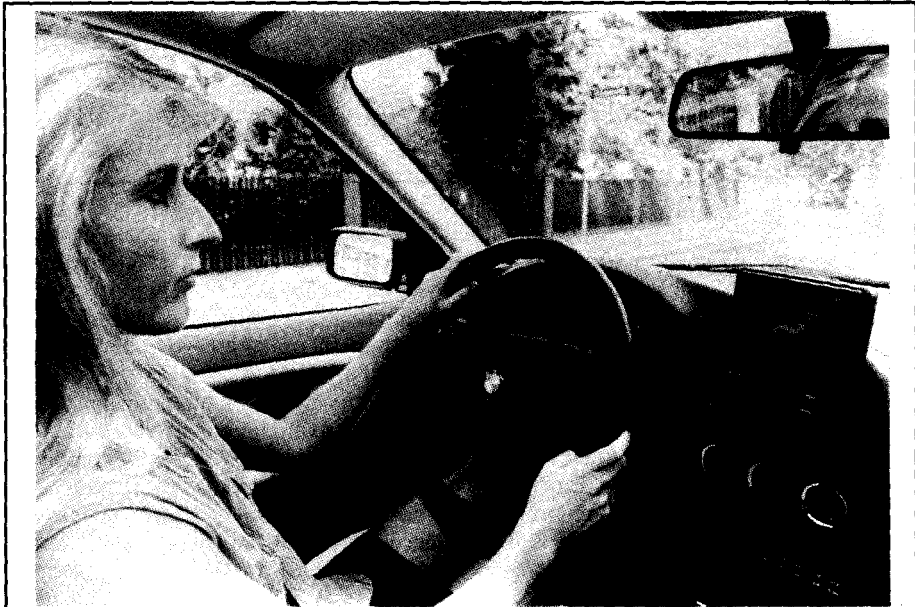
BMW's new 5-series cars feature a new Auto Scout car navigation system from Siemens. A console unit mounted on the dashboard (visible at right) pilots the driver via both on screen maps and acoustic clues. The required road maps and city plans are provided on diskette and are already available for many European countries and the USA.
