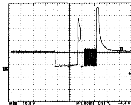
Fig.2: The injector current waveform. Following an initial 2ms pulse, a modulated current is to control AFR relevant to engine and load conditions.
