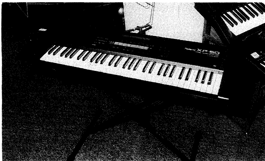
A Roland XP-50 keyboard/synthesiser, which Roland describes as a music workstation. Note the 3.5" floppy disk drive at the left hand end.
