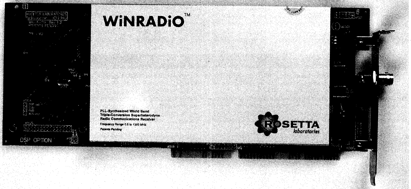
The hardware side of the WinRADIo package — a medium-length card which plugs into a standard AT-bus slot. As the inside of a PC is not the ideal environment for a communications receiver, all of the actual receiver circuitry is on a separate PCB and enclosed in a shielding box.
