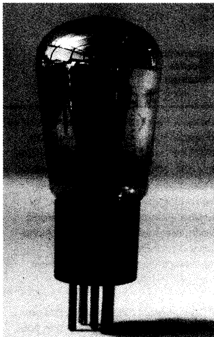
Germany's Telefunken were making indirectly heated valves very soon after America, but with 4V heaters. This REN1004 dates from 1928.
