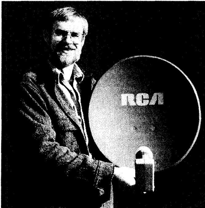
A technician holding one of the DSS receiving dishes made by RCA. Thanks to high power satellite transponders and the improved performance of digital transmission, they're particularly small and light.
