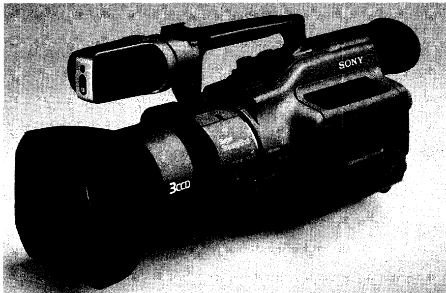
Sony's VX1000 camcorder, a three-CCD model using the Mini DV format. A digital output is provided, but as yet there's no means of accessing the signal.
