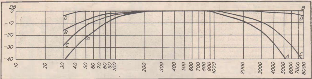
**SOME ILLUMINATING MEASUREMENTS.**—These curves of the performance of the Fidelity I.F. Super 5 show how the overall performance is affected by the design of the i.f. amplifier. Curve B shows the amplifier response and curve A the overall response when measured at the primary of the speaker transformer. Curve C (overall) and curve D (amplifier) result when the output is fed to a purely resistive load.
