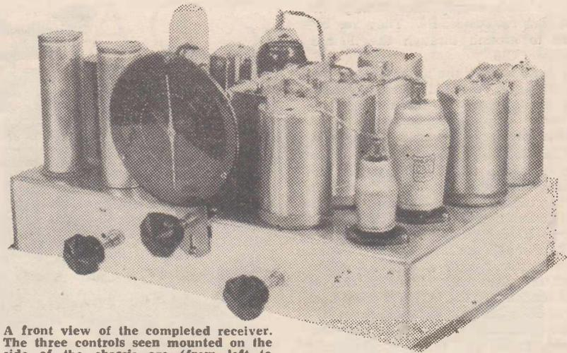
A front view of the completed receiver. The three controls seen mounted on the side of the chassis are (from left to right) the tone control, the main tuning control and the volume control.
