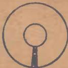
When the Eye appears, as illustrated, a strong signal is tuned correctly for maximum clarity.
