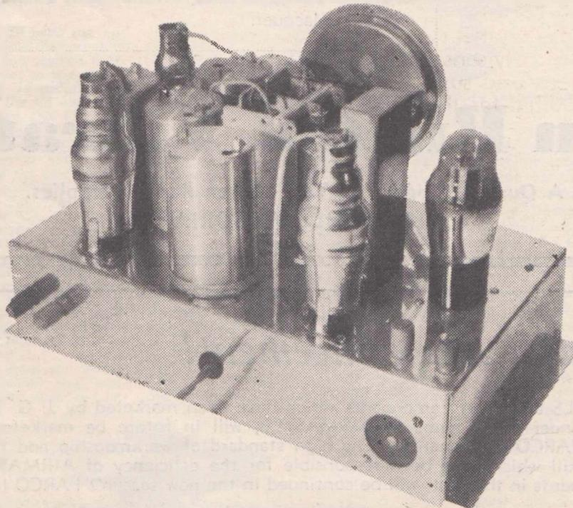
At the rear of the set can be seen the aerial and the earth terminals, the vibrator power input socket, and the two "A" battery leads arranged along the rear side of the chassis.
