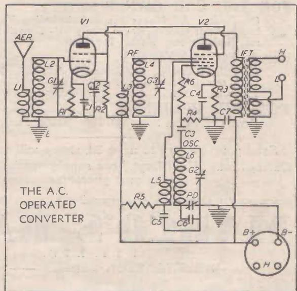
V2 and connect them to the filament lugs of the power input socket. All of this wiring must be carried out by means of twisted leads. Solder lugs should be placed under the bolts holding the coil shields, and these should be connected together with tinned wire and joined to the earth terminal.
