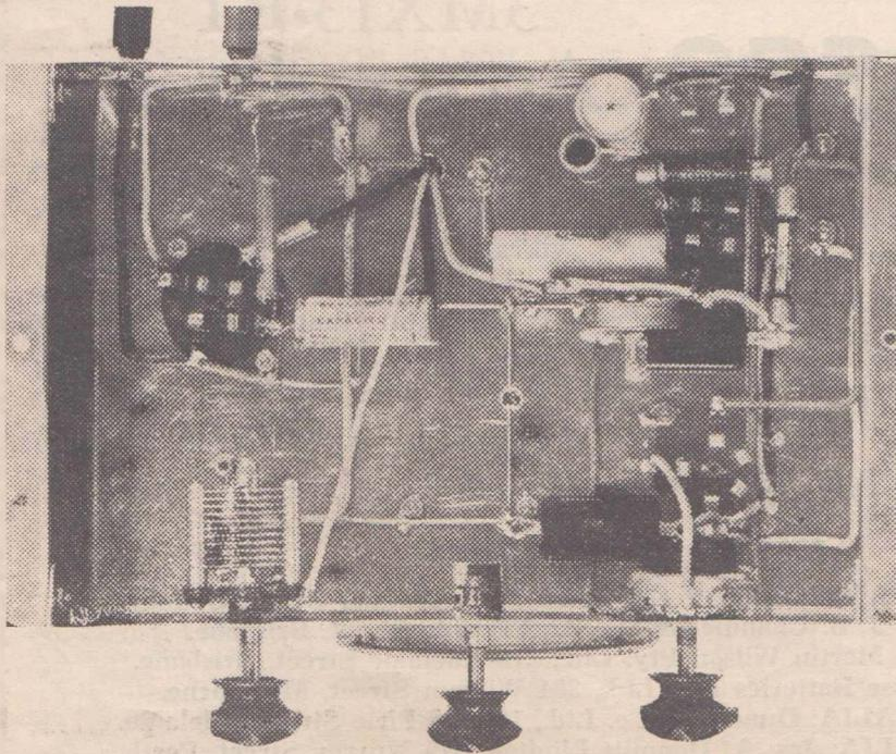
This illustration shows the placement and wiring of parts below the chassis. When wiring the receiver it is essential that all plate and grid leads be kept as short as possible.
