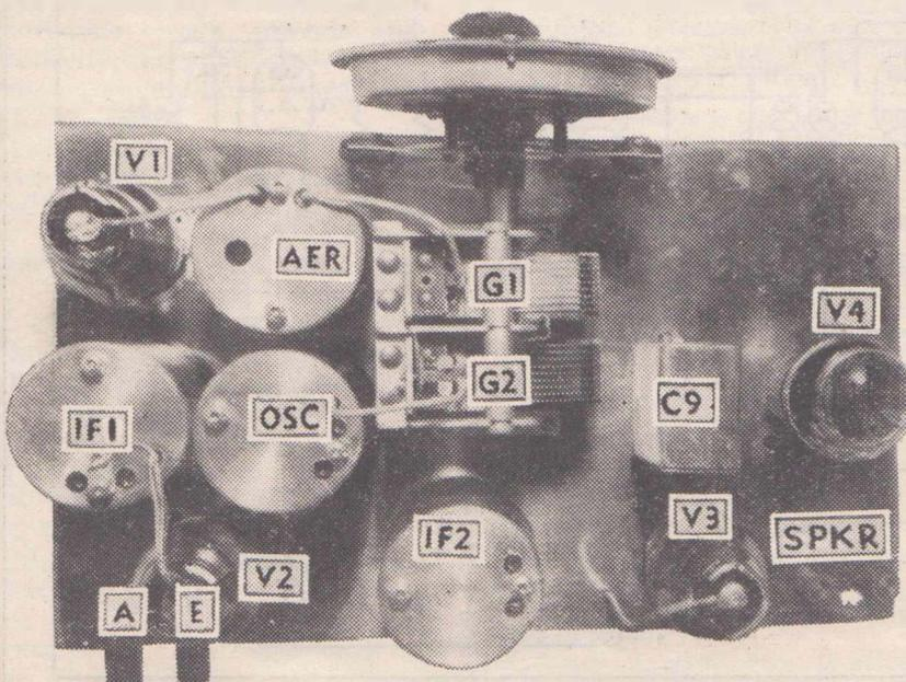
A keyed plan view of the receiver showing the arrangement of the component parts on top of the chassis.
