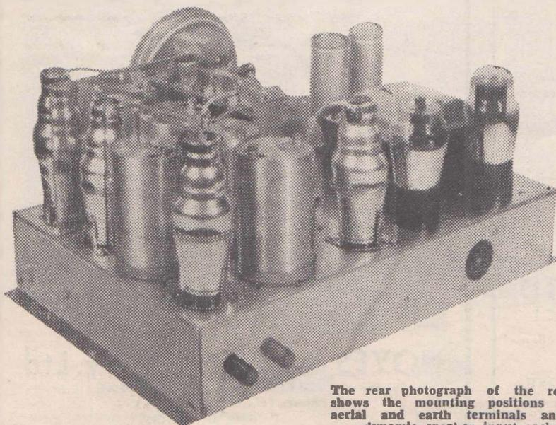
The rear photograph of the receiver shows the mounting positions of the aerial and earth terminals and the dynamic speaker input socket.
