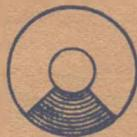
The "Magic Eye" as shown indicates that the signal the radio is reproducing is either from a weak station or is tuned incorrectly if reception is coming from a station nearby.
