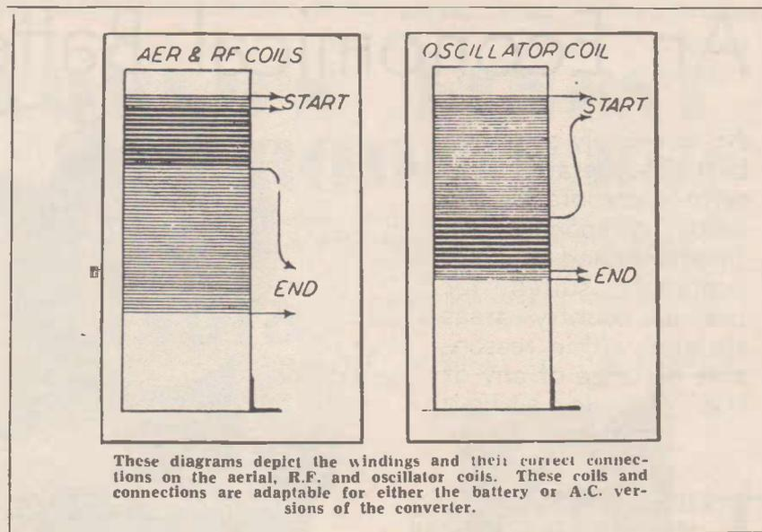
leaving the other one spaced by the diameter of the wire.
