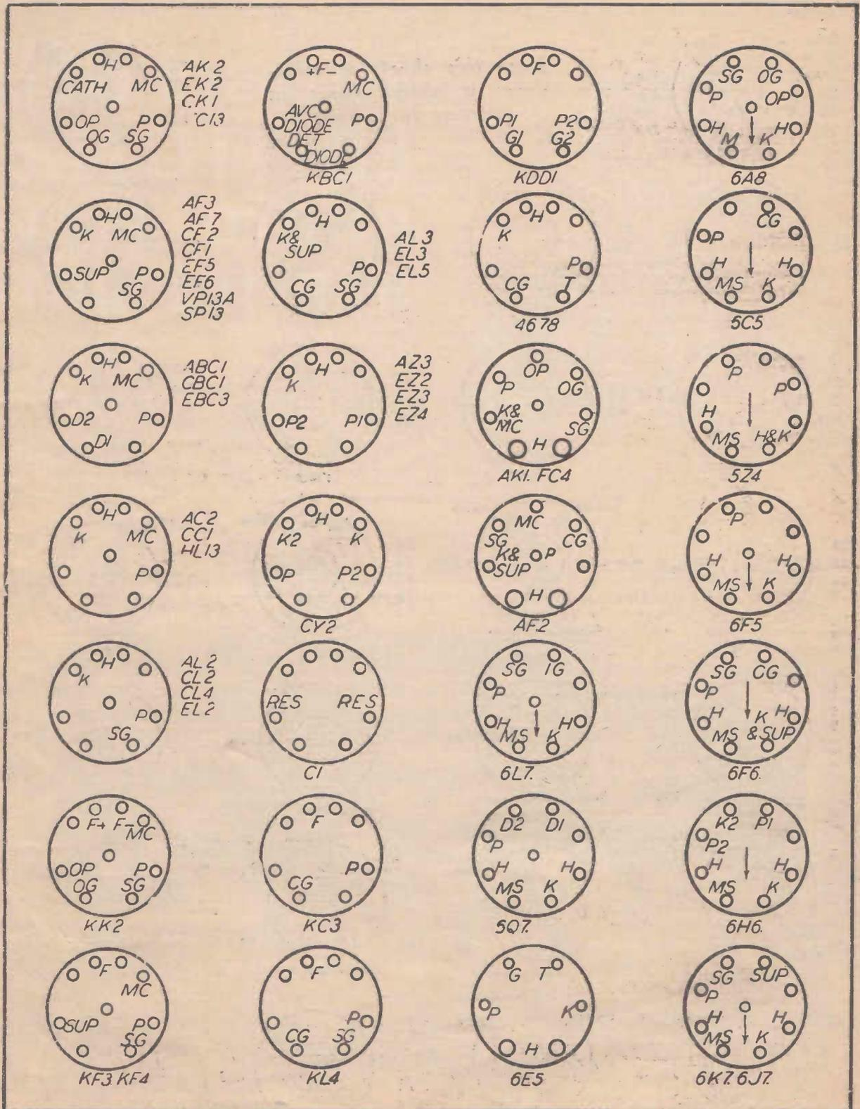
Note! Small unmarked circles in the centre of some socket diagrams indicate that the control grid connection is taken from the cap at the top of the valve.
