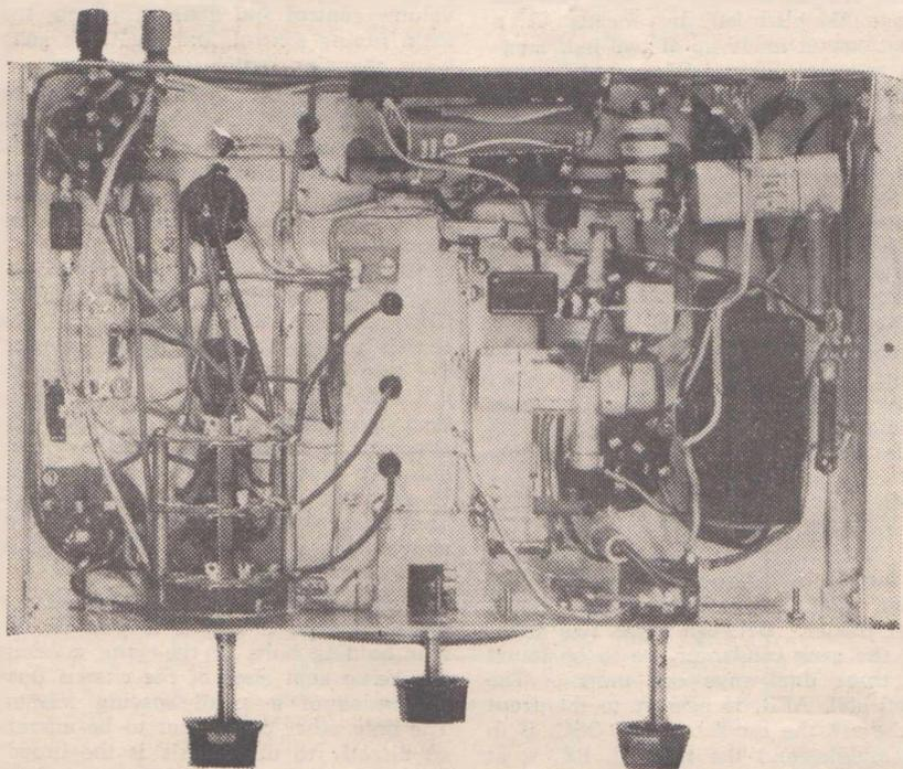
Another view of the receiver showing the placement and wiring of parts below the chassis. Care should be taken to ensure that all grid and plate leads are kept as short as possible in order to prevent tendency towards r.f. feed-back. This plan photograph of the receiver illustrates the arrangement of parts on top of the chassis. All components are key-lettered to correspond to the written description of the receiver.
