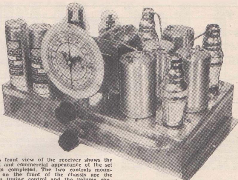
This front view of the receiver shows the neat and commercial appearance of the set when completed. The two controls mounted on the front of the chassis are the main tuning control and the volume control.
