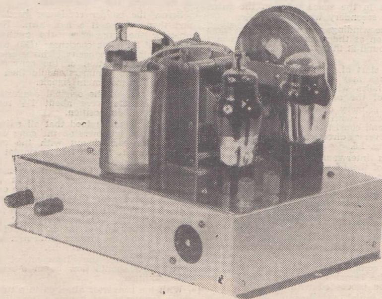
On the rear side of the chassis can be seen the battery input socket and the aerial and earth terminals.
