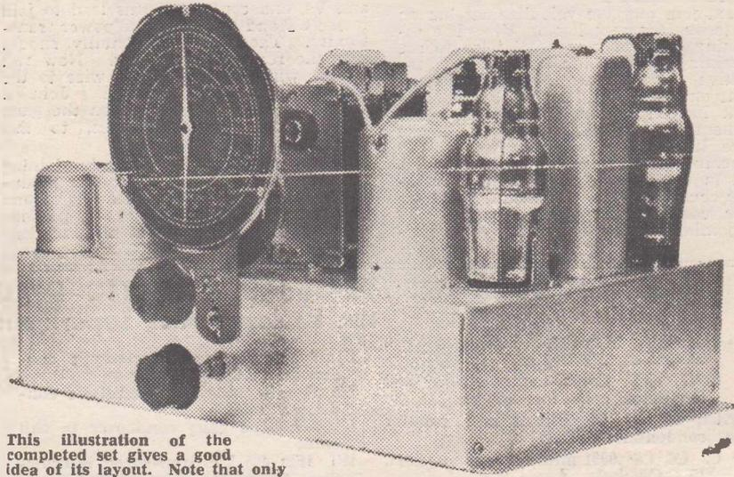
This illustration of the completed set gives a good idea of its layout. Note that only two controls—for tuning and volume are used.
