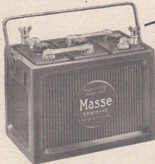
● Masse 3MX13-RT (capacity 120 ampere hours at the 100 hour rate) is an "A" type 6-volt accumulator with particularly heavy plates and double-thickness "Supercol" separators, deeply grooved for complete electrolyte activity. Its container is specially designed for inclusion in vibrator sets and is supplied with a quick fitting carrier handle.
