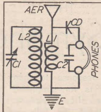
Circuit diagram of the trap-tuned crystal receiver.
