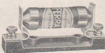
WIRE WOUND ANODE FEED RESISTANCES These Resistances are of the wire-wound type, the windings being sectionalised and supported on a moulded insulated bobbin within a bakelite tube with highly polished nickel-plated contact ends. 8/6 FROM . . . . .
