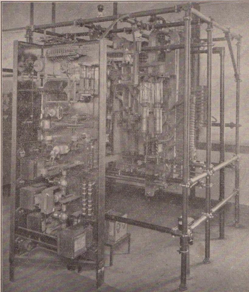
A view of the final stage of the Westinghouse Co's. 40 K.W. crystal controlled S. W. station W8KK.
