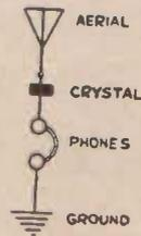
Fig. 27 shows the supposititious connection of headphones in a radio circuit.
