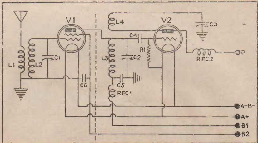
Fig. 1.—The schematic diagram which shows the circuit arrangements of the d.c. short wave adaptor.
