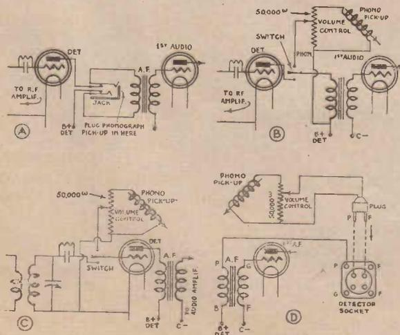
Fig. 2.—The schematic diagram showing various methods of pick-up connections.
