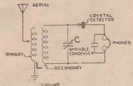
Fig. 34.—An even more selective arrangement, which is known as a "loosely coupled" circuit.
