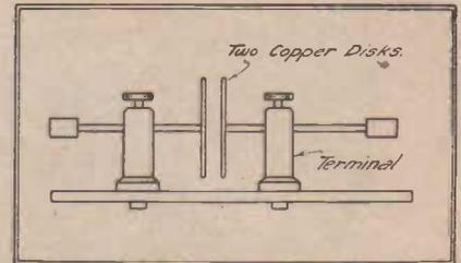
Details of the aerial coupling condenser used in the receiver are provided by this drawing.
