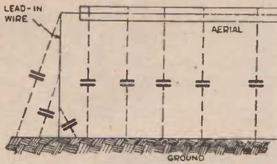
Fig. 25. The condenser effect existing between aerial and earth.
