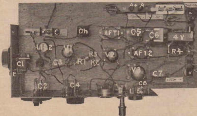
The baseboard view of the receiver, key-lettered to agree with other technical dope which has been provided. Note the unusually wide spacing of parts, which is such a feature of the set's construction.
