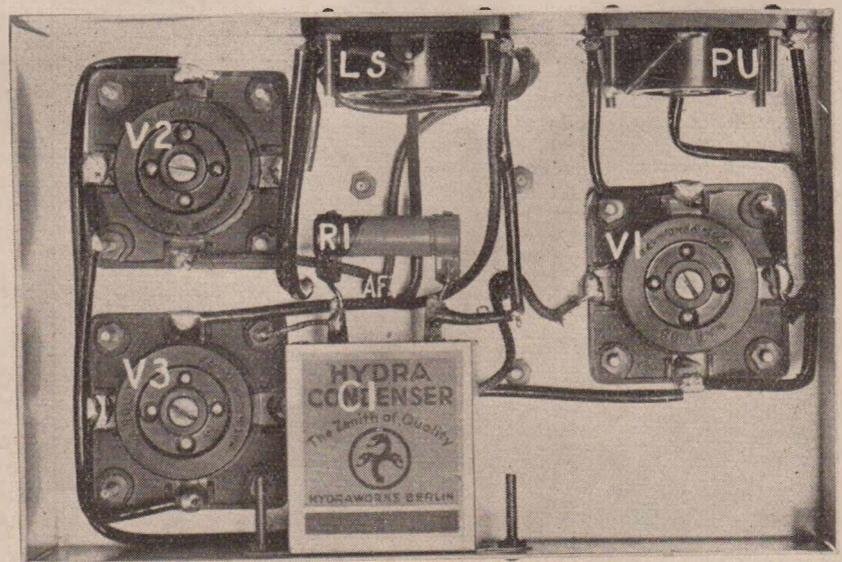
An under-chassis view of the amplifier, showing the components key-lettered to agree with the schematic diagram, the list of parts, and the wiring description.
