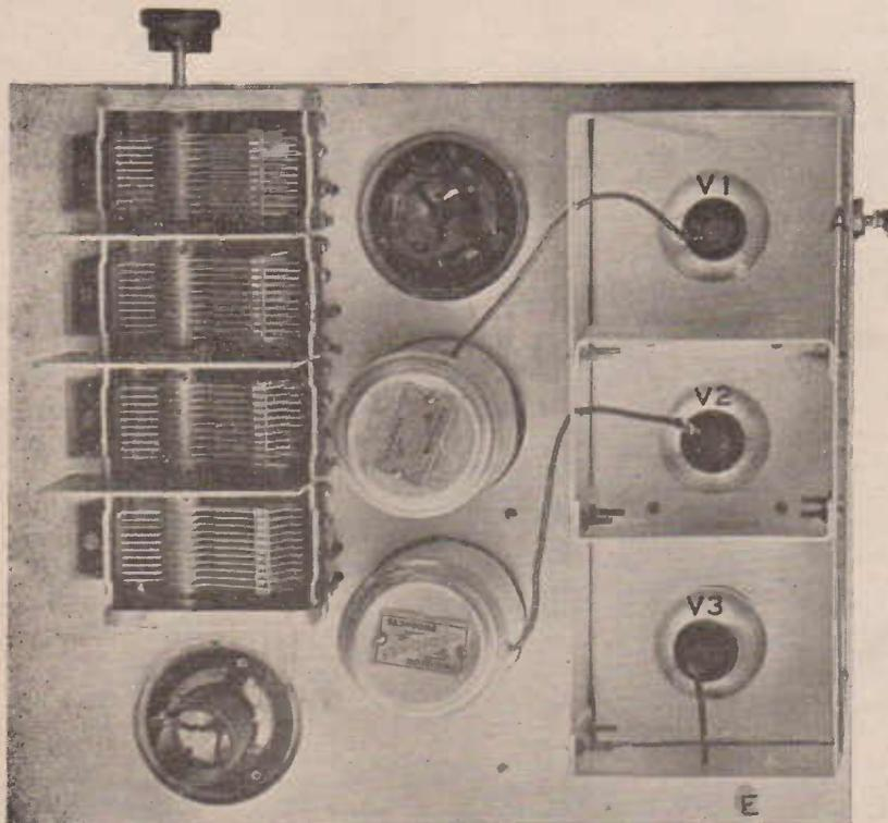
A view of a section of the receiver, showing the r.f. valves mounted in their screening boxes, and showing also two of the r.f. coils with their screens removed.
