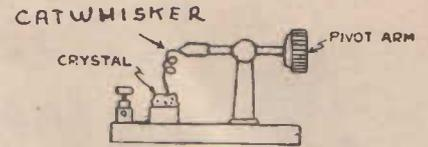
A diagrammatic view of a crystal detector. Fig. 29.
