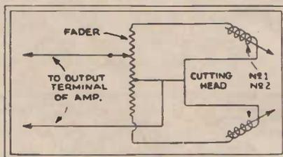
A fader system commonly used for mixing two cutting heads.
