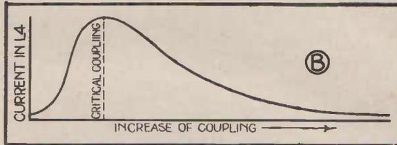
Fig. 102.B. The graph showing the relation between increase in coupling and current.
