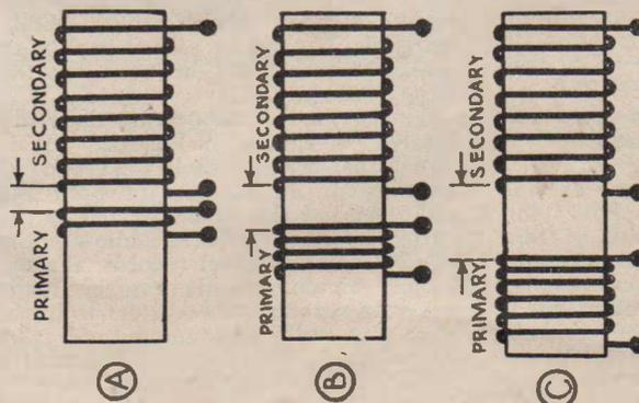
Fig. 104. Three forms of primary and secondary coupling are illustrated here.
