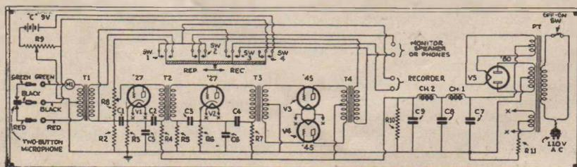
Fig. 72. Schematic circuit of the equipment with amplifier of the Portable Sound Recorder. The filtering of the power supply shown is very important.
