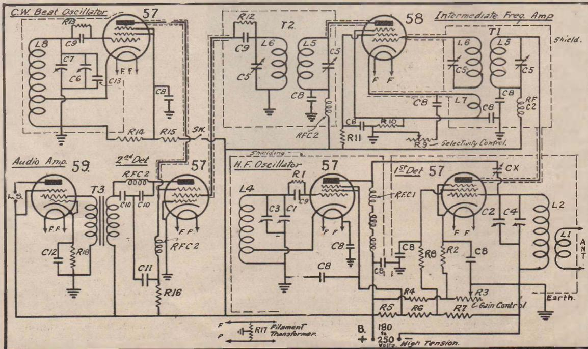
Schematic Diagram, showing the various stages in their relative positions on the chassis. Dotted lines indicate shielding. The common side of C10 and C11 must be earthed. This is not shown above.
