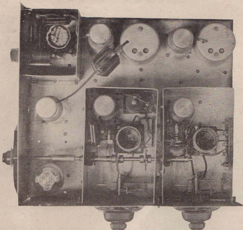
Looking Down on the Completed Receiver. Note How the Tuning Condensers are Ganged!
