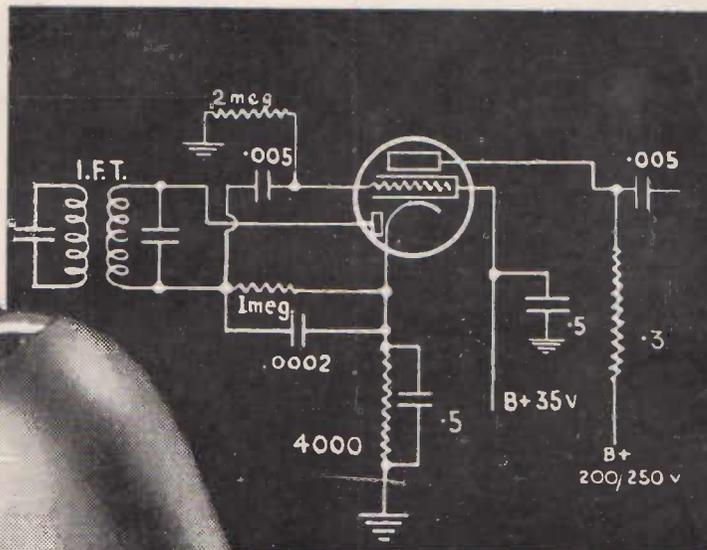
*A typical circuit arrangement incorporating the E444 Diode Screen Grid as a combined second detector and first audio stage in a conventional superheterodyne.*
