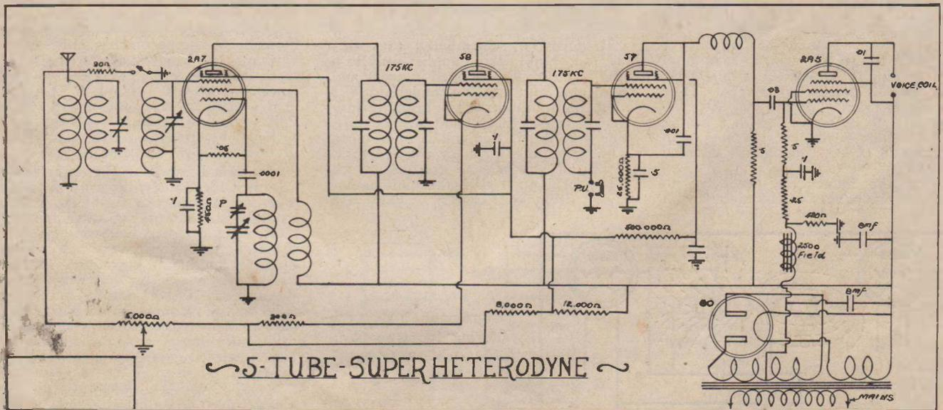
Schematic diagram of the Saxon Five, giving full circuit details.
