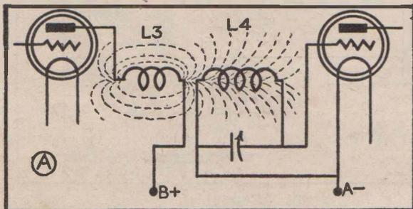
Fig. 102.A. Diagrammatic sketch showing loose coupling between L<sub>3</sub> and L<sub>4</sub>.
