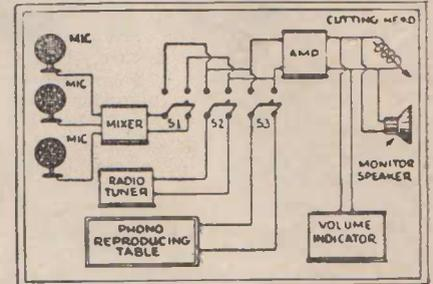
Fig. 62 Switching arrangement for connecting either alone, or in any combination the microphones, radio or phonograph to the recording amplifier.
