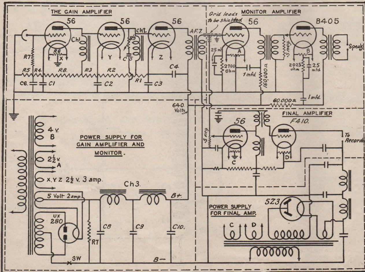
Schematic Diagram, showing the Three Units and Power Supply coupled together.
